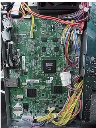
When the connection part of the connector is lifted up as shown in the figure, the connector is unlocked. It is necessary to remove the FFC with releasing the lock of the connector.
