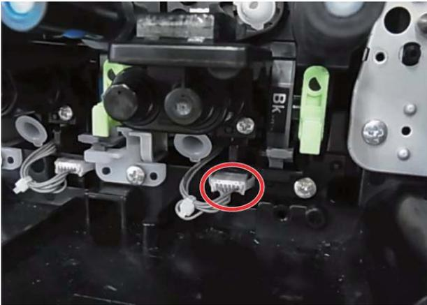
5) Pull out the developing unit with pressing the lever.
