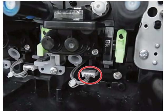
(Note1) Clean the developing material when the developing material is on the DV side label as shown in the figure. (F/R both side)
