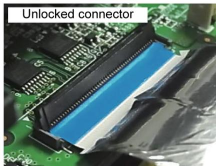
It is necessary to remove the FFC after the FFC is lifted up , pulled out obliquely upward and the tab is removed from the connection part. If the FFC is forced to remove, the FFC and the connector could be broken.
