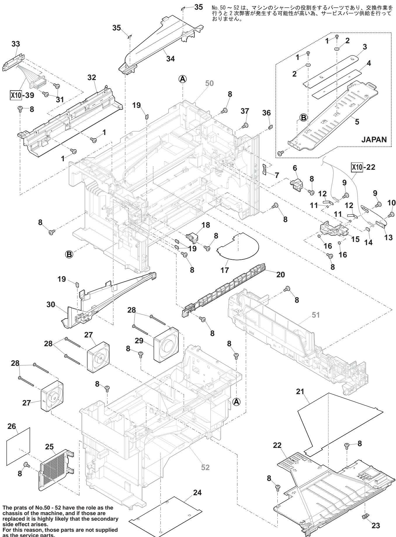
The parts of No.50 - 52 have the role as the chassis of the machine, and if those are replaced it is highly likely that the secondary side effect arises.
