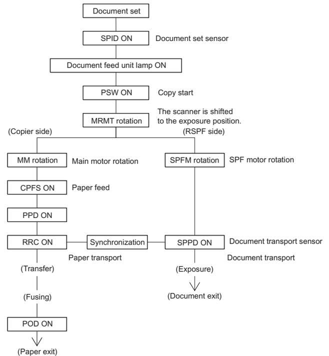
In the zooming mode, the magnification ratio in the sub scanning direction (paper transport direction) is adjusted by changing the document transport speed.
