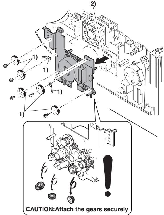
17) Remove the parts as shown below, and remove the pressure release solenoid and the paper feed solenoid.
