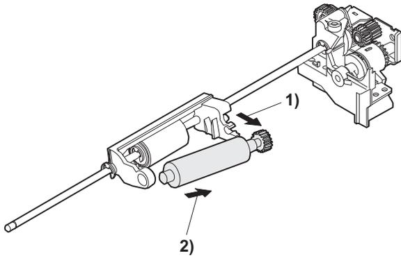
7) Cut the binding band and remove the multi paper feed solenoid.
