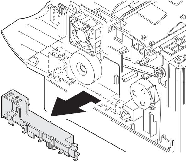
14) Remove two screws and remove the toner motor.
