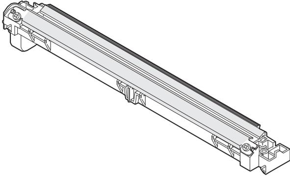
3) Insert the charger cleaner into the transfer unit, and move it a few times in the direction of the arrow shown in the figure below.
