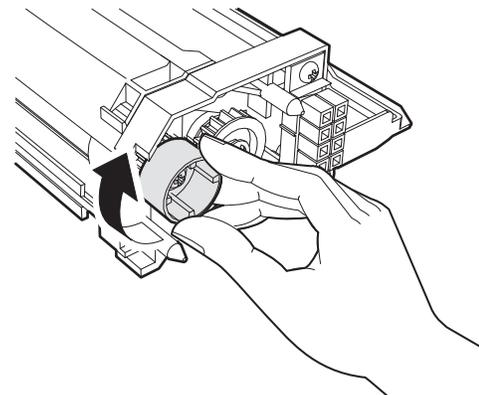
Note: Never rotate the gear in the reverse direction.
