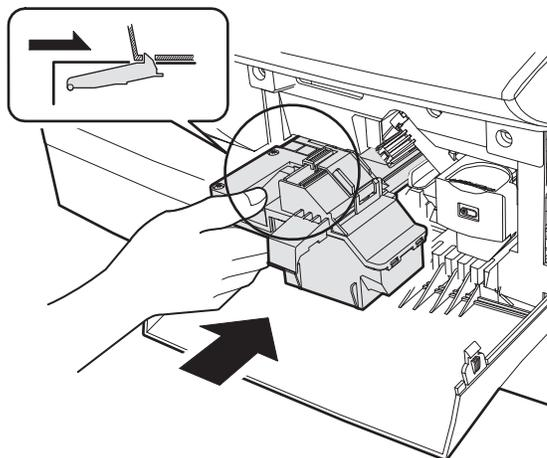
6) Pull out the shutter in the arrow direction.
