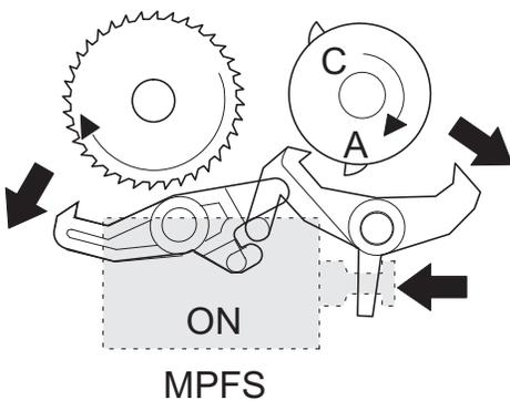
4) The lead edge of the transported paper is pressed on the resist roller by the transport roller. Then the paper is stopped temporarily to allow synchronization with the lead edge of the image on the OPC drum. From this point, the operation is the same as the paper feed operation from the tray. (Refer to 7-5 - 8.)
