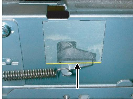
Align the edge of the mylar to the R part (the yellow line in the diagram below) so that the hole of the metal plate is covered as much as possible.
