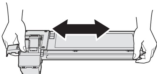
2) Hold the section of Toner unit shown in the figure below, remove the packing tape, and remove the cushion.
