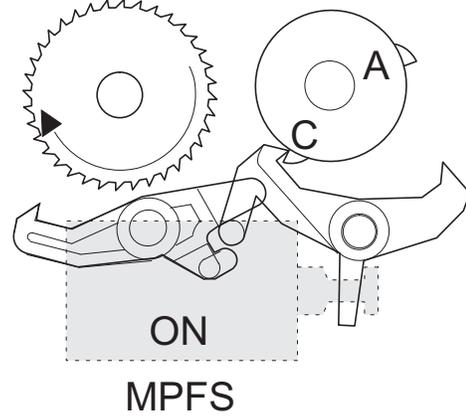
2) When the Start key is pressed, the manual paper feed solenoid (MPFS) turns on to disengage the manual paper feed latch. A from the manual paper feed clutch sleeve A, rotating the manual paper feed roller and the manual take-up roller. At the same time, the manual paper feed stopper opens and the manual take-up roller is pressed to the surface of the paper to start paper feeding.
