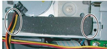
Press the cushion with a sharp-pointed stick or something to fill the gap between the mylar and the metal plate.
