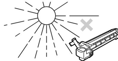
Store spare supplies such as drum cartridges and toner cartridges in a dark place without removing from the package before use. ▲
