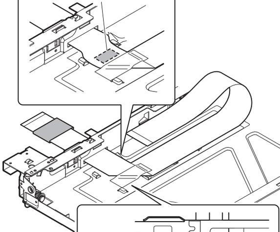
Note: Attach the FCC to fit with the marking line. Marking line.
