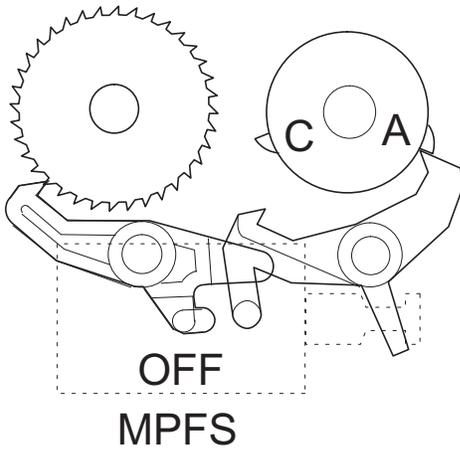
3) When pawl C of the manual paper feed clutch sleeve is engaged with the manual feed latch, the manual feed stopper falls and the manual take-up roller rises. At that time, the manual paper feed roller is rotating.
