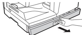
2) Remove the pressure plate lock. Rotate the pressure plate lock in the direction of the arrow to remove it while pressing down the pressure plate of the paper tray.
