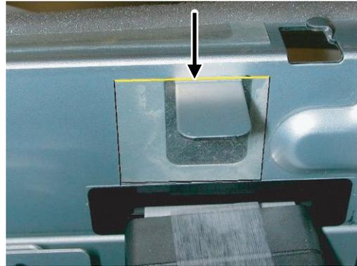
Attach along the edge of the projection (the yellow line in the diagram below).
