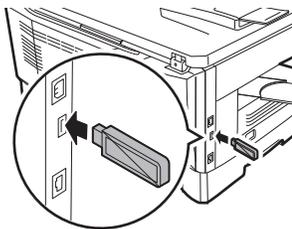
When the USB memory is inserted into the memory, upgrading is automatically performed.
