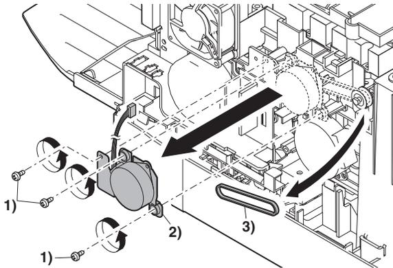
16) Remove five screws and the grounding wire, and remove the main drive unit.
