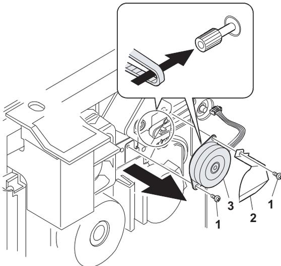
Note: When reassembling, be sure to engage the Duplex motor gear with the belt on the main body side.
