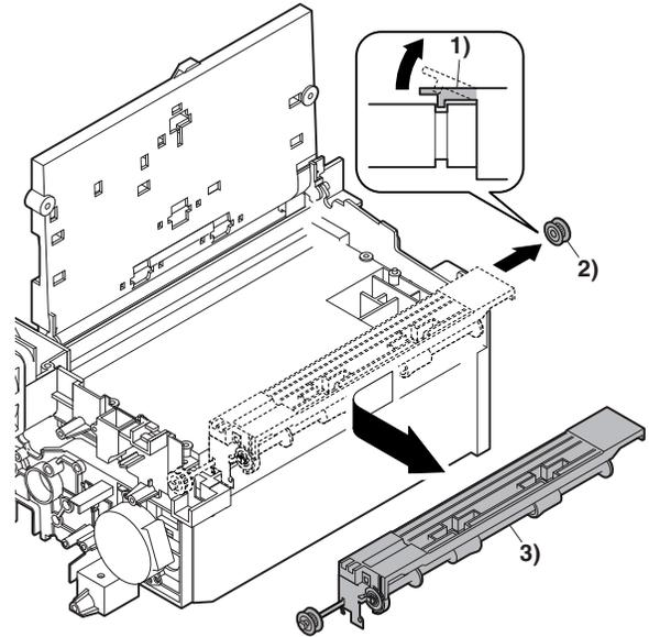
22) Disengage the pawl, and remove the pulley.
