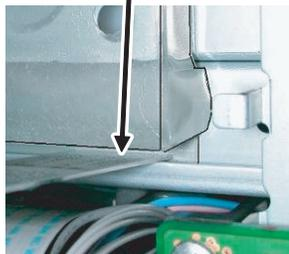
Press the mylar with a sharp-pointed stick or something so that it is stuck correctly.
