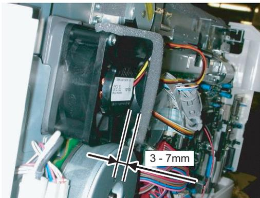
Attach the cushion leaving 3 - 7mm from the edge so that the gap between the Fan housing cushion and the filter of the rear cabinet is filled for sure.
