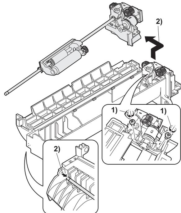
5) Remove three E-rings and remove the manual paper feed roller B9.
