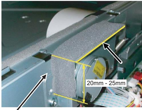
Press and attach the cushion aligning it to the metal plate so that there will be no gap between them.
