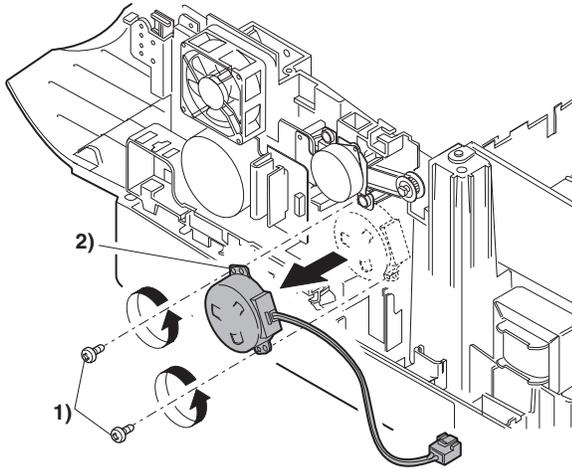
15) Remove three screws, and remove the DUP motor unit and the belt.
