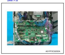
2. Remove all connectors on the FS control board.
