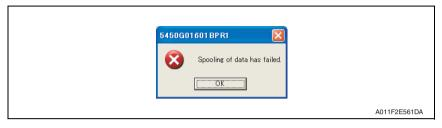
Check that the printer is ready and that it is correctly connected, and then click the [Update again].
