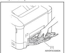
2. Press down the media lifting metal plate [1].
