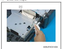
Wipe the tray3 media feed roller [1] clean of dirt using a cleaning pad dampened with alcohol.
