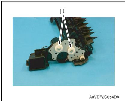
15. Remove two gears assy [1].
