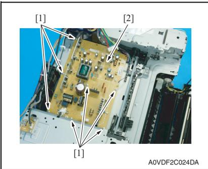
13. Remove seven screws [1], and remove the DC power supply [2].
