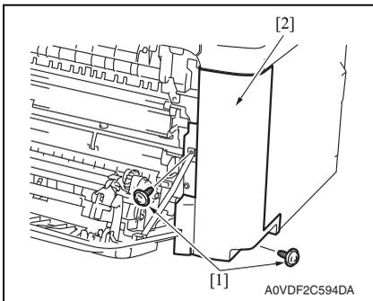
2. Remove two screws [1], and remove the rear right cover [2].
