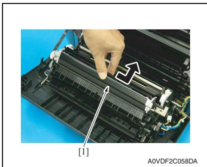
2. Remove the 2nd transfer roller unit assy [1].
