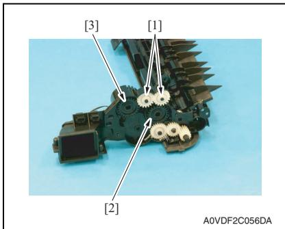
17. Remove two gears [1] and remove the switchback roller feed clutch [2] or the switchback roller reverse clutch [3].
