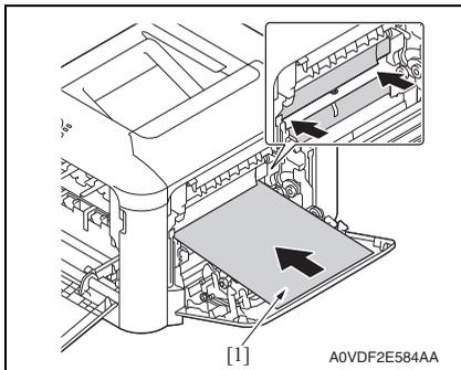
5. Insert the protective sheet [1] into the unit in the direction of the arrow until it stops.
