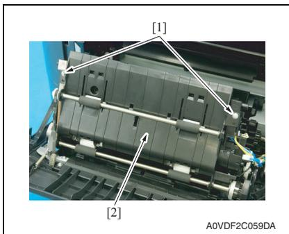
3. Remove two screws [1], and remove the duplex conveyance roller assy [2].
