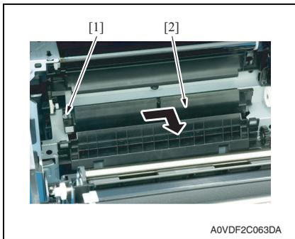
7. Remove the screw [1] and remove the sensor holder [2] as shown in the illustration on the left.
