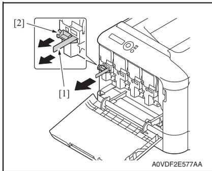
8. Make sure that the toner cartridge is securely installed, and then remove the protective film [1] and the bracket [2].
