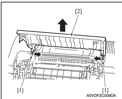
2. Unlock two tabs [1], and remove the exit cover [2].
