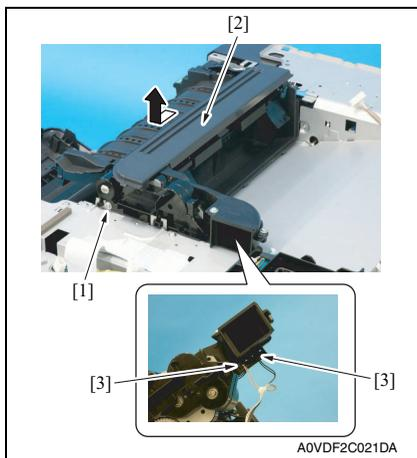
10. Remove the screw [1], and remove the exit drive assy [2].
