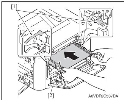
9. Insert the transfer belt unit [2] along the rail [1].
