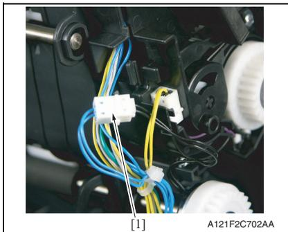
3. Connect the duplex conveyance roller clutch connector [1].
