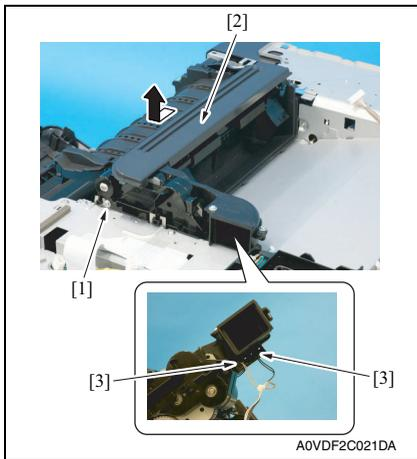
11. Remove the screw [1], and remove the exit drive assy [2].
