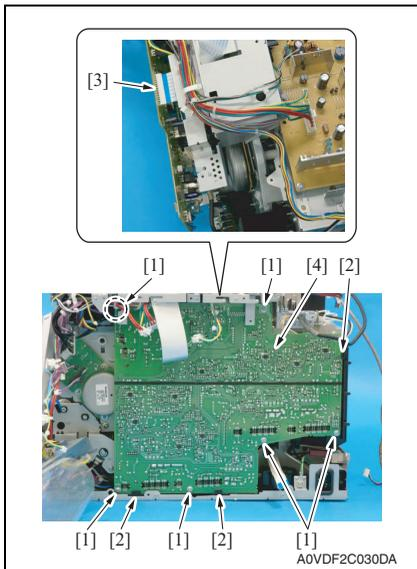
23. Remove six screws [1] and three tabs [2].
