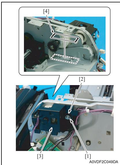
4. Remove the E-ring [1] and bushing [2], and remove the holder [3].
