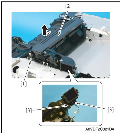
8. Remove the screw [1], and remove the exit drive assy [2].
