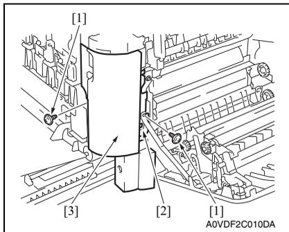
5. Remove two screws [1] and unlock the tab [2], and remove the front right cover [3].
