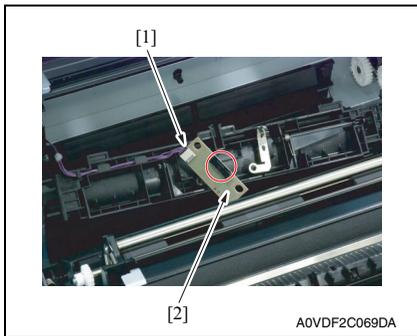
8. Disconnect the connector [1], and remove the IDC sensor [2].
