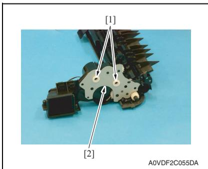
16. Remove two bushings [1], and remove the metal plate [2].
