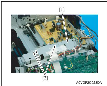
21. Remove three screws [2] of the metal plate [1].
