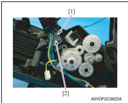
6. Remove the screw [1], and remove the 2nd transfer release solenoid [2].
