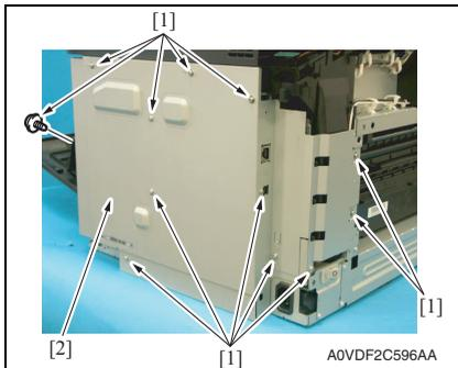
3. Remove twelve screws [1], and remove the board protective shield [2].
