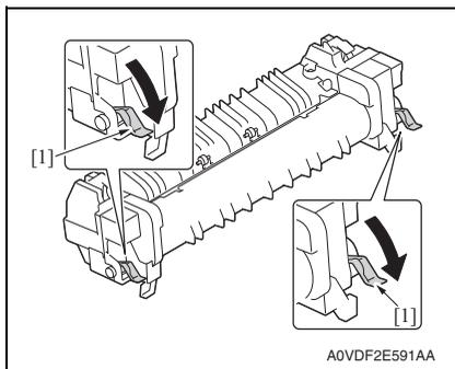
8. Pull down two levers [1] of a new fuser unit.
