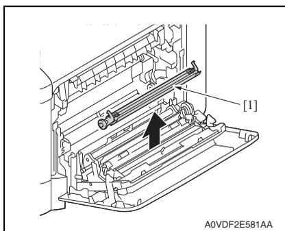
4. While continuing to press the levers, remove the transfer roller [1].
