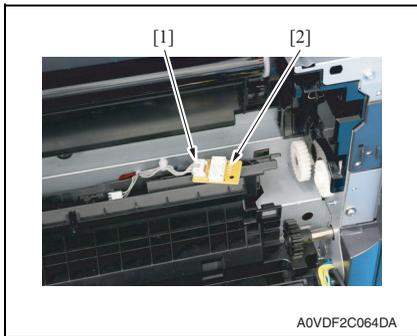
8. Disconnect the connector [1], and remove the temperature/humidity sensor [2].
