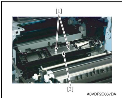
6. Remove two screws [1], and remove the sensor cover [2].
