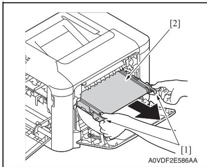
7. Hold the handles [1], and then carefully pull out the transfer belt unit [2].
