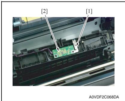
7. While slightly raising the ground plate [1], remove the IDC sensor [2].
