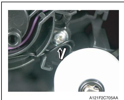
6. Using tweezers or similar tool, tidy up the harness on the duplex conveyance roller clutch side by pushing it in the direction of the arrow.
