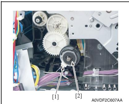
5. Disconnect the connector [1], and remove the tray2 media feed clutch [2].
