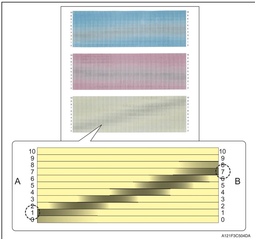
4. Make adjustments so that the gray area on each color sample of the output test pattern becomes parallel to the main scan direction.
