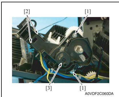
4. Remove two screws [1] and unlock two tabs [2], and remove the holder [3].
