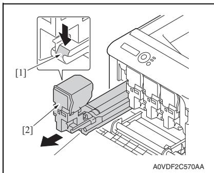
4. While pressing down the area marked "Push" [1] on the toner cartridge to be replaced, slide the cartridge [2] completely out of the printer.
