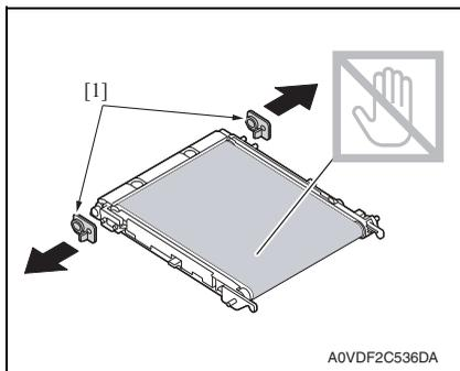
8. Remove the protective cover [1] from the new transfer belt.
