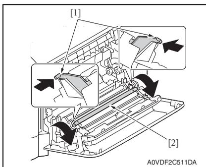
2. Push two levers [1] inside to unlock the transfer roller.
