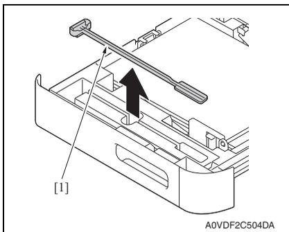
3. Remove the laser lens cleaning tool [1].
