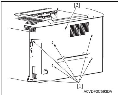
3. Remove six screws [1], and remove the left cover [2].
