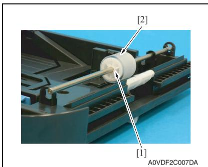
4. Remove the C-ring [1], and remove the tray2 feed roller [2].
