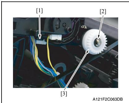
8. Remove the hookup connector from the holder and pull out the connector [1].
