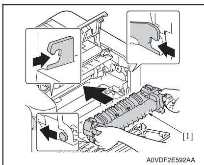
9. Insert the fuser unit [1] until it locks into place.
