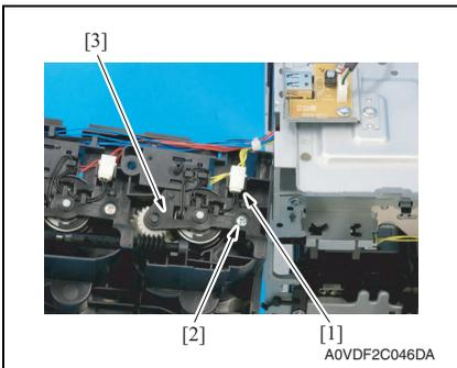
15. Remove the harness from guide, and disconnect the connector [1].
