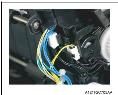
4. Fix the hookup connector of the duplex conveyance roller clutch to the holder of the conveyance unit.
