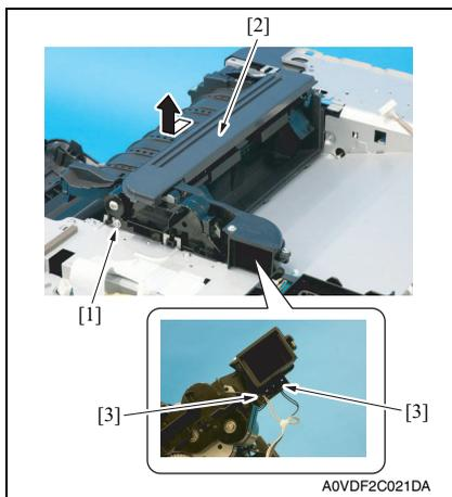
8. Remove the screws [1], and remove the exit drive assy [2].
