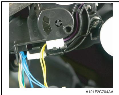
5. Route the harness of the duplex conveyance roller clutch as illustrated on the left.
