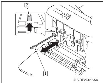
9. Insert the laser lens cleaning tool [1] into the laser aperture [2], pull it out, and then repeat this back and forth movement 2 or 3 times.
