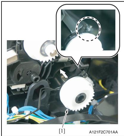
2. Install the duplex conveyance roller clutch [1] and fix it with the E-ring.
