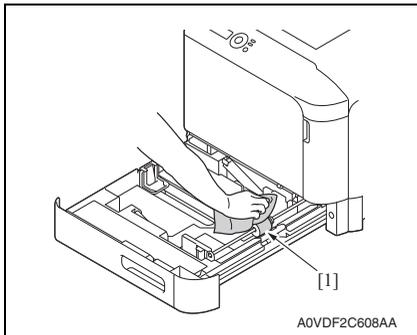
2. Using a cleaning pad dampened with alcohol, wipe the tray2 feed roller [1] clean of dirt.
