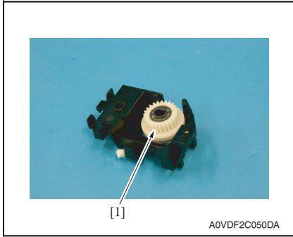
5. Remove the loop detection clutch [1].
