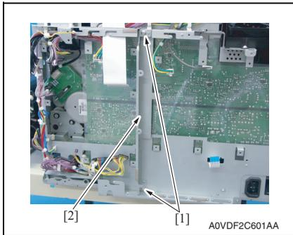
14. Remove two screws [1], and remove the mounting metal plate [2].
