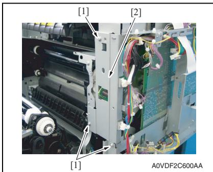
13. Remove three screws [1], and remove the metal plate [2].
