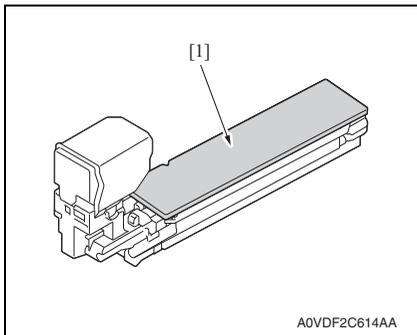
8. Attach the cover [1] to the removed toner cartridge.
