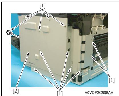
5. Remove twelve screws [1], and remove the board protective shield [2].
