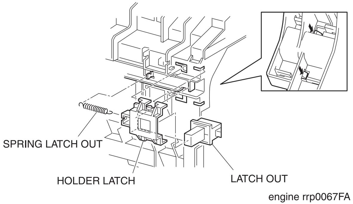
Figure: LATCH OUT Removal
