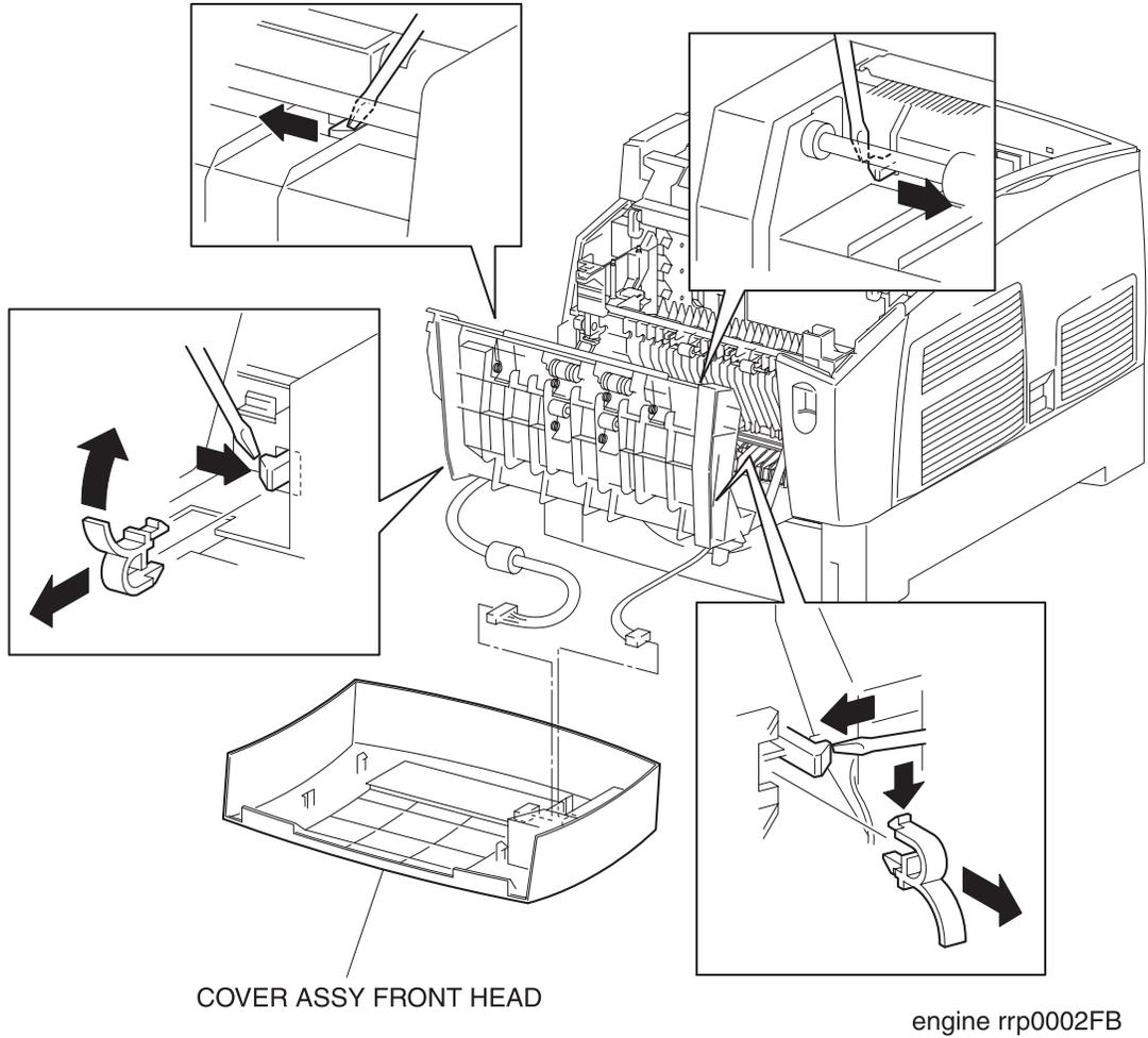
Figure: COVER ASSY FRONT HEAD Removal
