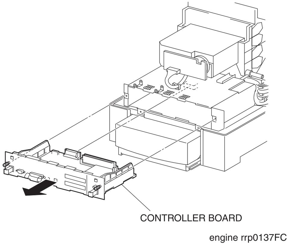
Figure: CONTROLLER BOARD Removal
