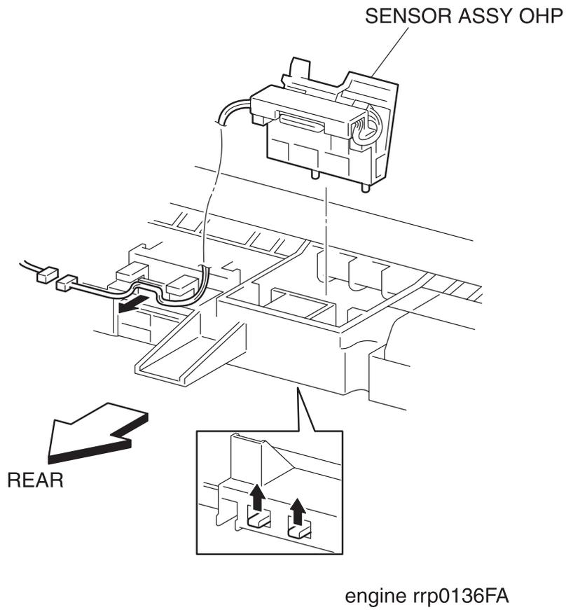
Figure: OHP SENSOR ASSY Removal (4)
