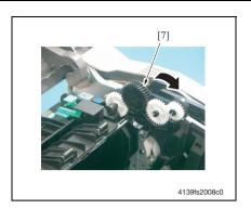
7. Swing open the Fusing Unit gear cover [7].
