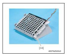
8. Remove the Duplex Cooling Fan Motor Cover [14].
