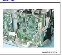
3. Disconnect all connectors and flat cables from the printer control board.
