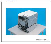
Lay the main body of the printer on its back.
