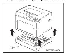
Lift the printer main body and then remove the Duplex option attachment [1] from the printer.
