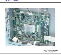
3. Disconnect all connectors and flat cables from the MFP board.
