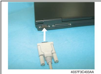
1. Connect the Crossing cable to the COM1 port on the PC.
