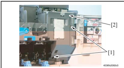
1. Remove the Control Panel.
