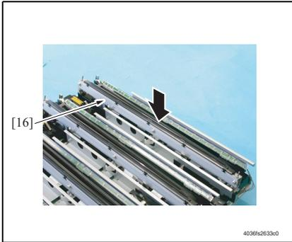
11. Press the LPH Assy [16] down into the locked position.
