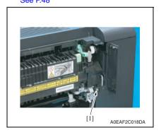
3. Open the cover and remove the screw [1].
