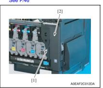
3. Remove the screw [1], and remove the right front cover [2].
