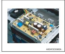
Disconnect all connectors on the DC power supply.
