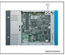
7. Disconnect two connectors [1] on the MFP board.
