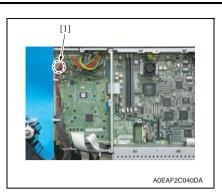
10. Disconnect the connector (PJ13A)[1] from the print control board.
