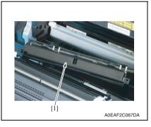
4. Unhook the spring, and remove the cover [1].
