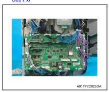
Remove all connectors on the FS control board.
