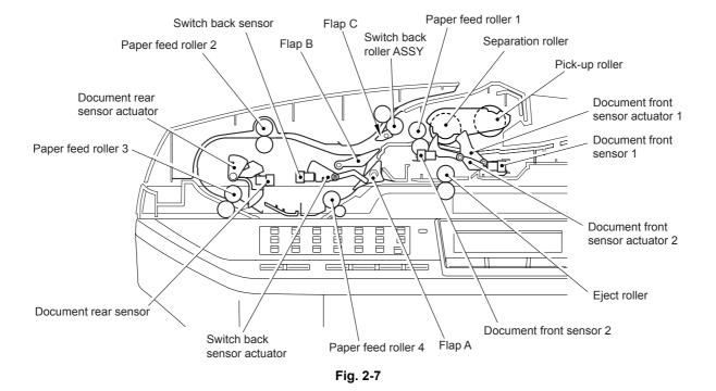
The duplex scanning mechanism allows you to use the following two types of scanning, "ADF scanning" and "document glass scanning". These two scanning methods are switched depending on whether the document front sensor 1 detects the document or not when starting scanning.
