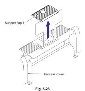
(8) Remove the Hook of the right side, and then remove the MP tray extention from the MP tray cover ASSY.
