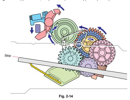
When the tray is pulled out from the machine, the pressure plate is returned to the original position. When the tray is put into the machine, the above operation is performed from the start again.
