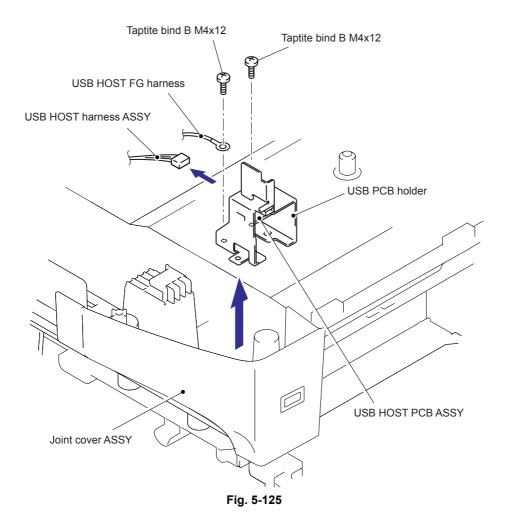
(5) Remove the cup S M3x6 SR Taptite screw, and remove the USB HOST PCB ASSY from the USB PCB holder.
