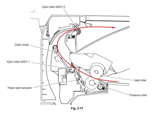
When a paper jam occurs, the main motor rotates conversely to throw out the engagement of the gear. Consequently, the eject roller ASSY 2 is released so that the jammed paper is removed easily.
