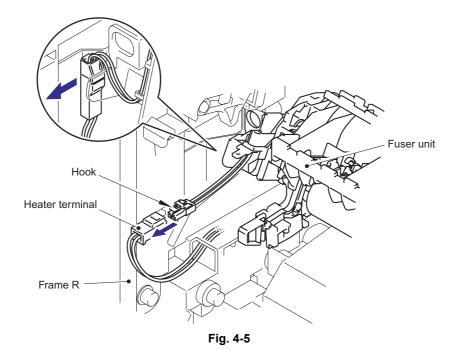
(10) Pull the FU harness cover 2 to the direction of 10a while pressing the Hook and pull out the FU harness cover 2 from the back of the machine.
