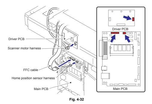
(18) Connect the six connectors of the each harness into the Main PCB.
