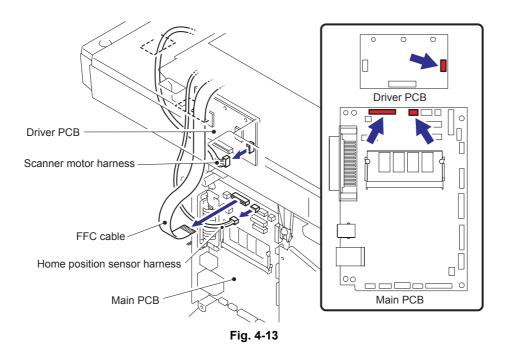
(21) Disconnect the six connectors of the each harness from the Main PCB.
