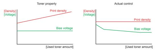
To obtain a print result of a constant density all the time, the machine counts the number of print pages immediately after the toner cartridge is replaced and changes the bias voltage according to the accumulated number of prints with the toner cartridge.
