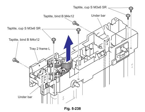
(3) Remove the two cup S M3x6 Taptite SR screws, and then remove the tray 2 paper feed frame.
