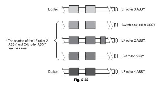
\* It is recommended to mark each of the roller ASSYs when disassembling them. Failure to assemble each roller ASSY onto the correct position may cause paper jam or stretching image.
