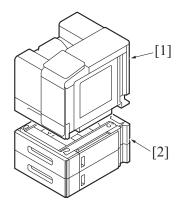
11. Lift the main body [1] and then remove the paper feed unit [2] from the main
