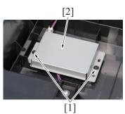
3. Remove two screws [1], and remove the cover [2].
