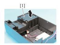
3. Remove the exhaust fan assy [1].
