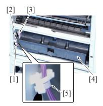
8. Remove four screws [1], and remove the plate [2].
