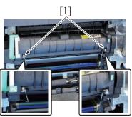
6. Hook two transfer unit pressers [1] on the fusing unit.
