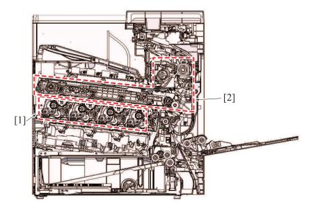
[1] Faulty spot responsible for an image trouble of the single-to-three-color system [2] Faulty spot responsible for an image trouble of the four-color system
