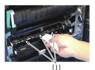
3. Using a cleaning pad with alcohol, wipe the registration roller [1] clean of dirt.
