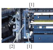
5. Remove the harness from the wire saddle [1] and the harness guide [2], and disconnect the connector [3].
