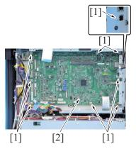
6. Remove nine screws [1], and remove the base board [2].
