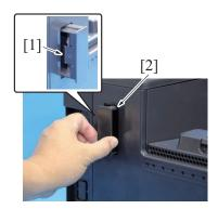
2. Unhook the tab [1], and remove the toner filter [2].
