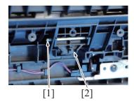
5. Slide the shaft [1], and remove the separation pad assy [2].
