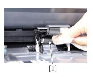
Using a cleaning pad dampened with alcohol, wipe the manual bypass tray feed roller [1] clean of dirt.
