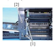
4. Remove two screws [1], and remove the front right cover/1 [2].
