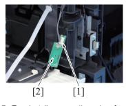
6. Disconnect the connector [1], and remove the NFC board [2].
