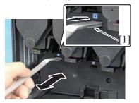
3. Clean the PH window by putting the PH window cleaning jig [1] back and forth a couple times.
