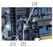
3. Remove the screw [1], and remove the harness guide [2] and the gear assy [3].
