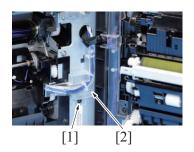
7. Remove the screw [1], and remove the cover [2].
