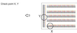
Adjustment for X direction: Check point X
