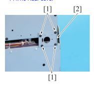
2. Remove four screws [1], and remove the plate [2].
