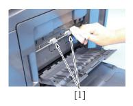
2. Using a cleaning pad dampened with alcohol, wipe the duplex unit transport roller [1] clean of dirt.
