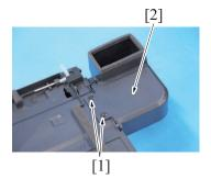
4. Remove two screws [1], and remove the duct [2].
