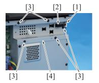
12. Remove five screws [1], and remove the paper feed unit [2].
