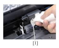
Using a cleaning pad dampened with alcohol, wipe the manual bypass tray pick-up roller [1].
