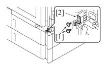
7. Remove two screws [1], and remove the plate [2].
