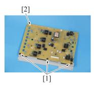
5. Remove the screw [1], and remove the cover [2].
