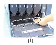
Wipe the areas [1] around the waste toner collecting port clean of spilled toner and dirt.
