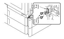
8. Remove two screws [1], and remove the plate [2].
