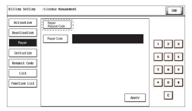
3. Write down or print out the serial number, repair request code and request code.
