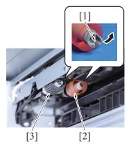
2. Unhook the tab [1], and remove the feed roller [2] and pick-up roller [3].
