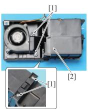
5. Remove four screws [1], and remove the exhaust fan/1/2 assy [2]
