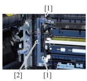
3. Remove two screws [1], and remove the cover [2].
