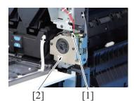
7. Remove the screw [1], and remove the USB hub board [2].
