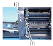
4. Remove two screws [1], and remove the front right cover/1 [2].
