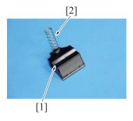
6. Remove the spring [2] from the separation pad [1].
