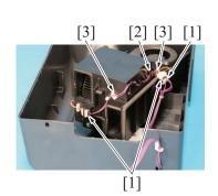
4. Disconnect three connectors [1], and remove the harness from the harness guide [2] and two wire saddles [3].
