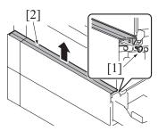
5. Remove the screw [1], and remove the cover [2].
