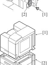
Lift the main body [1] and then remove the paper feed unit [2] from the main body.
