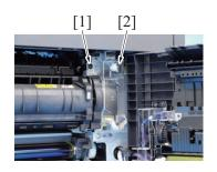
3. Remove the screw [1], and remove the cover [2].
