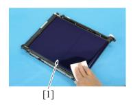
2. Using a hydro-wipe (65AA-99#), wipe the transfer belt [1].
