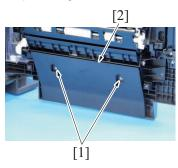
2. Remove two screws [1], and remove the cover [2].
