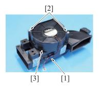
3. Remove the harness from two wire saddles [1], and disconnect the connector
