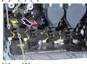
5. Remove two screws [3], and remove the imaging unit [4].
