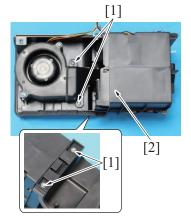
5. Remove four screws [1], and remove the exhaust fan/1/2 assy [2]
