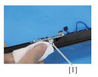
3. Wipe the IDC sensor window [1] clean of dirt.
