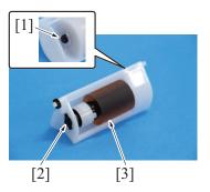
5. Remove the C-clip [1], pull out the shaft [2], and remove the tray 1 separation roller assy [3].
