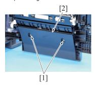
2. Remove two screws [1], and remove the cover [2].
