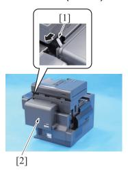
1. Push the lock shaft [1] to the left, and remove the clean unit [2].
