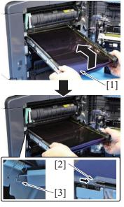
2. Hold up the transfer belt [1], and insert the transfer belt unit so that the groove [2] is along the rail [3].
