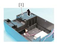
3. Remove the exhaust fan assy [1].
