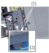
13. Remove two screws [1], and remove the boss [2].
