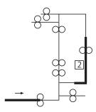
4. The second sheet of paper is taken up and fed in and the image of the fourth page of the original is printed. The first sheet of paper stops temporarily at the re-feeding position.
