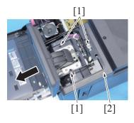
12. Remove three screws [1], and slide the cover [2].
