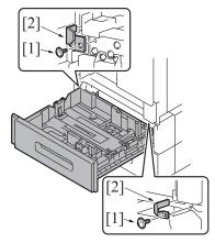
4. Remove two screws [1], and remove the two plates [2].
