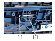
5. Slide the shaft [1], and remove the separation pad assy [2].
