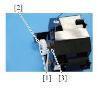
6. Remove two E-rings [1], the gear [2] and the bushing [3].
