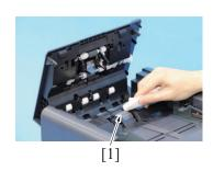
Using a cleaning pad dampened with alcohol, wipe the ADF separation pad [1] clean of dirt.
