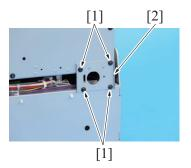
8. Remove four screws [1], and remove the plate [2].
