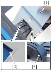
4. Raise the protrusion [2] of the cover [1] along the groove [3], and remove the cover [1].
