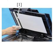
2. Using a cleaning pad dampened with alcohol, wipe the ADF paper guide [1] clean of dirt.
