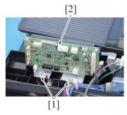
5. Remove two screws [1], and remove the DF control board assy [2].
