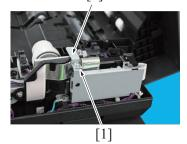
2. Remove two screws [1], and remove the fixing bracket [2].
