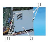
7. Remove five screws [1], and remove the plate [2].
