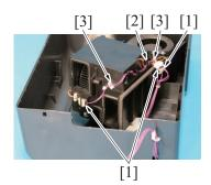
4. Disconnect three connectors [1], and remove the harness from the harness guide [2] and two wire saddles [3].
