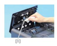
Using a cleaning pad dampened with alcohol, wipe the ADF feed roller [1] clean of dirt.
