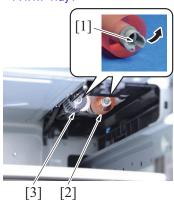
2. Release the tab [1] of each roller, and remove the tray 1 feed roller [2] and tray 1 pick-up roller [3].
