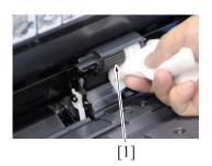
Using a cleaning pad dampened with alcohol, wipe the manual bypass tray pick-up roller [1].
