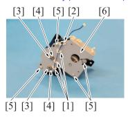
4. Remove the harness from three wire saddles [1] and the edge cover [2].5. Remove two E-rings [3], two bushings [4] and four screws [5], and remove the
