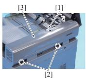
3. Remove the two screws [1], release two tabs [2], and remove the rear cover [3].
