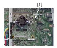
4. Remove the cable from the edge cover [1], and disconnect the connector [2].
