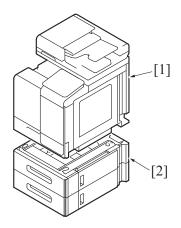
11. Lift the main body [1] and then remove the paper feed unit [2] from the main body.
