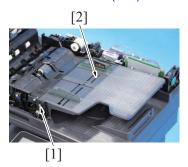
3. Remove the screw [1], and remove the document feed tray [2].
