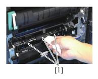
3. Using a cleaning pad with alcohol, wipe the registration roller [1] clean of dirt.
