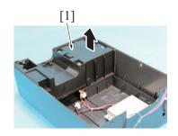
3. Remove the exhaust fan assy [1].
