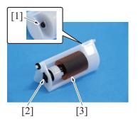
Remove the C-clip [1], pull out the shaft [2], and remove the tray 1 separation roller assy [3].
