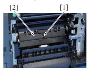
2. Remove the screw [1], and remove the cover [2].
