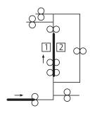
6. While the first sheet of paper is fed out, the second sheet of paper is taken up and fed in and the image of the fourth page of the original is printed.
