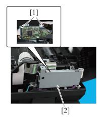
3. Pull out the DF CIS relay board assy [2], and disconnect two flat cables [1].
