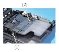
3. Remove the screw [1], and remove the document feed tray [2].
