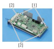
6. Remove four screws [1], and remove the DF control board [2].
