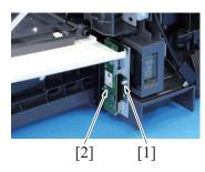
6. Remove the screw [1], and remove the wireless LAN board [2].
