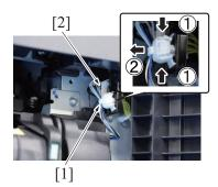
4. Remove the cable tie [1] from the main body, and disconnect the connector [2].
