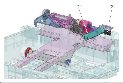
[1] Empty sensor actuator [2] Tray 2 paper empty sensor (PS1/2)
