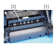
11. Remove the screw [1], and remove the guide [2].
