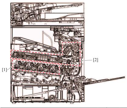
[1] Faulty spot responsible for an image trouble of the [2] Faulty spot responsible for an image trouble of the foursingle-to-three-color system color system
