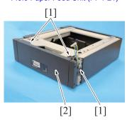
2. Remove three screws [1], and remove the rear over [2].
