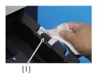
Using a cleaning pad dampened with alcohol, wipe the tray 1 separation roller [1] clean of dirt.
