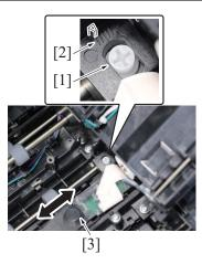
7. Rotate the adjustment screw [1], and slide the DF CIS module assy [3] while referring the graduation [2] to make adjustment.
