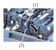
8. Remove the screw [1], and evacuate the stopper [2] of the DF CIS module.
