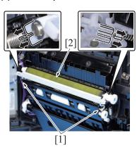
Holding onto the lock levers [1] (at two places), mount the new transfer roller unit [2].
