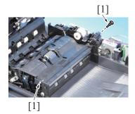
4. Remove the screw [1], and remove the document feed tray [2].
