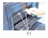
2. Using a cleaning pad dampened with alcohol, wipe the duplex unit transport roller [1] clean of dirt.
