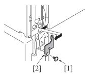
9. Remove the screw [1], and remove the plate [2].
