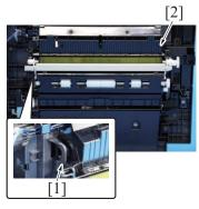
6. Unhook the hook [1], and remove the 2nd transfer pressure unit [2].
