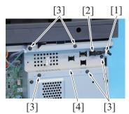
Remove the cable from the edge cover [1], and disconnect the connector [2].
