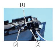
3. Remove two screws [1], and remove the plate [2].
