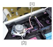
5. Remove two screws [1], and slide out the fax speaker [2].
