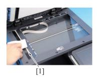
3. Using a cleaning pad dampened with alcohol, wipe the document reading glass [1] clean of dirt.
