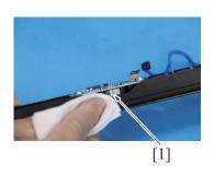
3. Wipe the IDC sensor window [1] clean of dirt.
