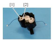
6. Remove the E-ring [1] and remove the transport clutch [2].
