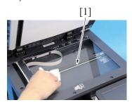
2. Using a cleaning pad dampened with alcohol, wipe the original glass [1] clean of dirt.
