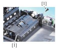
Slide the CIS module assy [2] to the position shown in the illustration while holding the belt [1].
