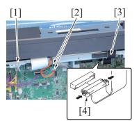
11. Raise the DF CIS module assy [1], and remove the flat cable [3] from the harness guide [2].
