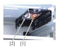
2. Using a cleaning pad dampened with alcohol, wipe the tray 1 feed roller [1] and tray 1 pick-up roller [2] clean of dirt.
