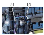
3. Remove the screw [1], and remove the harness guide [2] and the gear assy [3].
