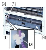
9. Remove five screws [1], and remove the plate [2].
