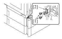
7. Remove two screws [1], and remove the plate [2].
