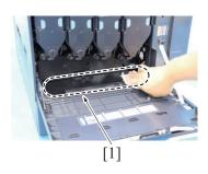
2. Wipe the areas [1] around the waste toner collecting port clean of spilled toner and dirt.
