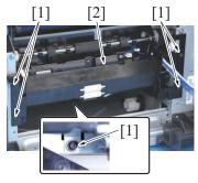
12. Remove five screws [1], and remove the paper feed unit [2].
