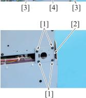
6. Remove four screws [1], and remove the plate [2].
