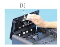
2. Using a cleaning pad dampened with alcohol, wipe the ADF pick-up roller [1] clean of dirt.
