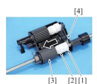
6. Slide the gear [1], gear [2] and feed roller [3], and remove the pin [4].
