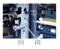
7. Remove the screw [1], and remove the cover [2].
