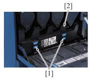
2. Hold the both handles [1], and remove the waste toner bottle [2].
