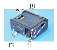
5. Remove six screws [1], remove the clean unit cover assy [2].
