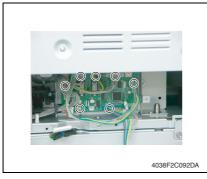
Remove all the Connectors on the Tray 2 Control Board.
