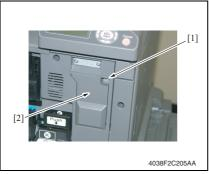
5. Remove the Screw [1], and remove the Connector protective cover [2].
