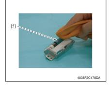
Using the soft cloth dampened with alcohol, wipe the Bypass Paper Separation Roller [5].
