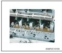
Remove all the Connectors and the Flat Cables on the PH Interface Board.
