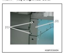
1. Remove two Screws [1], and remove the Tray 2 Right Rear Cover [2].
