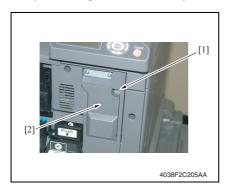
6. Remove the Screw [1], and remove the Connector protective cover [2].
