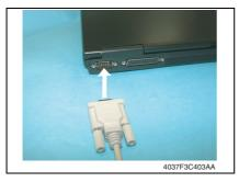
Connect the Crossing cable to the COM1 port on the PC.
