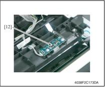
Repeat the step 6 and 7, and remove the IDC/Registration Sensor/2 (rear side) [12].
