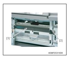
4. Remove the Screws [2] and remove the Reinforcement plate [3].
