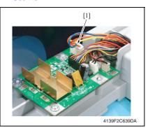
4. Disconnect the connector (PA01) [1] from the DF control board.
