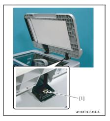
Loosen the one screw [1] in the back to the right.
