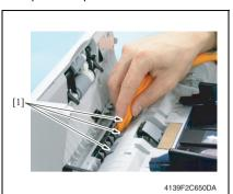
Wipe the registration rollers [1] clean of dirt using a soft cloth dampened with alcohol.
