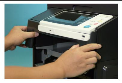
4. Disconnect the connector (A) and then remove the scanner front cover.
