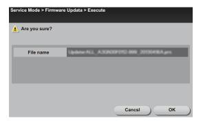
9. The firmware upgrading procedure starts.
