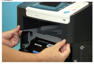
3. Hold the sections shown in the illustration of the scanner front cover and unhook the two tabs in such a way as to lower the cover while pulling it toward.
