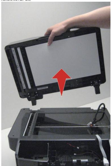
Installation note: After the new ADF is installed, perform scanner manual registration, see I.4.17 ADF Adjustment.
