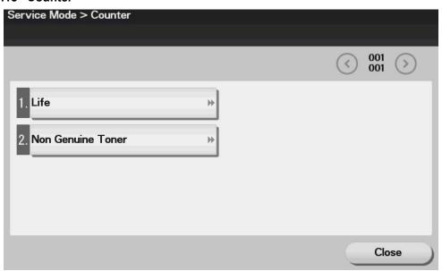
· The counter displays the counts of various counters to allow the technical representative to check or set as necessary.
