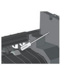
$\it 5$ . Squeeze the latches to release, and dislodge the interface cable from its slot.
