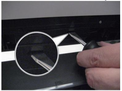
3. Disconnect the blade fastener (A) holding the ground cable to the ADF relay board.
