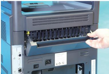
2. Pull the exit door upward to release the hinges, and remove.
