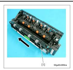
4. Slide the fusing front guide assy [1] for removal.
