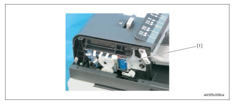
[1] Pressure roller release solenoid (SD1)
