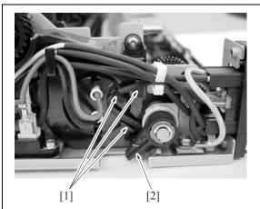
• When installing the fixing claw unit, be careful that the edge of the fixing claw pressing spring [1] does not run on the web case.
