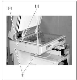
Remove the 7 screws [1] and remove the scanner exterior/F [2].
