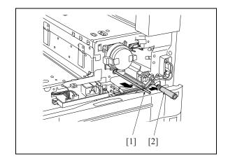
6. Remove the 11 screws [1], and remove the write cover [2].
