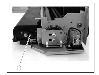
When installing the fixing claw unit, be careful that the edge of the fixing claw pressing spring [1] does not run on the web case.
