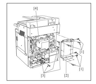
Remove the various wiring connectors from the SCB (System control board) [1].
