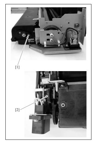
• When returning the wiring harness, be sure to hook the wiring harness securely on the wiring harness holder section [1] so that it does not interfere with the web operation lever [2].
