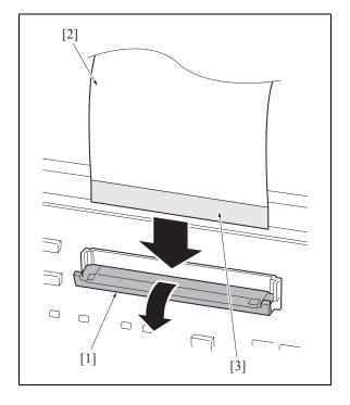
2. Push back the lock lever [1] to lock the ribbon cable [2].
