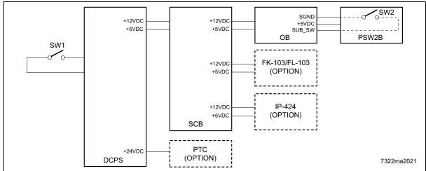
Setting the SW1 (Main power switch) to the ON position supplies AC power to the DCPS (DC power source) which in turn supplies +12DVC and +5DVC to the SCB (System control board). The DCPS also supplies +5DVC to the OB (Operation board) through the SCB.
