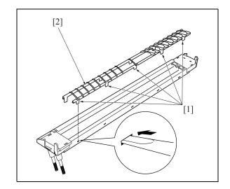
3. Remove the spark arrestor plates/F [1], /R [2].
