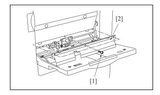
3. Remove the 2 screws [1], then remove the bypass sensor.
