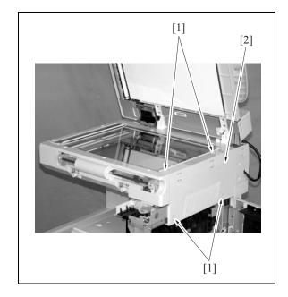
4. Remove the 4 screws [1] and remove the scanner exterior/L [2].
