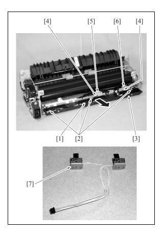
• When returning the fixing web in use, be sure to rotate the web drive gear until the original web winding shaft [1] starts to turn.
