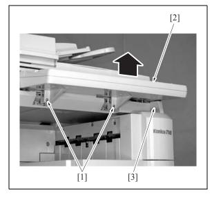
4. Loosen the 2 screws [1] and remove the front cover [2] and the front door [3].
