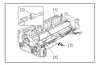
When returning the fixing web in use, be sure to rotate the web drive gear until the original web winding shaft [1] starts to turn after the assembling.
