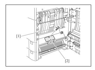
3. Remove the 2 stop rings [1] and the bearing [2] on this side, and remove the paper feed roller unit [4] by sliding the bearing [3] on the rear side to the rear.
