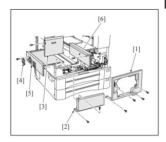
5. Remove the write cleaning knob [2] from the dust proof glass cleaning rod [1] and then puch the rod [1] to inside of main body.
