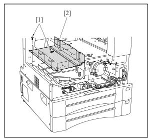
7. Remove the two write unit mount pieces [2] (each is held in place by screw [1]).
