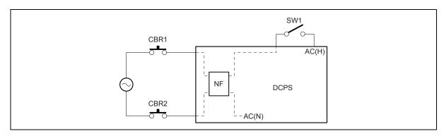
The follwing components are powered regardless of whether the SW1 (Main power switch) is on or off, provided that the power cord remains plugged in.
