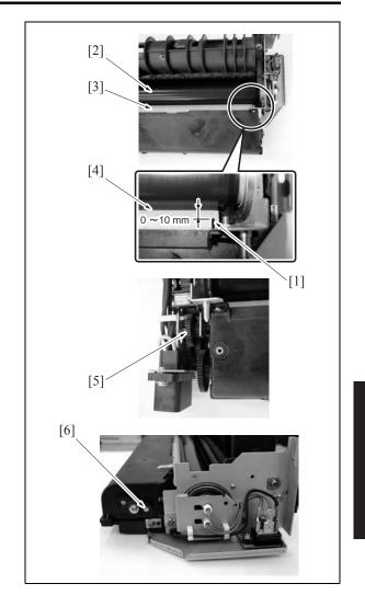
• When installing the fixing claw unit, be careful that the edge of the fixing claw pressing spring [1] does not run on the web case.
