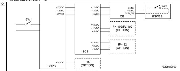
Setting the SW1 (Main power switch) to the ON position supplies AC power to the DCPS (DC power source) which in turn supplies +12DVC, -12VDC, and +5DVC to the SCB (System control board). The DCPS also supplies +5DVC to the OB (Operation board) through the SCB.
