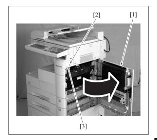
3. Remove the 2 angle adjusting screws [1], and remove the operating section stopper [3] while lifting up the operating section [2].
