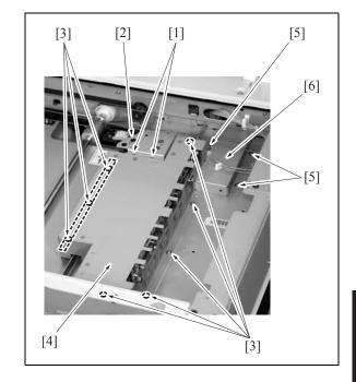
5. Remove the ribbon cable [2] from the ADB (A/D conversion board) [1].
