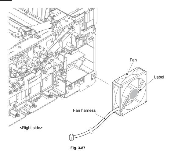
Harness routing: Refer to "8. Fan harness, Fan FG harness".
