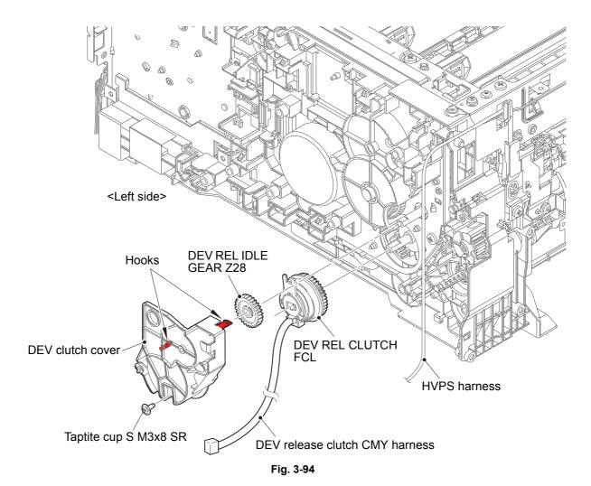
Harness routing: Refer to "3. DEV release clutch CMY harness, 10. HVPS harness".
