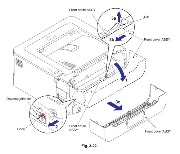
(4) Remove the Support flap 1 from the Front cover ASSY.
