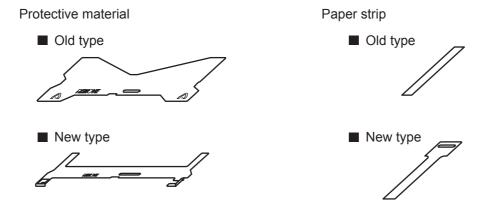
Make the protective material of drum unit by the following procedures, and use it at the time of packing.
