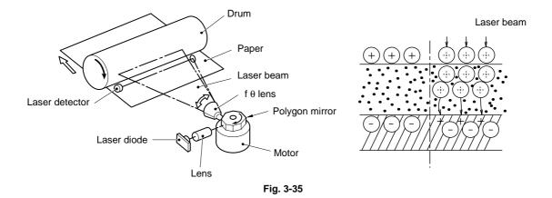
The area exposed to the laser beam is the image to be printed. The surface potential of the exposed area is reduced, forming the electrostatic image to be printed.
