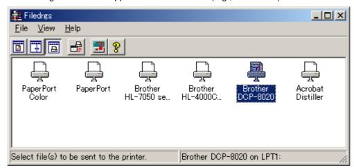
(5) Drag and drop the update data onto the icon of the model being used in the Filedrgs windows.
