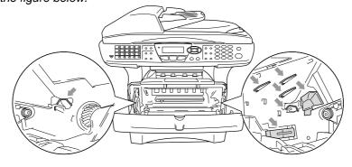
(3) While pressing the blue lock lever, take the toner cartridge out of the drum unit assembly.
