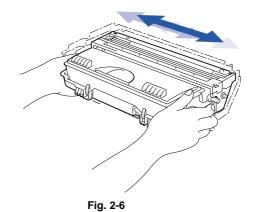
(4) Push the drum unit assembly into the machine (until it snaps into place).
