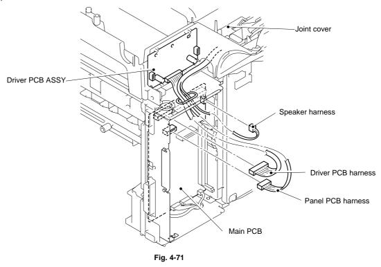
(2) Remove the four bind B M4x12 Taptite screws, and then remove the joint cover.
