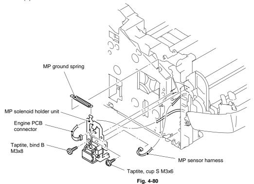
(5) Remove the cup S M3x6 Taptite screw, and then open the MP chute ASSY cover.
