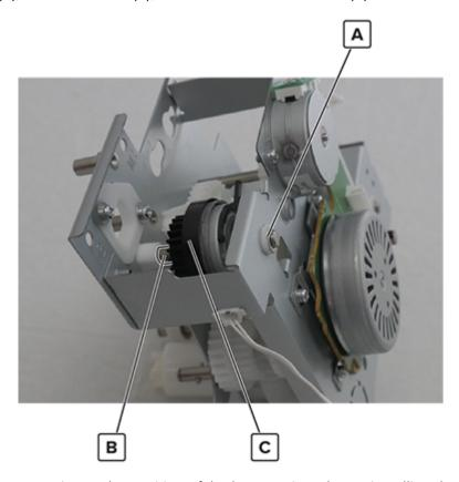
**Installation note:** Pay attention to the position of the locator pins when reinstalling the clutch.
