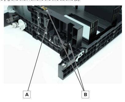
**3** Remove the sensor from its housing on the division board.
