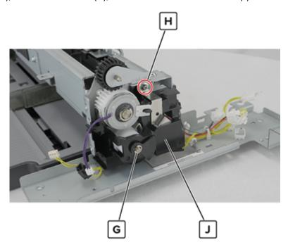
Warning—Potential Damage: Do not lose the ground plate and solenoid actuator.
