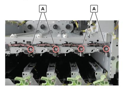
**9** Move the cable guide out of the way, and then remove the LED.
