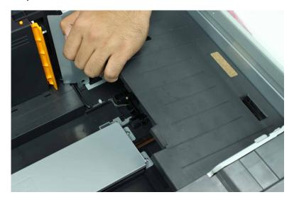
**3** Rotate the actuator (C) until it is in the upright position, and then slide out to remove.
