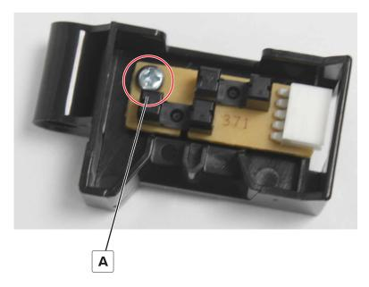
**Installation note:** Toggle the sensor to make sure that it bounces back.
