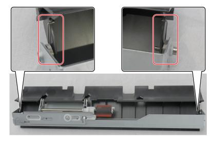
${\bf 6}\;$  Remove the two screws (J), and then remove the separator assembly (K).
