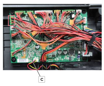
**5** Remove the J18 cable (C) from the cable harness, and then remove the motor.
