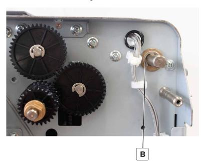
**9** From the other end of the shaft, remove the clip (C), and then remove the bushing.
