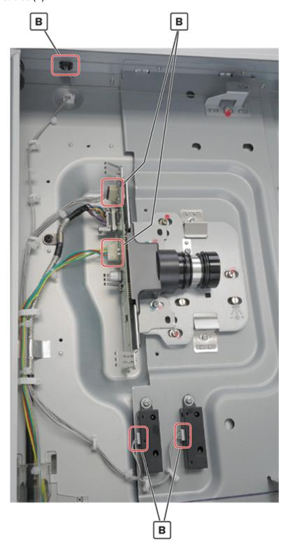
**11** Release the tab, and then remove the cable guide.
