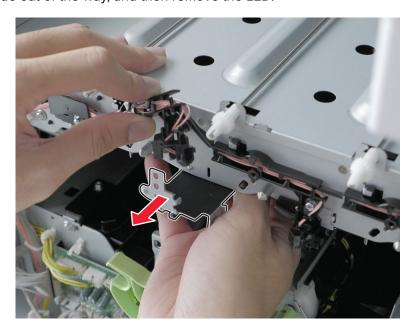
**Installation note:** Insert the tip of the LED bracket to its slot (A) at the back.
