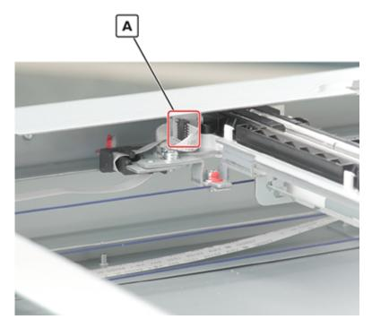
**10** Pry the guide to release, and then pull it off the frame.
