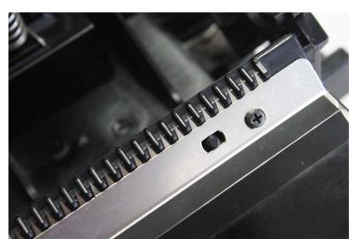
**Installation note:** Align the two springs while pushing down the assembly, and then move the assembly to the left to lock.
