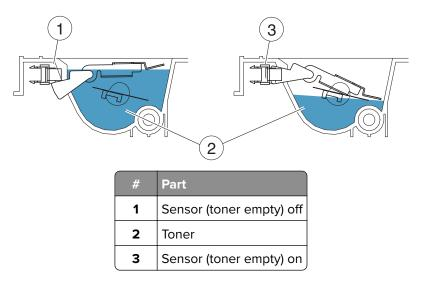
The motor (toner supply) of each color drives the toner conveying screw and toner agitating blade. The toner agitating blade rotates to agitate toner in the toner hopper. The toner conveying screw rotates to replenish the developer unit with toner.
