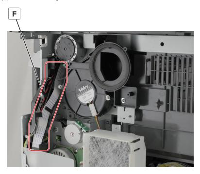
8 Remove the paper exit fan. See "Paper exit fan removal" on page 639.
