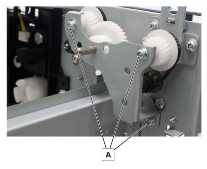
7 Remove the three gears and two belts.
