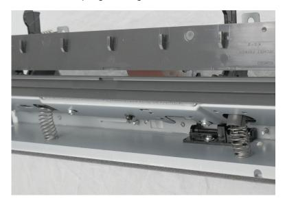
**7** Remove the eight screws (B, C), and then remove the bracket.
