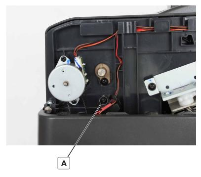
**3** Disconnect the cable, and then remove the sensor.
