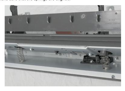
**7** Remove the eight screws (B, C), and then remove the bracket.
