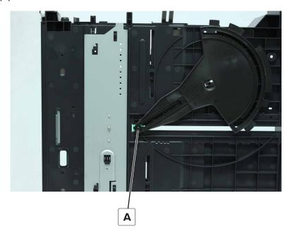
4 Raise the lift plate, move the length guide slightly under the lift plate, and then remove the guide.
