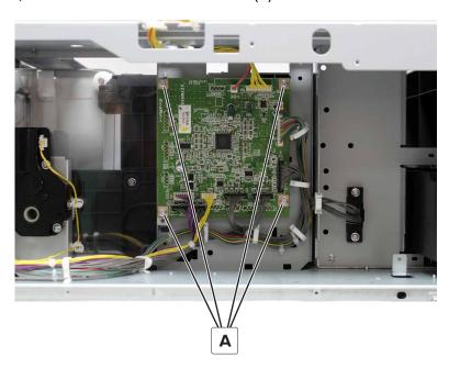
**3** Remove the controller board.
