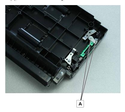
**6** Separate the registration unit handle from the registration unit lock shaft.
