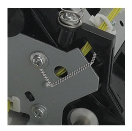
8 Disconnect the two cables (C), remove the cables from the cable guides, and then remove the bracket (D).
