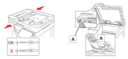
**Note:** Make sure that the protrusion on the ADF and flatbed scanner has no clearance.
