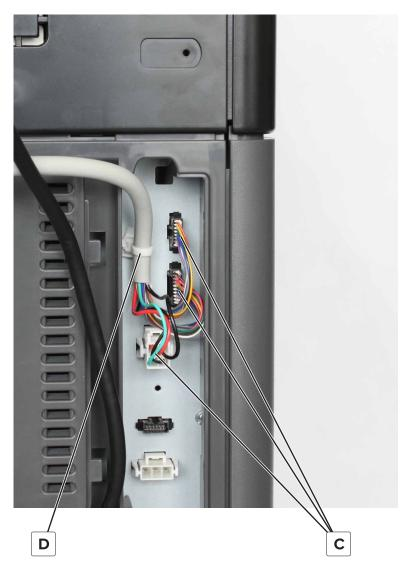
**7** Open the ADF, and then remove the two screws (D).
