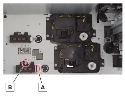
**3** Remove the sensor housing, and then remove the sensor.
