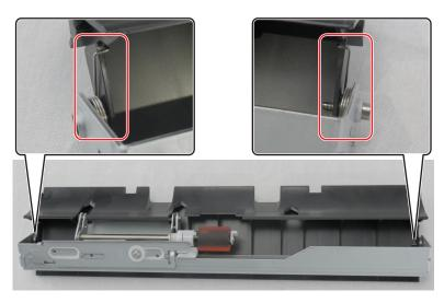
4 Remove the two screws (C), and then remove the separator assembly (D).
