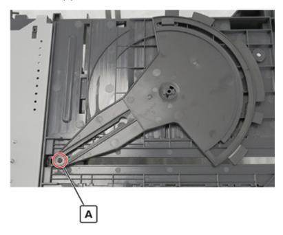
**4** Remove the sensor actuator.
