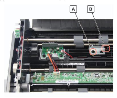
**5** Remove the sensor from its bracket.
