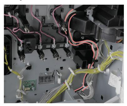
**26** Release the cable guide (D), remove the five screws (E), and then pull the bracket.
