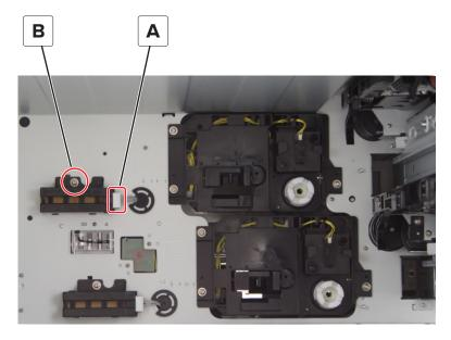
**3** Remove the sensor housing, and then remove the sensor.
