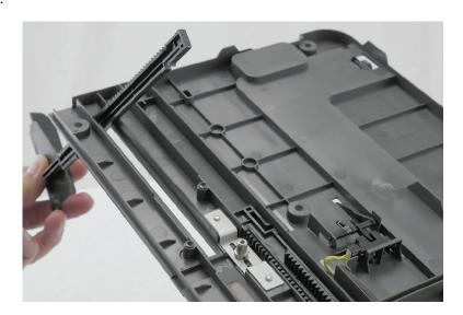
**Installation note:** Take note of the positions of the gear and dots.
