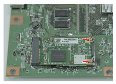
**Installation warning:** To avoid data corruption, do not remove and install the eMMC and EEPROM (A) from one engine board to another as a method of troubleshooting.
