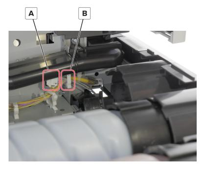
**5** Disconnect the motor cable, and then remove it.
