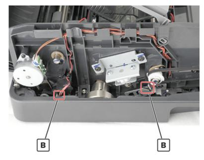
8 Disconnect the sensor cable J15 from the controller board, and then remove it.
