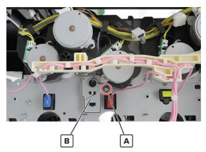
**13** Remove the sensor from the bracket.
