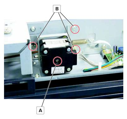
**Note:** Do not fully tighten the screws.
