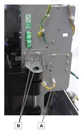
**3** Lift the registration unit to release, and then remove.
