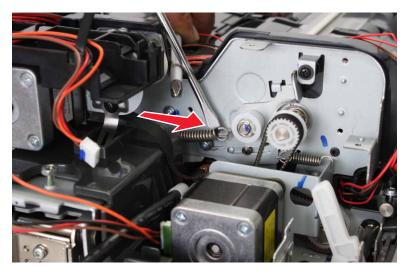
**c** Replace the motor, and then loosen the screw to engage the belt onto the motor.
