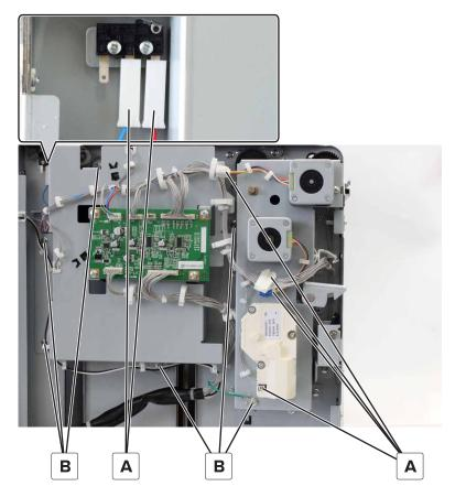
**5** Disconnect the cable, and then remove the sensor.
