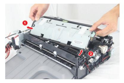
**8** Remove the screw (B), and then remove the cover.
