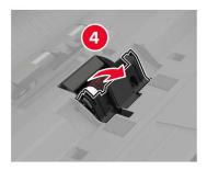
2 Remove the ADF separator roller, and then remove the ADF separator roller spring.
