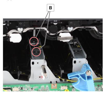
**7** Remove the housing, and then separate it from the contact.
