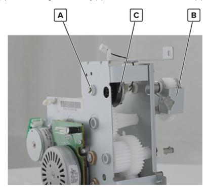
**Installation note:** Pay attention to the position of the locator pins when reinstalling the clutch.
