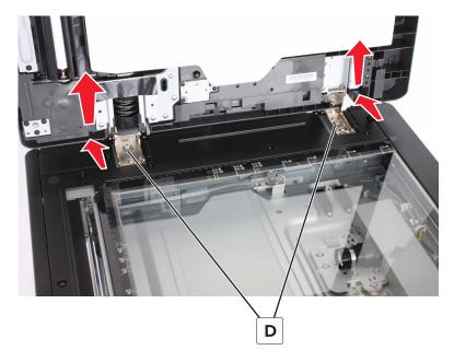
Warning—Potential Damage: Be careful not to break the ADF angle open actuator.
