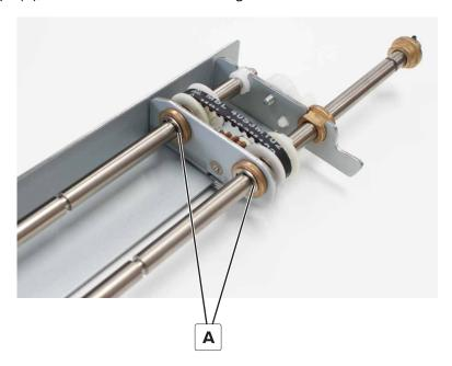
**3** Remove the two clips (B), and then remove the two bushings.
