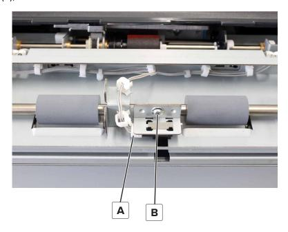
**7** Remove the adhesive (C), and then remove the sensor.
