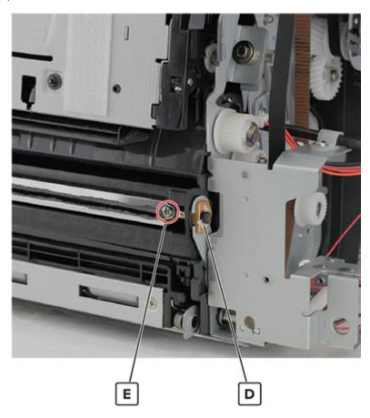
**10** Remove the cleaning shaft with scan glass cleaner, and then separate the shaft from the cleaner.
