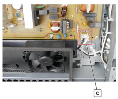
**9** Remove the cable from the switch.
