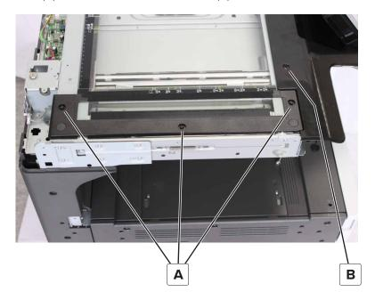
6 Slightly raise the scanner front cover, and then remove the ADF duplex scan glass.
