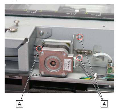
**4** Release the belt from its motor and gear, and then remove it.
