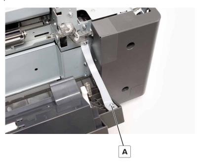
**3** Pry the right hinge to release, and then remove the cover.
