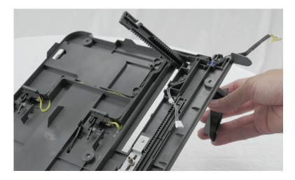
**Installation note:** Take note of the positions of the gear and dots.
