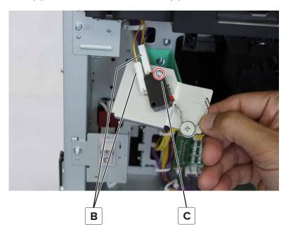
**5** Release the retainer, and then remove the switch.
