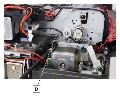
**b** Use a flat-head screwdriver to push the spring toward the left of the ADF, and then retighten the screw.
