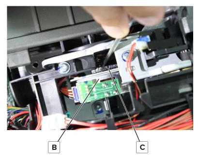
**4** Disconnect the cable from the motor, and then remove the motor.
