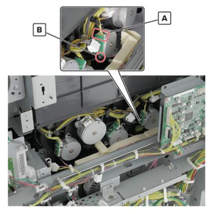
Note: Turn the motor counterclockwise to remove it.
