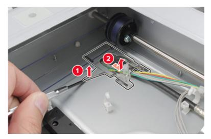
**12** Disconnect the cable (C) from the scanner controller board.
