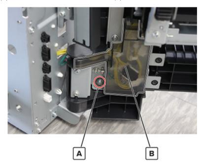
**3** Disconnect the two cables (B), and then remove the cables from the cable guides.
