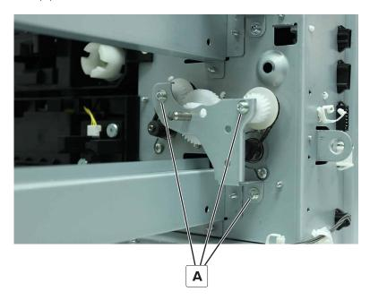
**6** Remove the three gears and two belts.
