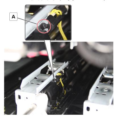
**Installation note:** Make sure that the spring is properly installed.
