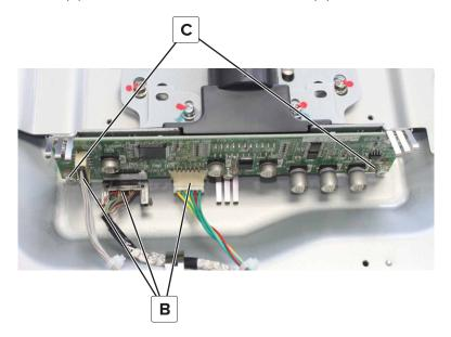
**Installation note:** Make sure to reinstall the scanner CCD cable with its metal component facing up.
