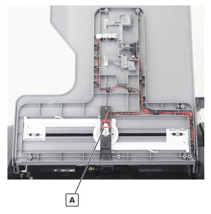
**Installation note:** Move the ADF paper guide racks to their farthest positions. Make sure that the gear hole (A) is positioned as shown.
