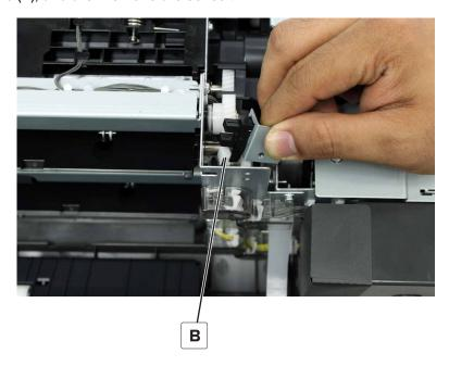
Remove the sensor from the bracket.
