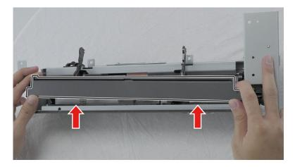
**Installation note:** Make sure that the springs are aligned.
