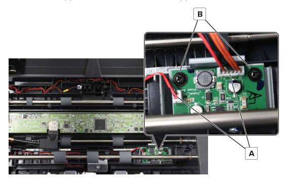
**4** Remove the ADF CIS power supply board.
