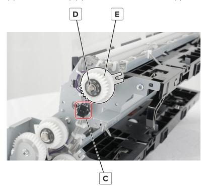
**Installation note:** Pay attention to the position of the tab locator on the clutch.
