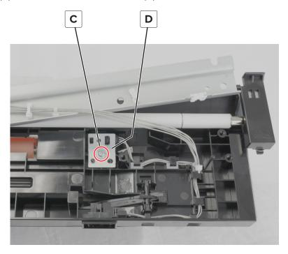
**4** Disconnect the cable (E), and then remove the sensor from the bracket.
