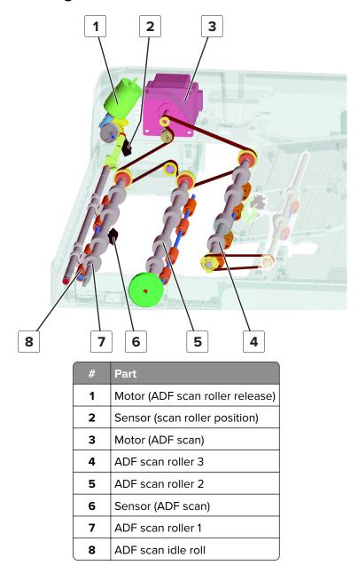
The motor (ADF scan) drives the ADF scan rollers 1, 2, and 3 to transport the document into the document scanning section. The sensor (ADF scan) detects the document after the leading edge passes through the ADF scan roller 1.
