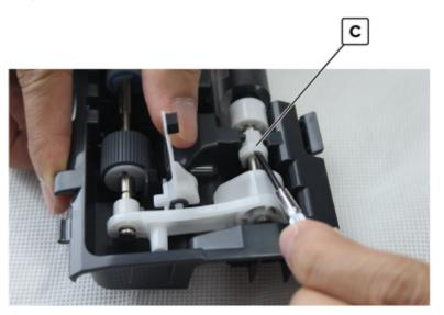
**4** Move the bushing to unlock the roller shaft.
