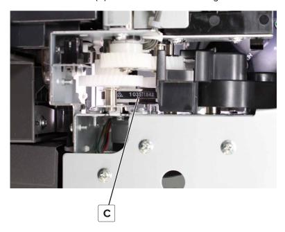
**Installation note:** Make sure that the feed motor belt is installed properly before installing the feed motor.
