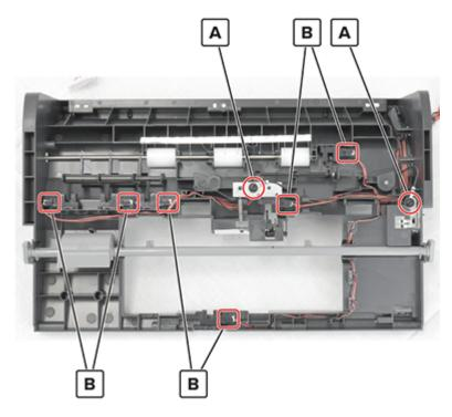
**4** Separate the ADF ground cable from the ADF top cover sensor cable.
