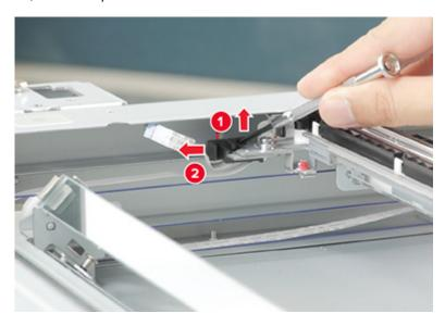
**11** Release the cable from its guide.
