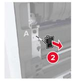
**3** Loosen the screws that secure the transfer belt.
