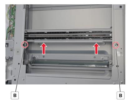
**18** Remove the bracket (C) on each end of the scanner carriage.
