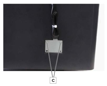
**5** Remove the plate, and then remove the cover.
