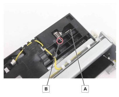
**7** Remove the shaft, and then remove the actuator.
