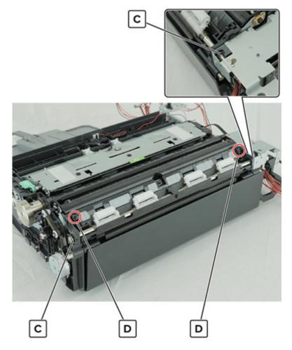
**9** Slide the shaft to release, and then separate the ADF scan roller 1 backup roller from the ADF scan deflector.
