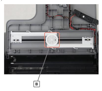
**Installation note:** Move the ADF paper guide racks to their farthest positions. Make sure that the gear hole (A) is positioned as shown.
