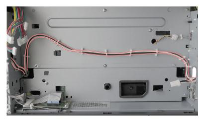
**24** Disconnect the cable (C) from the rear side, and then release it from its guides.
