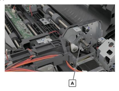
**7** Remove the screw (B), and then remove the bushing.
