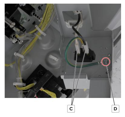
**7** Remove the socket from the power socket mounting plate.
