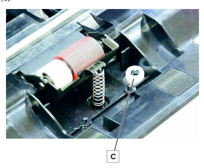
**4** Set the spacer on the lower part of the spring with its deeper groove facing up.
