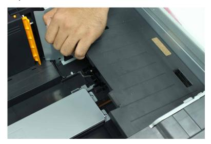
**3** Remove the actuator (C).
