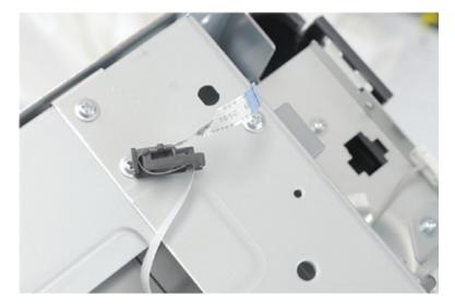
12 Release the latch, and then pull the cable guide off the frame.
