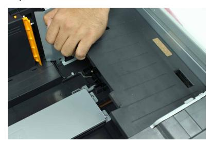
**3** Remove the actuator (C).
