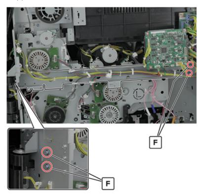
**10** Remove the cables from the guides on the bracket, and then remove the bracket.
