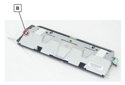
7 Remove the E-clip (B), and then remove the gear.
