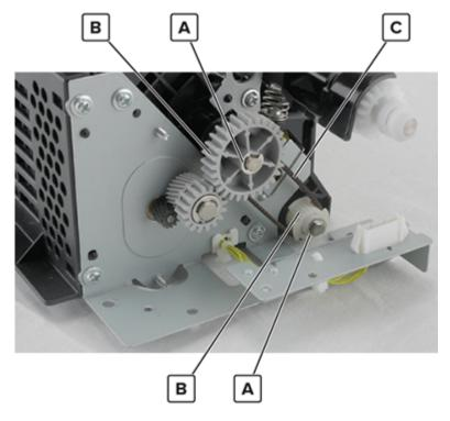
Warning—Potential Damage: Do not lose the washers.
