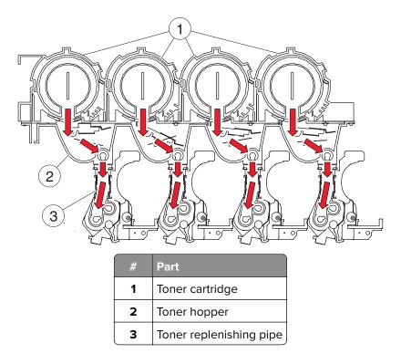
The toner hopper of each color has a sensor (toner empty). When toner is low in the toner hopper, the sensor (toner empty) is triggered. The motor (toner cartridge) turns for a predetermined period to supply toner to the toner hopper.
