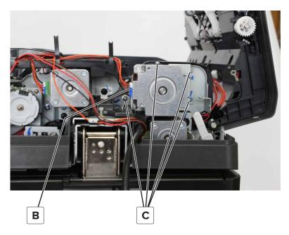
**5** Remove the motor from its bracket.
