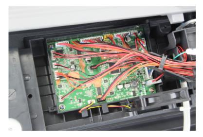
**5** Disconnect the cable (A), remove the four screws (B), and then remove the motor bracket.
