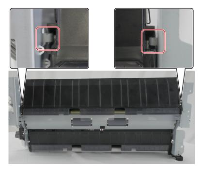
**5** Remove the screw (G), and then remove the feed guide (H).
