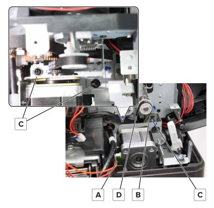
**5** Remove the motor from the ADF, and then remove the motor from the bracket.
