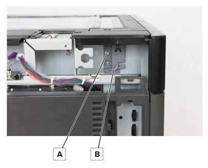
**4** Disconnect the cable from the sensor.
