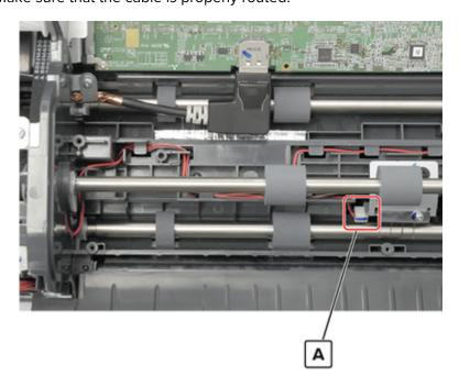
4 Disconnect the sensor cable J10 from the controller board, and then remove it.
