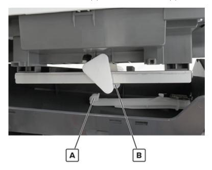
**4** Unhook the spring from the lock, and then remove the lock.
