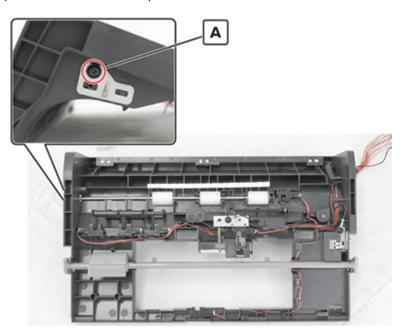
**Installation note:** Take note of the alignment of the arrow with the lines on the plate.
