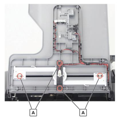
**4** Remove the gear, and then remove the racks.
