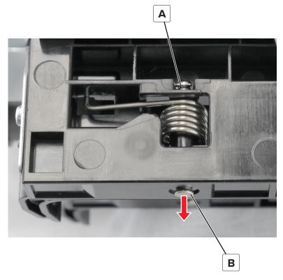
**3** Unhook the spring (C), and then remove the actuator (D).
