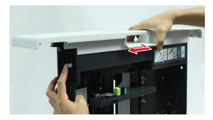
**4** Disconnect the spring (B) from the tray, and then remove the shaft.
