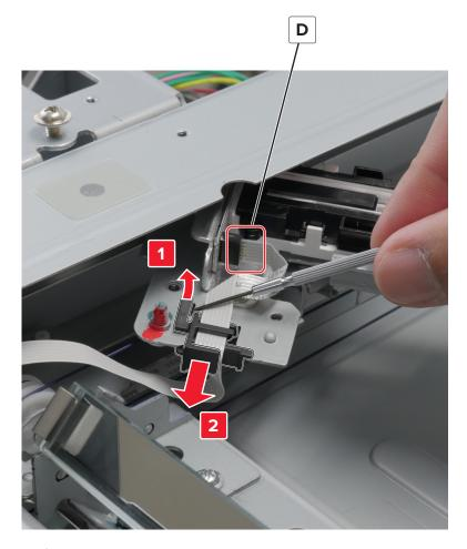
**20** Remove the scanner carriage.
