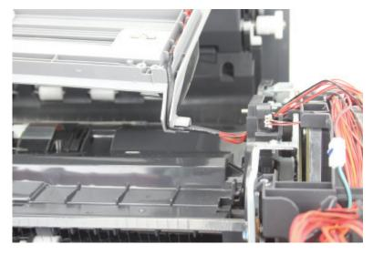
**5** Disconnect the connectors (A), and then remove the cable.
