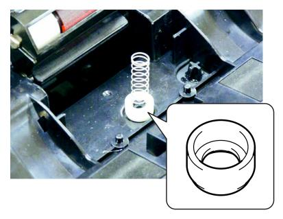
**5** If the spring force is not enough, set the spacer on the lower part of the spring with its shallow groove facing up.
