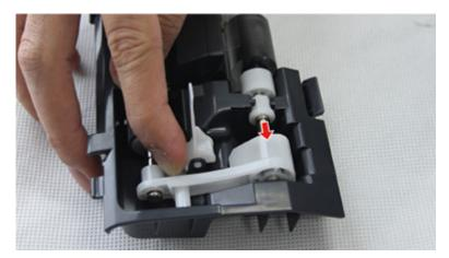
**5** Lift the roller assembly, and then remove the clip (D).
