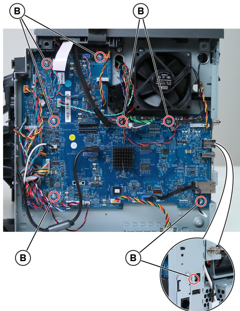
5 Remove the controller board.
