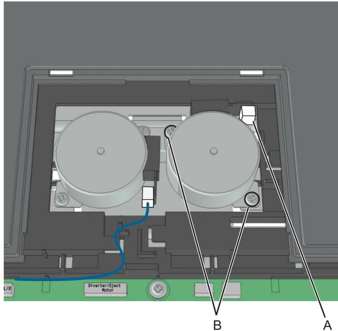
**Warning—Potential Damage:** Be careful not to lose the tamper belt when removing the motor.
