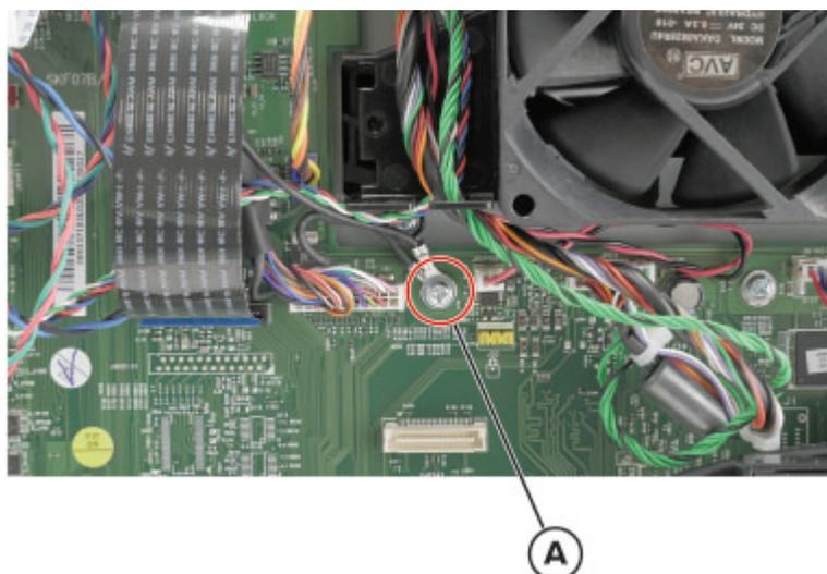
**4** Remove the scanner rear cover. See [“Scanner rear cover removal” on page 286](#).
