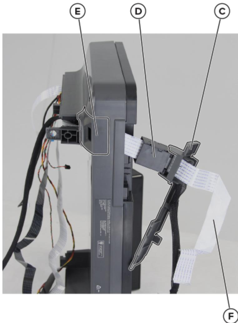
**Note:** Pay attention to the routing of the ADF flat cable and of the double-sided part of the cable.
