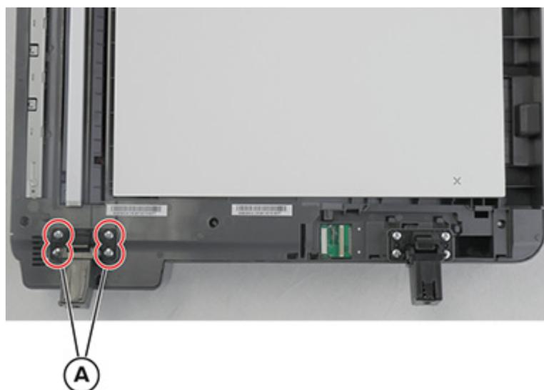
**Installation note:** When installing the left hinge, make sure that the extension (A) is facing to the left.
