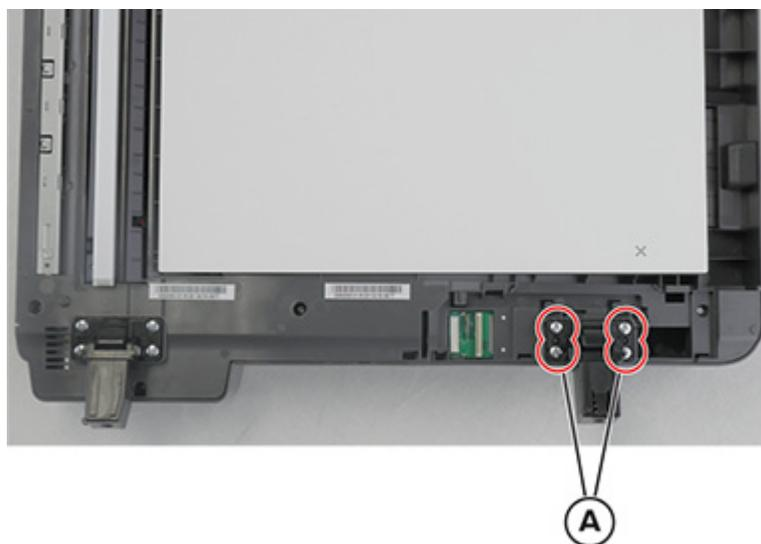
**Installation note:** When installing the right hinge, make sure that the latch (A) is positioned as shown.
