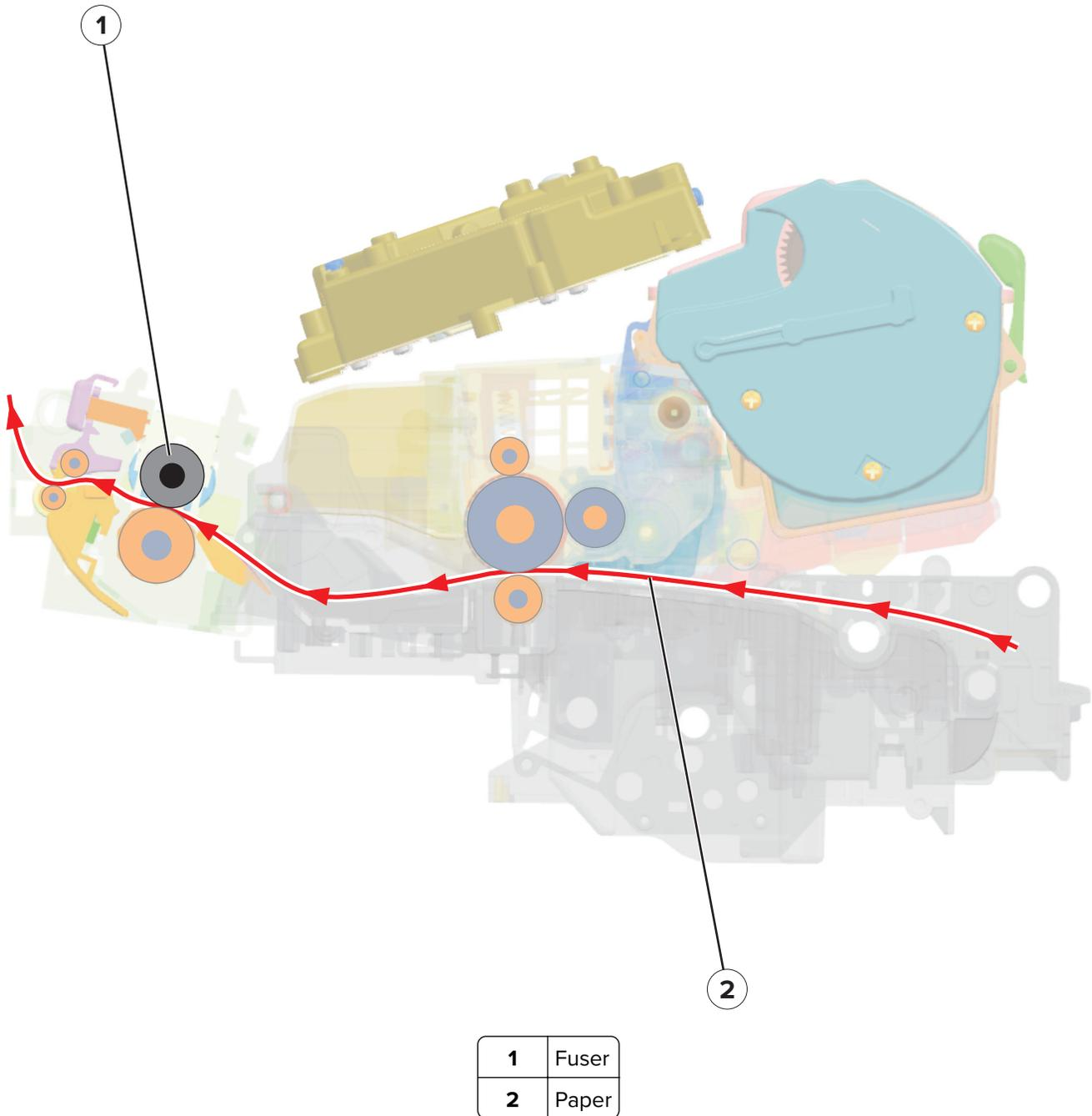
Even if the toner image is already on the paper, the toner particles are not yet permanently bonded to the surface. For the final part of printing, the paper is transported to the fuser where heat and pressure are applied to it. As a result, the toner particles melt and permanently fuse with the paper, completing the print process. The print cycle repeats for the succeeding pages.
