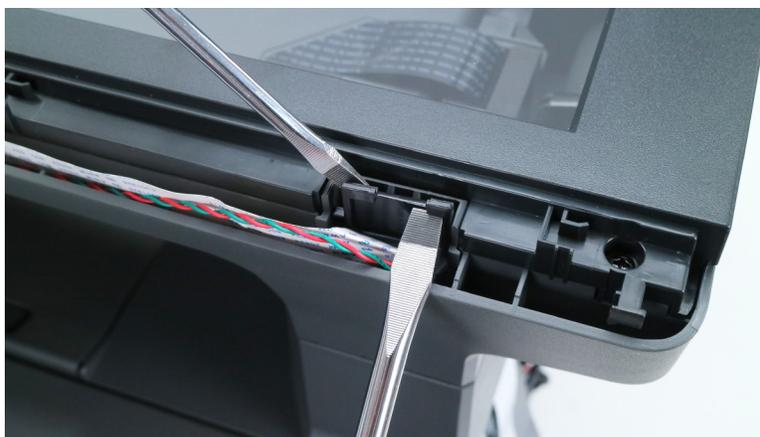
**Installation note:** Make sure that the flat cable is inserted as shown.
