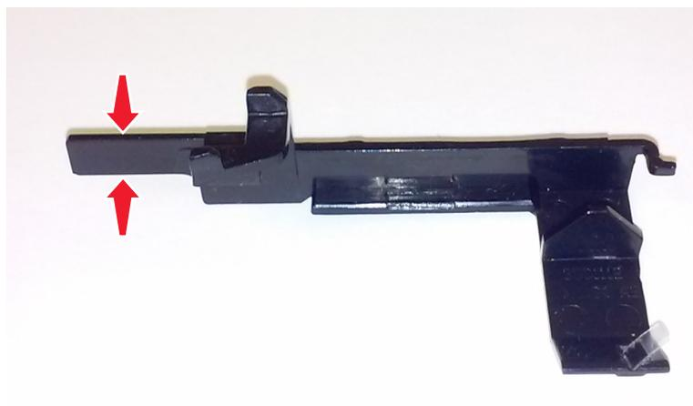
**b** Apply RheoGel 793 to the point of contact between the bracket (A) and cam.
