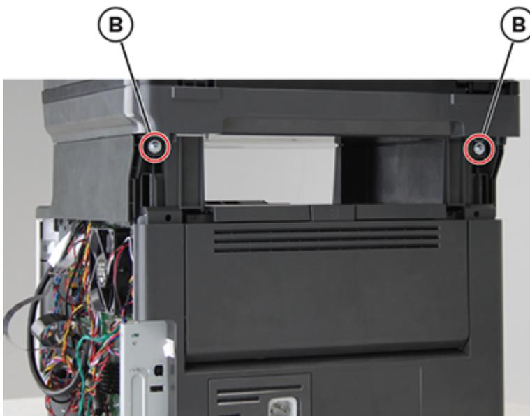
**6** Remove the flatbed scanner assembly.
