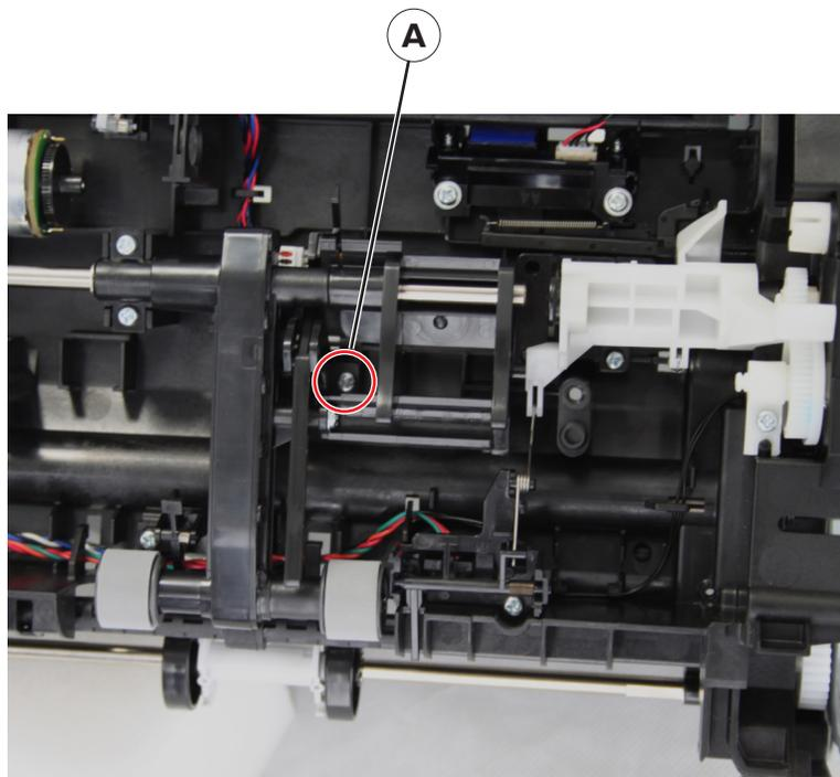
5 Lift the pick roller assembly, and then rotate the sensor flag to remove it.
