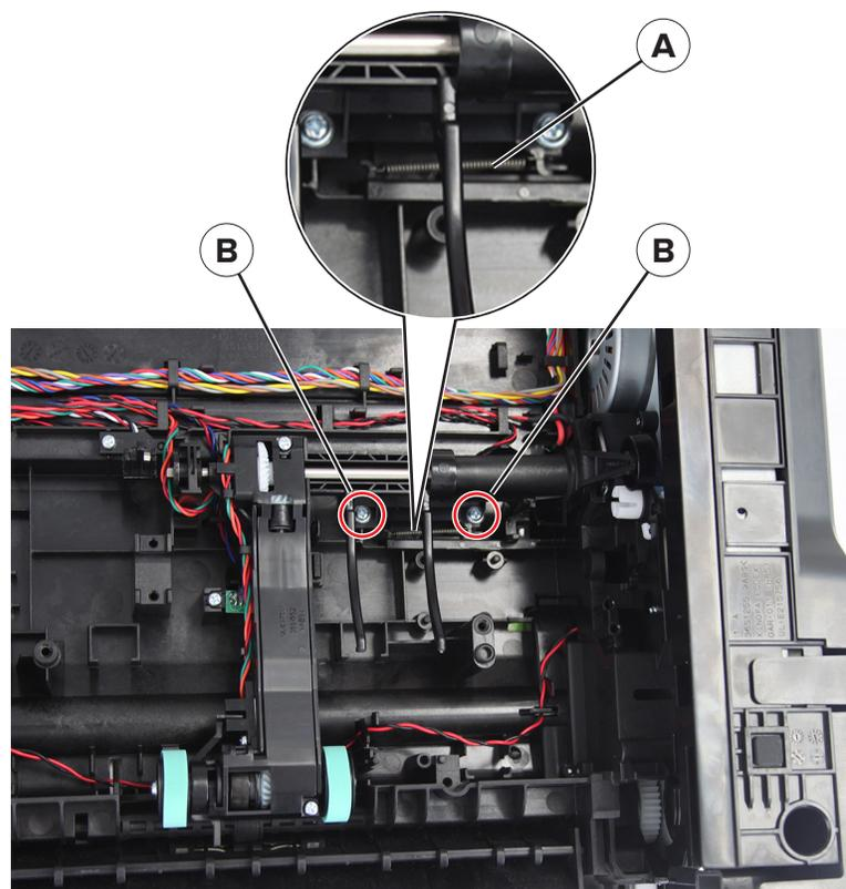
**6** Disconnect the cable, and then remove the sensor.
