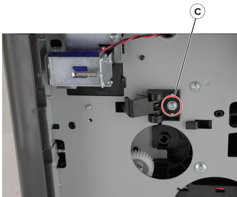
5 Remove the fuser actuator.
