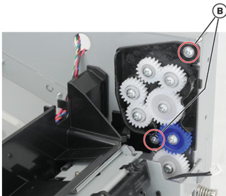
**7** Remove the redrive gear assembly.
