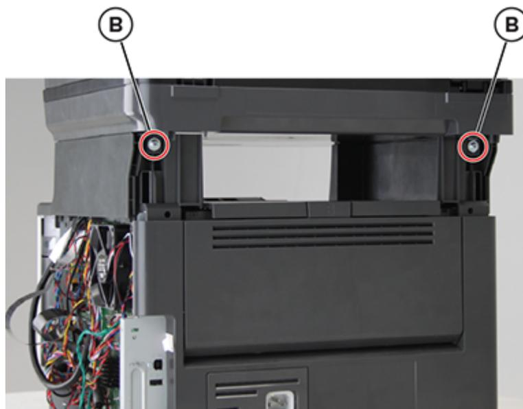
**6** Remove the flatbed scanner assembly.
