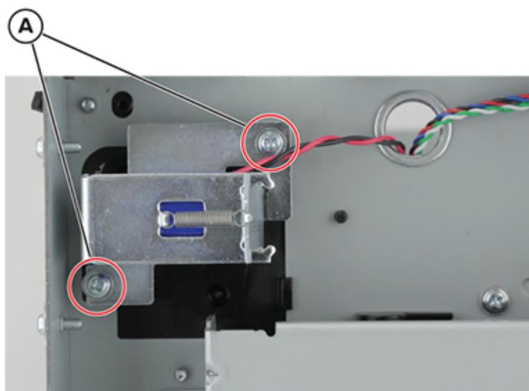
**5** Remove the fuser. See [“Fuser removal” on page 288](#).
