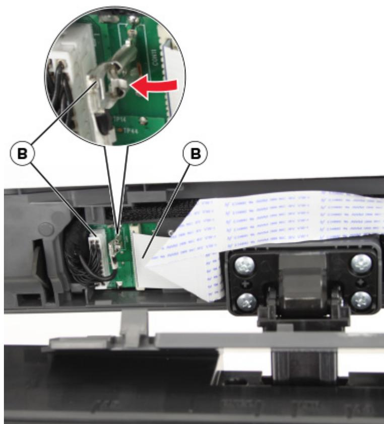
**4** Release the cables off the assembly, and then remove the ADF.
