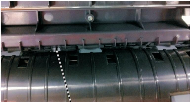
A photograph of the paper feed sensor assembly, showing several rollers and a sensor component. A white arrow labeled 'F' points to the sensor. <p data-bbox="938 1795 961 1822">F</p>                        |
