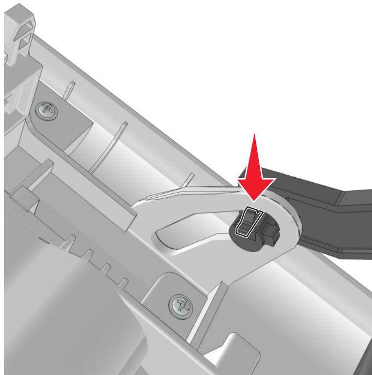
**3** Remove the 4 screws (A), and then remove the main drive gearbox.
