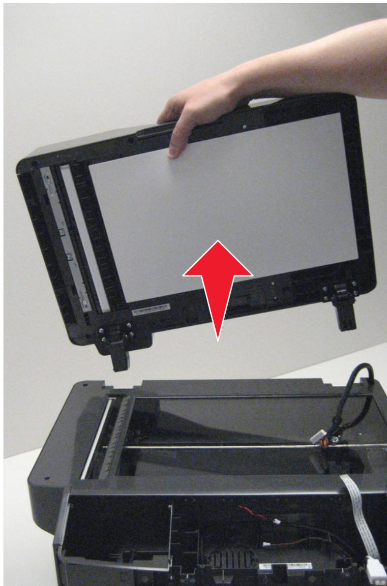
**Installation note:** After the new ADF is installed, perform scanner manual registration, see [“Scanner manual registration” on page 261](#) and scanner calibration, see [“Scanner calibration” on page 237](#).
