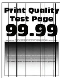
**Note:** This check applies only to printer models with a hot roll fuser.
