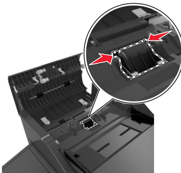
**3** Pull away the separator roll and remove.
