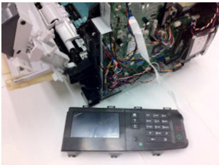
After installing the LSU, perform the mechanical and electronic LSU adjustments with the printer in this configuration. When the LSU is properly adjusted, re-install the control panel assembly to the scanner, and then re-install the scanner assembly to the MFP.
