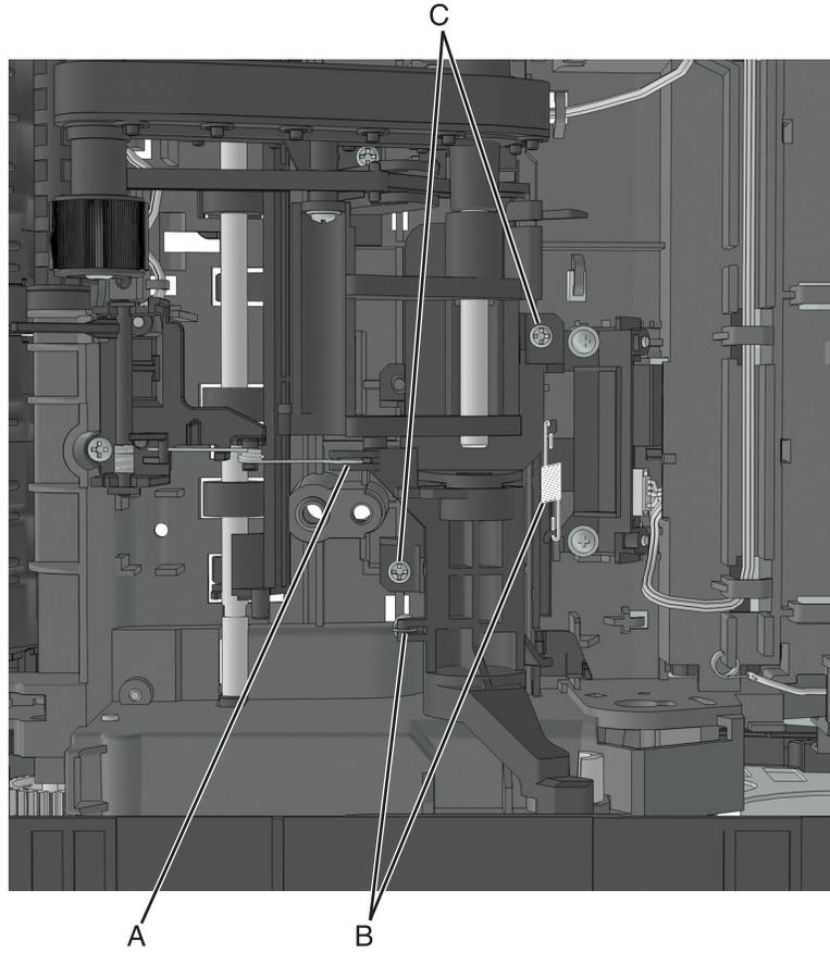
Below are the cam release and bracket.
