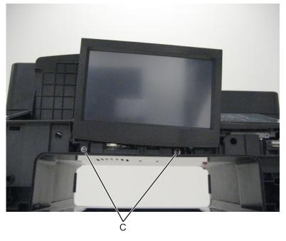
7 Gently flex the wireless chamber wall to the left to release and lift the control panel assembly upward to remove it from the scanner assembly.
