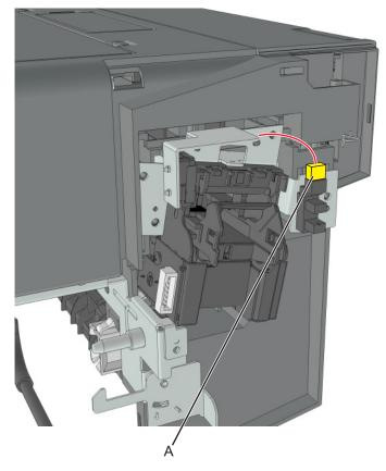
**3** Release the latches, and pull the sensor off the frame.
