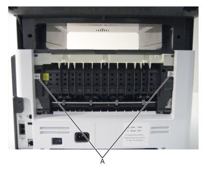
**3** Lift the upper portion of the machine to release the cover, and then remove the cover.
