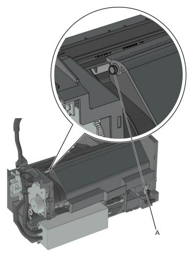
**4** Using a flat-blade screwdriver, release the latches, then remove the input cover.
