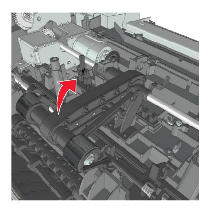
**3** The sensor flag must align with the media present sensor (A).
