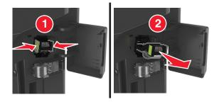
**3** Lift the staple guard, and then remove any jammed or loose staples.
