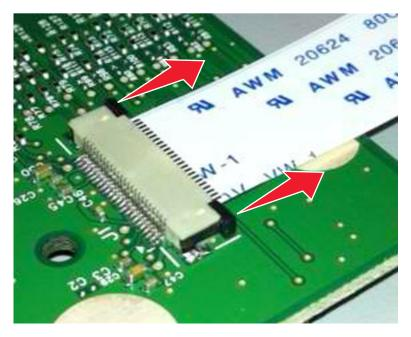
**2** Slide the cable out of the connector.
