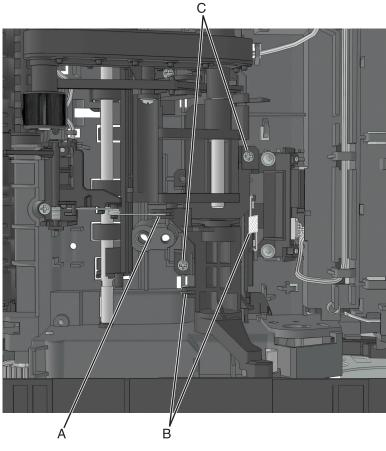
Below are the cam release and bracket.
