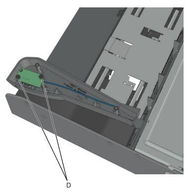
**11** Route the sensor cable off the stapler, then remove the sensor.**Note:** Pay attention to the original routing of the cables.
