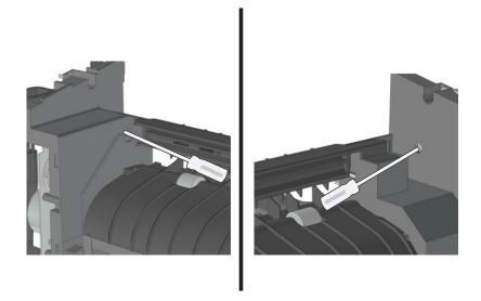
**5** Squeeze the latches to release, and dislodge the interface cable from its slot.
