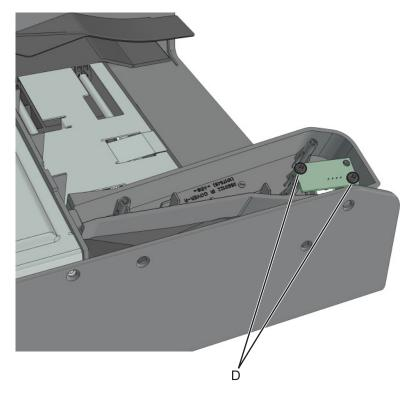
11 Route the sensor cable off the stapler, then remove the sensor.Note: Pay attention to the original routing of the cables.
