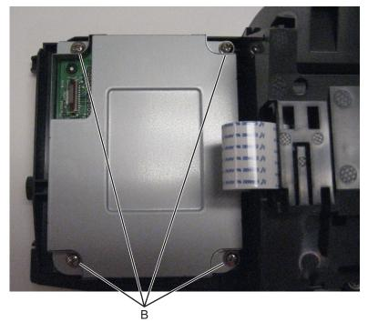
6 Disconnect the UICC video cable from the UICC card.
