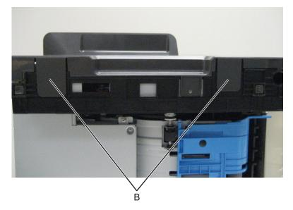
**4** Pull the cover forward, and remove it from the printer.
