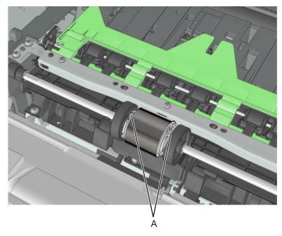
**3** Pull the MPF pick roller outward to remove.
