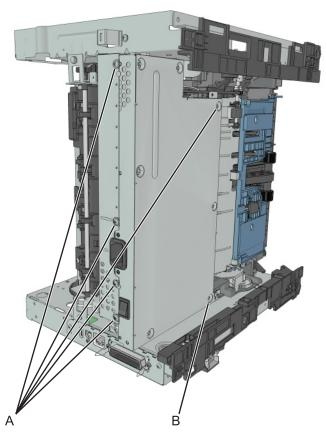
6 Remove the power supply, and then disconnect the cable from the power supply.
