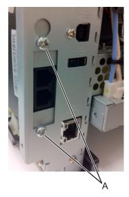
**5** Lift the modem to release, and then remove.
