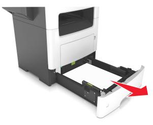
2 Firmly grasp the jammed paper on each side, and then gently pull it out.Note: Make sure all paper fragments are removed.
