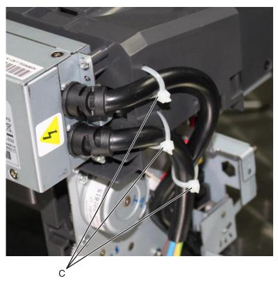
10 Route the cable off the stapler, and remove the power supply unit.Note: Pay attention to the original position of the cable.
