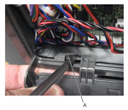
**3** Slide the access door to release the hinges, then remove it from the right cover.
