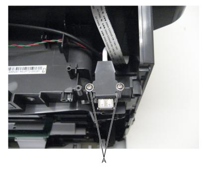
**2** Remove the USB cable bracket.
