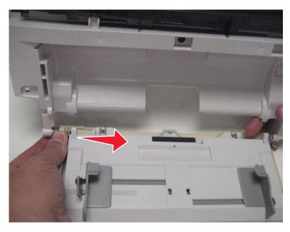
**Installation note:** Insert the straight end of the spring into the hole on the front access cover before sliding the MPF tray onto the left pivot of the front access cover.
