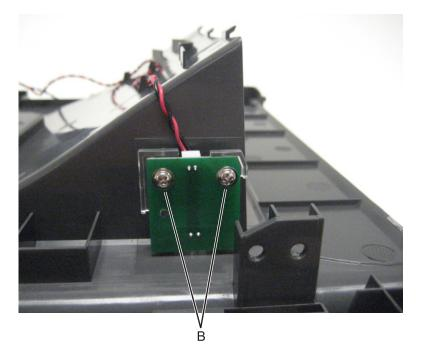
**5** Disconnect the cable (J1RED1) from the sensor.
