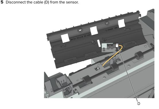
6 Release the latches, and then remove the sensor.
