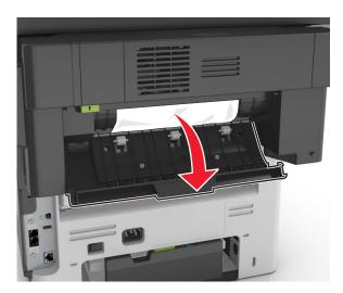
2 Firmly grasp the jammed paper on each side, and then gently pull it out.Note: Make sure all paper fragments are removed.
