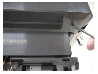
**3** Remove the scanner assembly from the MFP.
