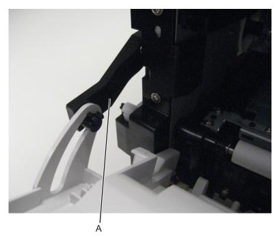
**3** Rotate the front access cover to a position that aligns the gap on the cover with the right hinge.
