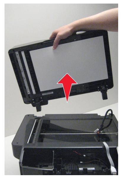
**Installation note:** After the new ADF is installed, perform scanner manual registration, see <u>"Scanner manual registration" on page 225</u> and scanner calibration, see <u>"Scanner calibration" on page 201</u>.
