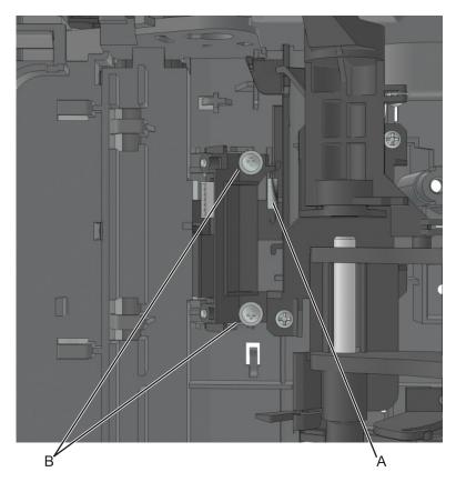
**9** Disconnect the cable from the sensor.
