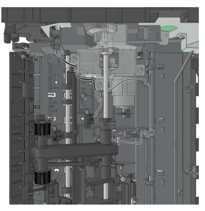
c Secure the cable near the lift plate gearbox using cable ties. Cut off any excess cable tie.
