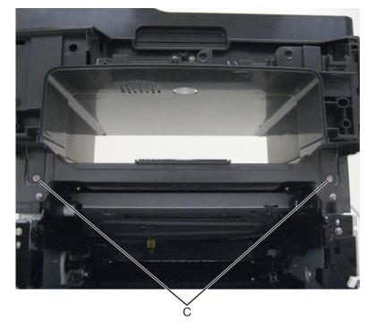
**12** Lift the complete scanner assembly away from the printer, and remove.
