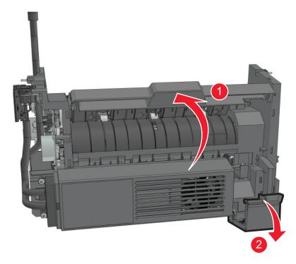
**2** Push inwards to release the hinges, then remove the staple access door.
