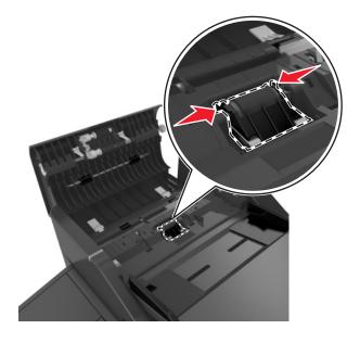
Pull away the separator roll and remove.
