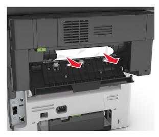
**3** Open the finisher trap door, and then remove any paper fragments from inside the trap door.
