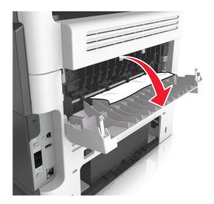
3 Firmly grasp the jammed paper on each side, and then gently pull it out.Note: Make sure all paper fragments are removed.
