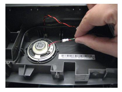
**8** Feed the speaker cable through the channel on the right side of the printer.
