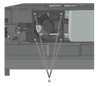
7 Route the cable off the stapler, and remove the cooling fan.Note: Pay attention to the original routing of the cable.
