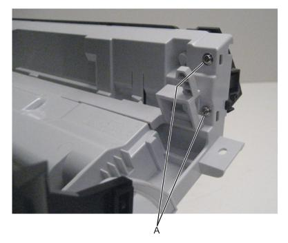
${\bf 3}~$  Lift the left side of the cover, and then remove the front bin cover.
