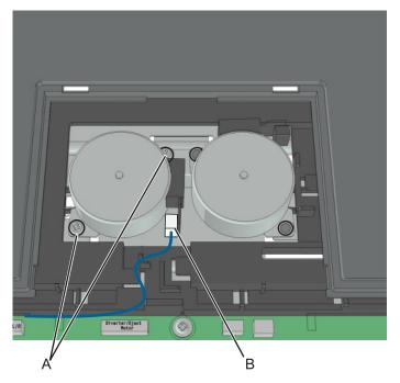
Warning—Potential Damage: Be careful not to lose the tamper belt when removing the tamper motor. Installation note: Make sure to engage the motor gears with the tamper belt.
