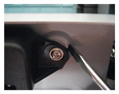
**5** Disconnect the two cables (A), and then remove the three screws (B) securing the LSU.
