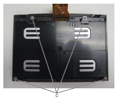
7 Remove the plastic mounting bracket, and remove the display from the LED bezel.
