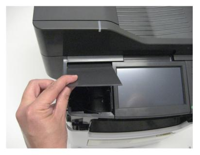
**2** Position the display at the angle shown, to access the card behind it.
