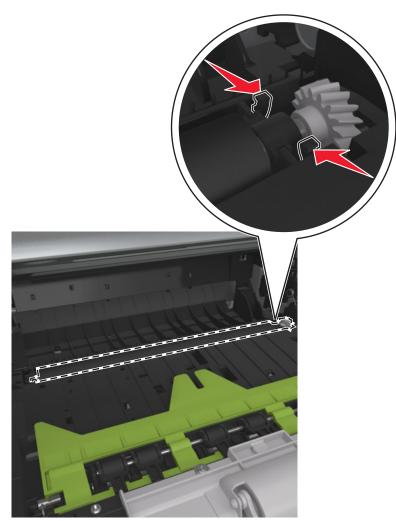
**2** Lift to remove the transfer roll.
