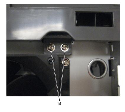
**11** Remove the two screws (C) on the front of the device securing the scanner assembly to the printer frame.
