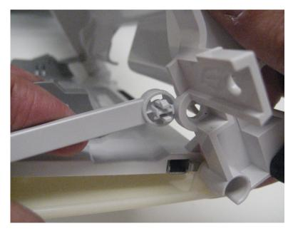
**4** Push the MPF tray to the left to release the right pivot on the front access cover.
