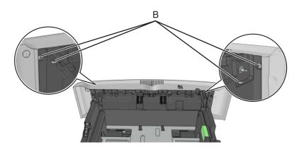
4 Push out the top part of the drawer cover, and then remove the separator roll assembly.
