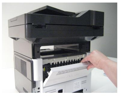
**2** Pull the exit door upward to release the hinges, and remove.
