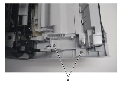
**4** Release the tabs on top of the cover, and then remove the name plate cover.
