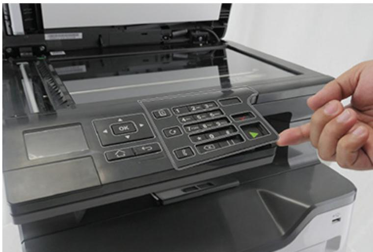
**Installation note:** When installing the cover, put in place the two latches (A) first.
