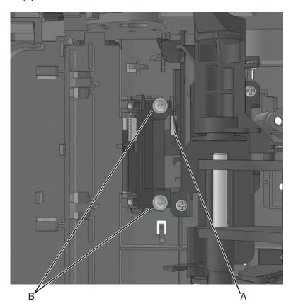
**9** Disconnect the cable from the sensor.
