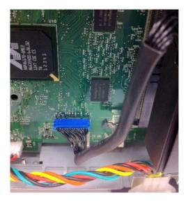
**5** Loosen the two screws (A) securing the modem to the controller board shield.
