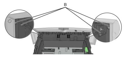
4 Push out the top part of the drawer cover, and then remove the separator roll assembly.
