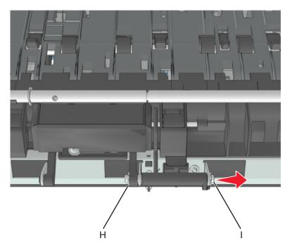
Remove the separator pad and the spring underneath.
