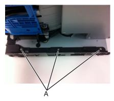
**Installation note:** Before removing the guide, note the position of the ground spring. It will need to be re-installed when the guide is re-installed.
