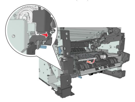
Release the front guide from the guides at each end.
