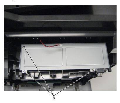
**2** Remove the UICC shield.
