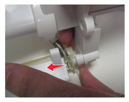
**5** Slide the tray to the right, and remove the MPF tray and spring.
