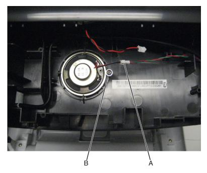
Slide the speaker off the scanner assembly.
