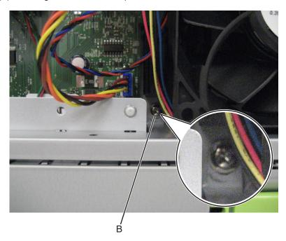
Remove the screw (C) securing the shield to the printer.
