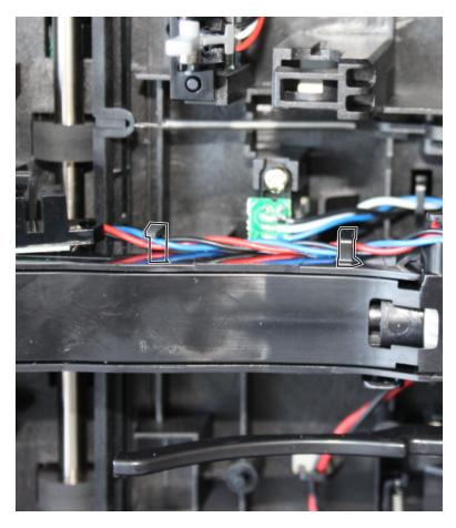
**c** Bring the cable in front of the two cable holders near the ACM shaft.
