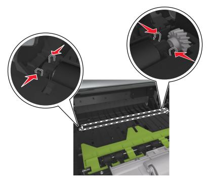
**2** Lift to remove the transfer roll.
