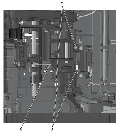
Below are the cam release and bracket.
