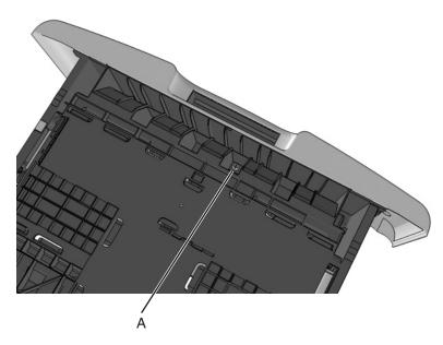
Remove the E-clip, and then remove the gear.
