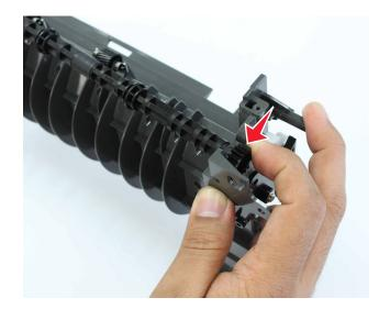
**8** If necessary, remove the bushing (B) from the redrive assembly.
