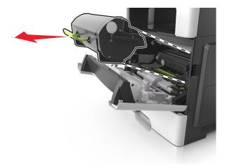
**3** Lift the green handle, and then pull the imaging unit out of the printer.
