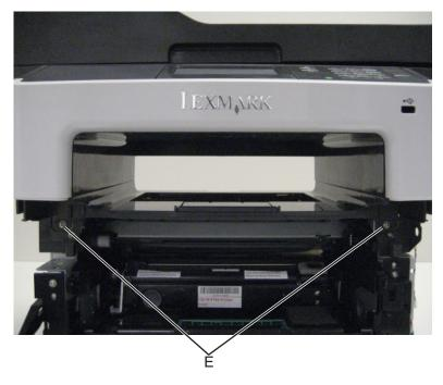
**12** Lift the scanner assembly, and remove.
