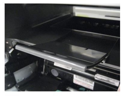
Push up on the center tab of the bin extender while pulling the extender towards the front of the printer.
