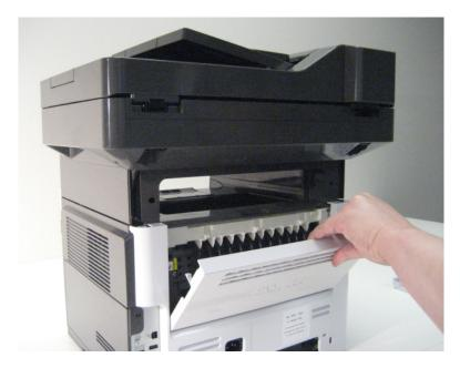
Pull the exit door upward to release the hinges, and remove.
