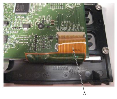
**3** Remove the five screws, and then remove the UICC.
