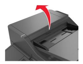
Squeeze the latches to release the separator pad.
