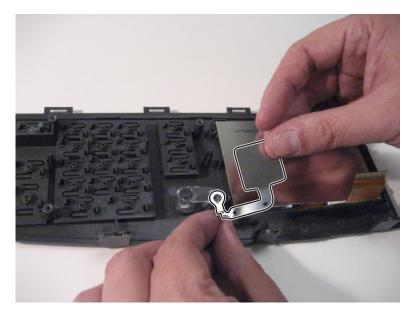
**5** Remove the light tube (B).
