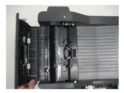
Release the cover by gently bending the ADF away from the top cover (1), and then lift the top cover (2) and remove.
