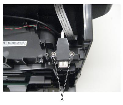
3 Remove the USB cable bracket.
