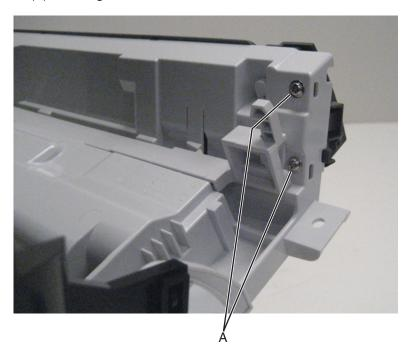
**3** Lift the left side of the cover, and then remove the front bin cover.
