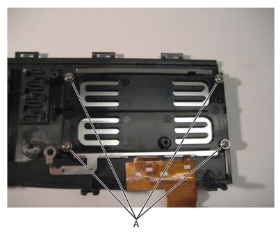
Remove the ground shield.
