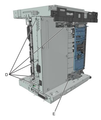
**7** Remove the power supply, and then disconnect the cable from the power supply.
