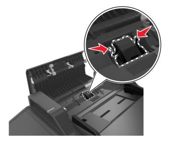
Pull away the separator pad and remove.
