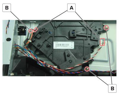
• For the Polygon LSU, disconnect the cable (A), remove the three screws (B), and then disconnect the cable JLSU1 from the controller board.
