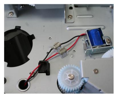
**d** Route the cable using the new path, and secure it with a cable tie (C).
