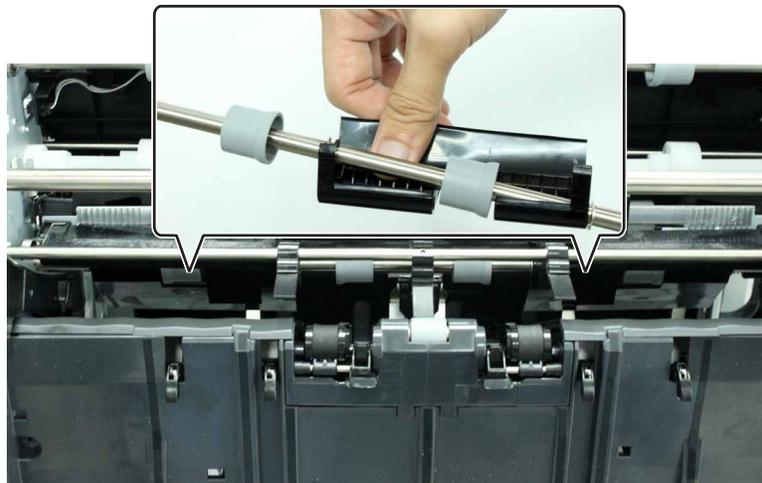
**Installation note:** Position the tabs of both bails over the metal frame.
