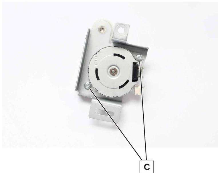
**Installation note:** Rotate the bracket counterclockwise to tighten the belt before installing all the screws.
