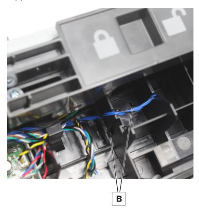
Disconnect the cable (C), and then remove the sensor.
