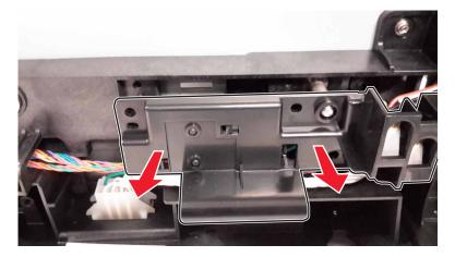
Disconnect the sensor cable (B).
