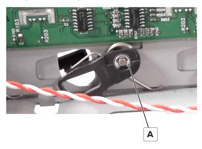
**5** Pull the bell crank (B) and spring (C) off the mounting pin.
