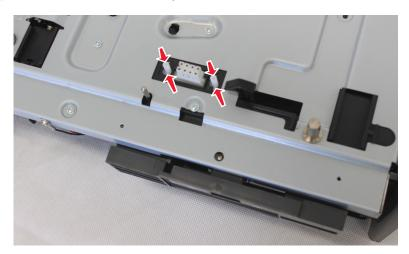
Squeeze, and then push the latches into the tray base to release the cable.
