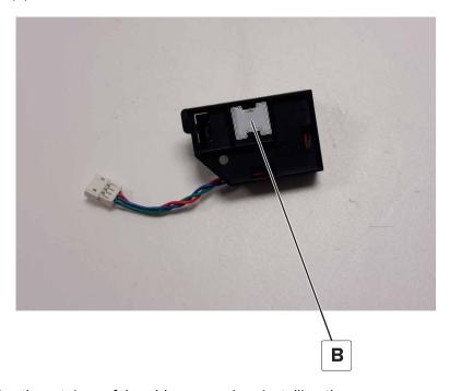
**Installation note:** Use the retainer of the old sensor when installing the new sensor.
