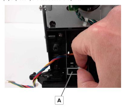
Disconnect the sensor cable (A), and then remove the sensor.
