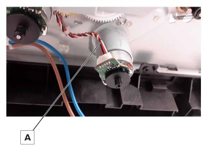
**3** Remove the two screws (B), and then remove the motor.
