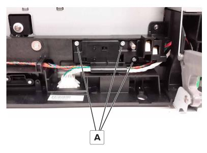
Pull the mounting assembly away from the printer.
