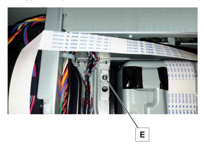
**Installation note:** When installing the printhead, replace the screws but do not tighten them right away. After installing the screws, turn the printhead clockwise until it stops before tightening the screws fully. After performing these steps, you may need to align the printhead if there is skew. You will also need to perform (TBD).
