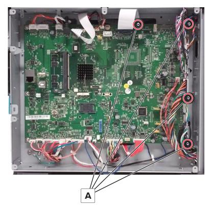
Remove the five screws (A), and then remove the controller board.
