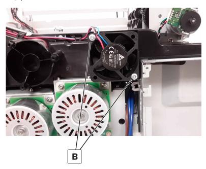
**6** Route the fuser fan cable out of the retainers (C), and then remove the fan.
