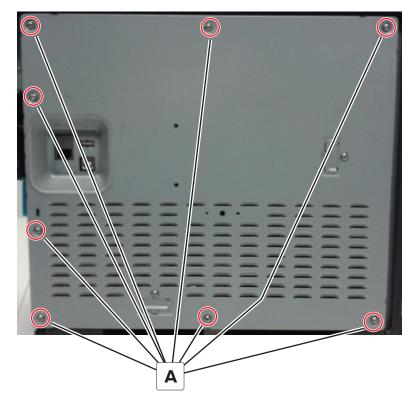
2 Remove the controller board shield.
