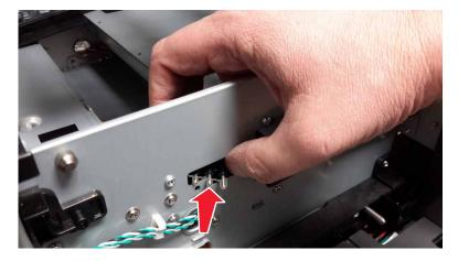
**6** Remove the cable from the retainer clips, and then remove the cartridge contacts.
