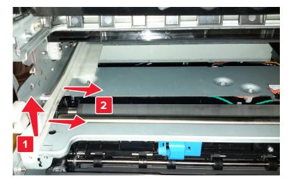
**9** Gently twist the rail to release the two tabs (D) from the frame, and then remove it.
