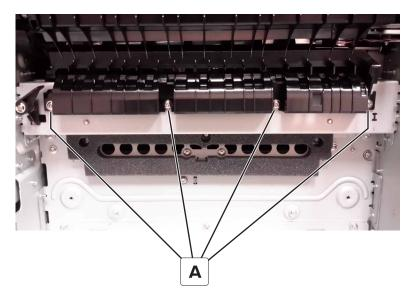
**3** Hold the redrive deflector up, and then remove the redrive guide.
