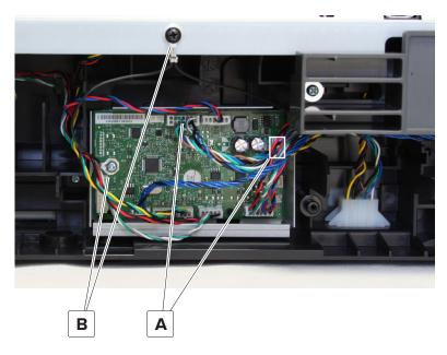
Squeeze, and then push the latches into the tray base to release the cable.
