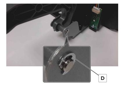
**7** Slide the shaft out, and then remove the TPS wiper.
