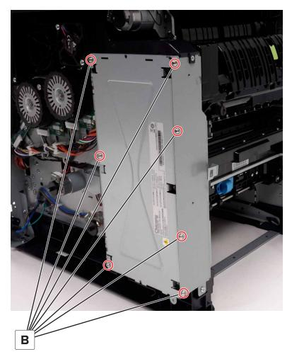
**5** Disconnect the two cables (C), and then remove the LVPS.
