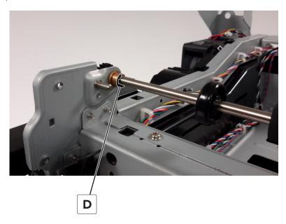
Slide the output shaft to the left, and then remove from the printer.
