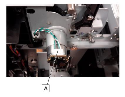
Remove the four screws (B), and then remove the motor.
