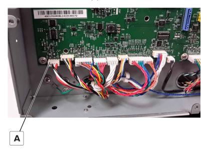
**5** Route the cable through the printer, and then remove the sensor contact assembly.
