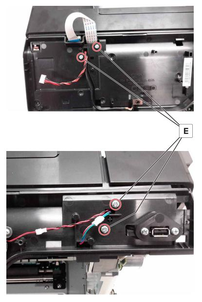
Route the control panel cables, speaker cable, and redrive sensor cable through the tub.
