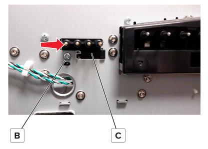
**5** Push the cartridge contacts assembly into the printer.
