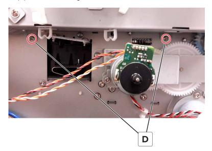
**6** Remove the two screws (E) from the top-left and top-right corners of the EP drive, and then remove the gear box.
