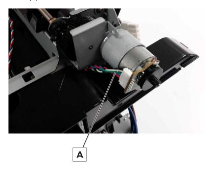
Remove the three screws (B), and then remove the motor.
