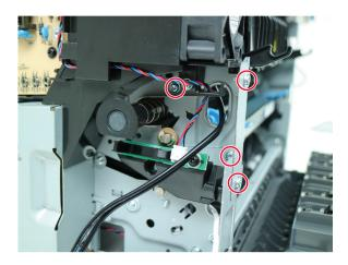
Release the bracket, and then move it out of the way.
