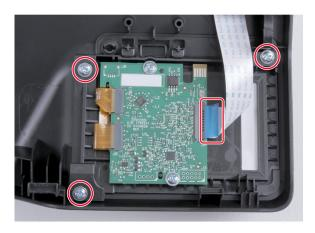
**6** Remove the control panel.
