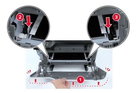
Release, and then move the door hinge out of the way.
