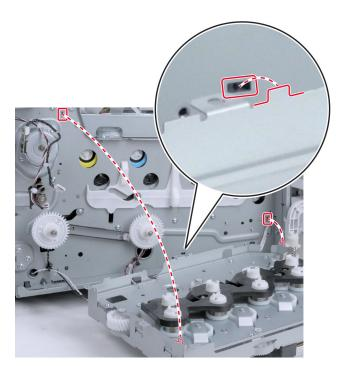
• Thread the cables to their slots. Be careful not to disconnect the switch cable from the printhead.
