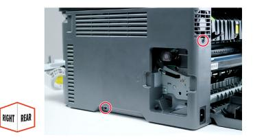
Position the printer as shown, and then release the rear latches.
