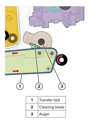
When the toner image on the transfer belt is transferred to the page, the transfer belt rotates and gets cleaned by the cleaning blade. The cleaning occurs for every page that is printed.
