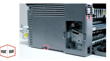
**2** Slightly move the cover to remove the screw behind it.
