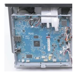
Release the antenna card from its bracket, and then release it from the controller board frame.
