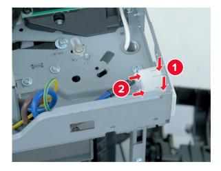
Using a prying tool, release the connector from the frame.
