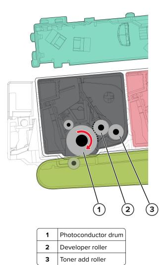
When the laser exposes the photoconductor drum in the print cartridge, the HVPS sends charge to the developer roller. For each color, the print cartridge engages the photoconductor drum so it is in contact with the developer roller. Because of the charge difference, the toner is attracted to areas of the photoconductor drum surface exposed by the laser.
