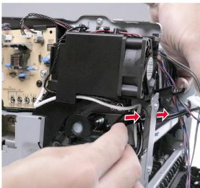
Loosen the two screws until the fuser is released.
