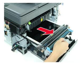
**Installation warning:** To avoid print quality issues, do not touch or scratch the transfer belt and transfer roller surface.
