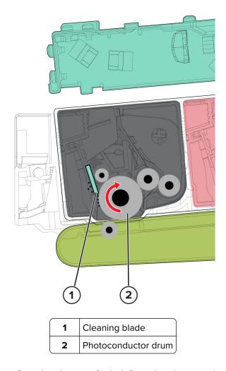
After each plane of color is transferred to the transfer belt from the photoconductor drums, a cleaning blade scrapes the remaining toner from the surface of each photoconductor drum.
