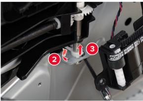
**5** Slightly pull the feeder, lower the pick roller, and then release the sensor bracket.
