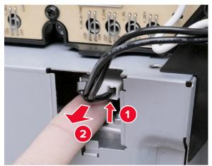
Thread the cable through the hole.
