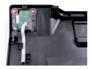
6 Remove the control panel.
