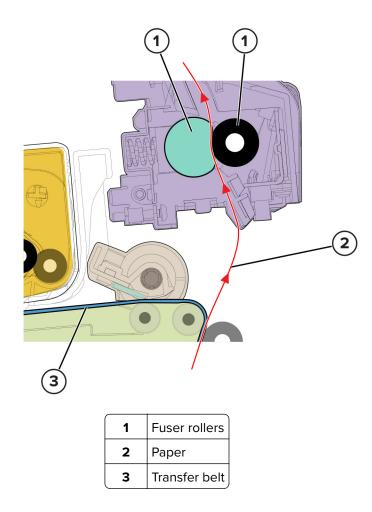
With the help of the transfer roller, the paper with the image moves into the fuser area.
