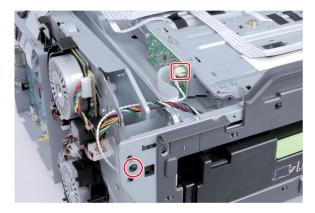
6 Remove the switch bracket.
