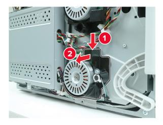
Disconnect the cable, and then remove the three screws.
