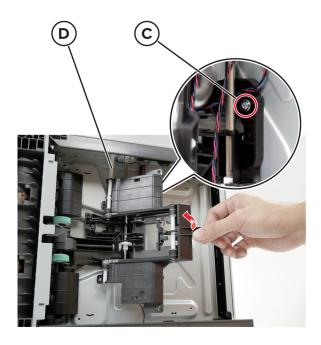
**4** Release the retainer, and then release the bottom end of the pick roller shaft.
