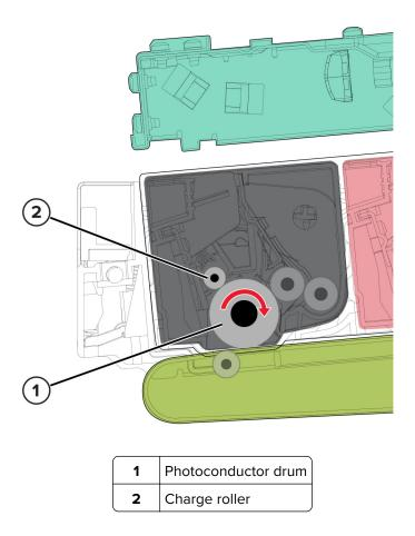
During the charge step, voltage is sent from the HVPS to the charge roller on each of the four photoconductor drums. In this printer, the charge roller is part of the print cartridge.
