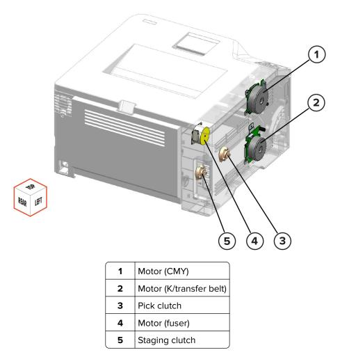
When a print job is sent to the printer, the printhead motor initiates and the fuser starts to heat. After the printhead motor reaches speed, the CMY and K motors begin turning to start the EP process. For more information, see **EP process**" on page 448.
