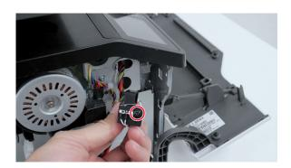
Slightly push the door as shown, and then press the latches to lock.
