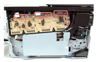
Cut the cable tie, and then remove the four screws.
