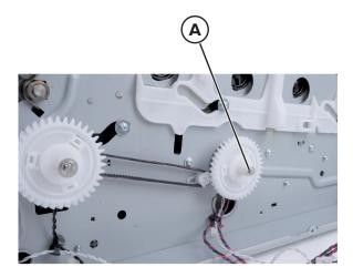
**8** Disconnect the cable, and then remove the clutch.
