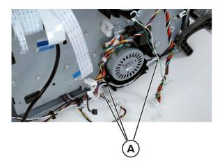
Remove the screw, and then remove the speaker.
