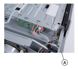
Release the cables from the printhead.
