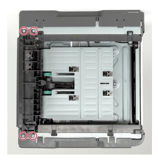
**2** Disconnect the cable, and then remove the screw.
