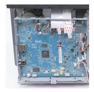
Disconnect the cables, and then release the spring (A).
