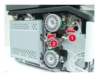
**3** Disconnect the cable, and then remove the three screws.
