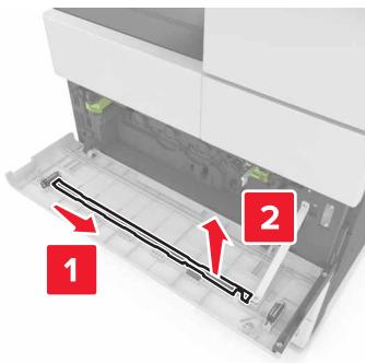
6 Insert the wiper into the hole until it stops, and then slide it out. Repeat three times.
