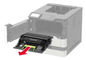
**4** Remove the used transfer roller.
