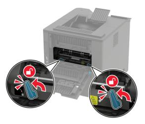
Remove the used hot roll fuser.
