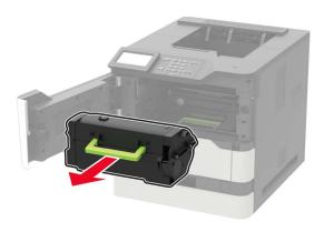
Remove the used imaging unit.
