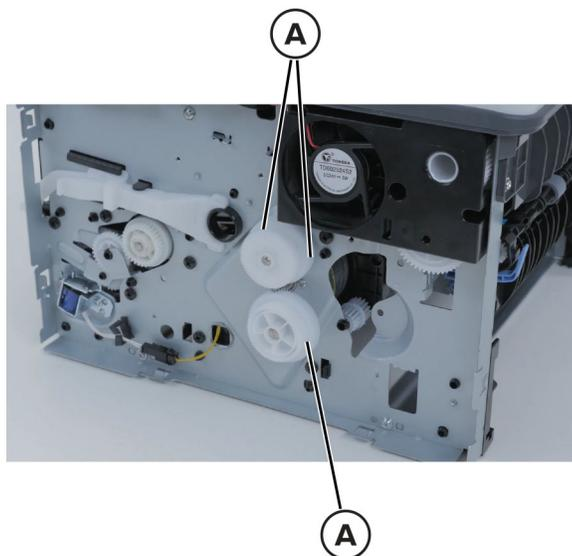
**Installation note:** Pay attention on how the gears are installed on the main drive and on the printer. Some gears may have a coupler within them. For more information, see the *Main drive removal* video.
