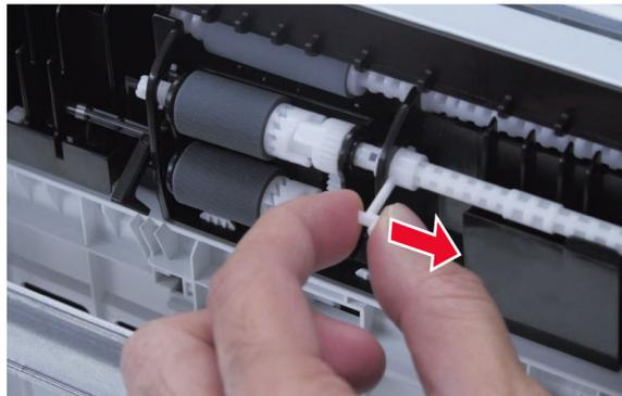
**Note:** Perform the same procedure to remove the left pick roller retainer.
