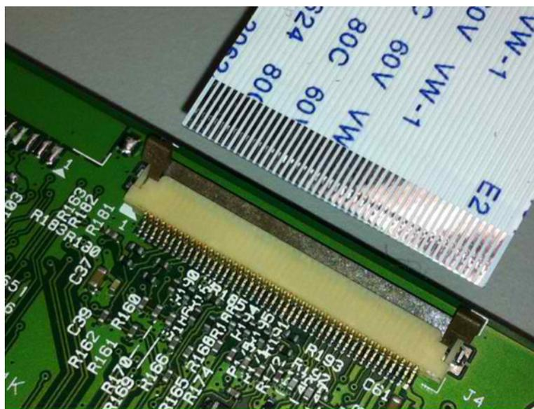
2 Rotate the locking actuator to the locked position.
