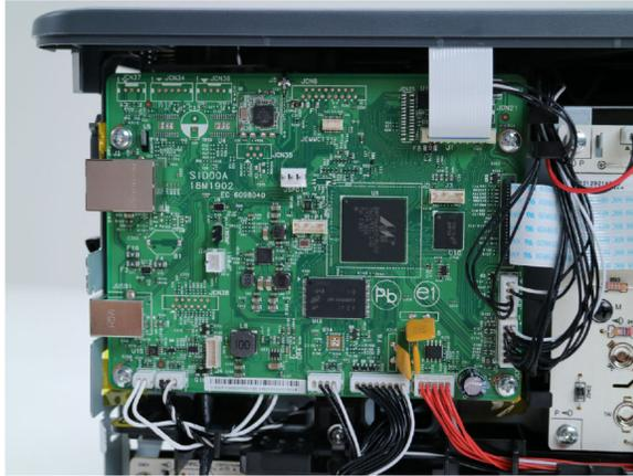
7 Remove the controller board.
