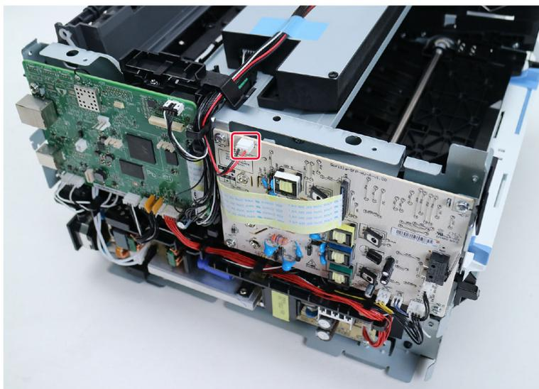
9 Remove the fan, and then remove the gear.
