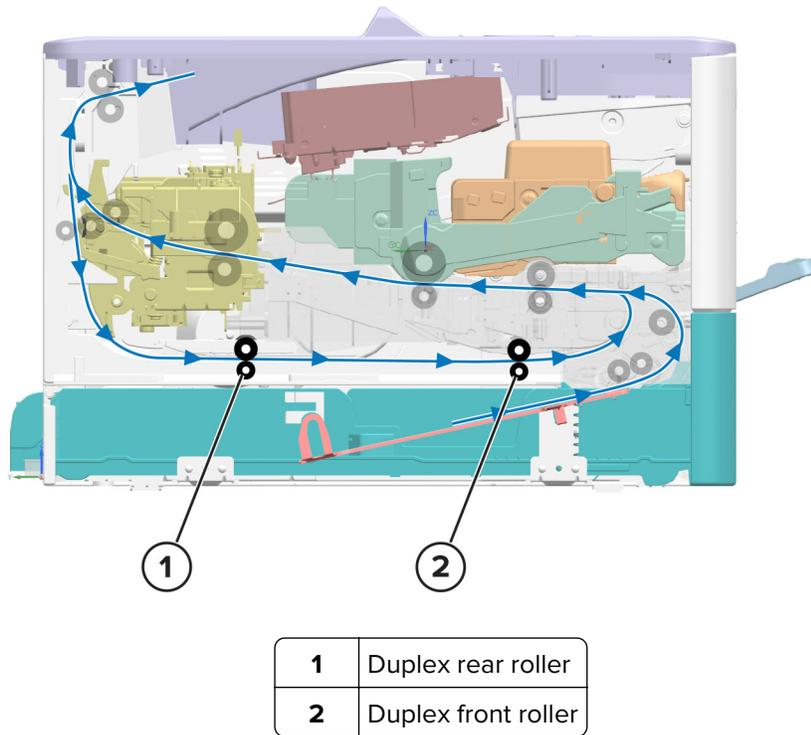
After the first side is printed, the paper stops at the output bin while still in the exit roller. The paper is fed back into the duplex paper path to have the opposite page printed.
