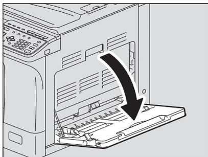
**3 Pull the paper holding lever out, and then load the envelope face down on the bypass tray.**
