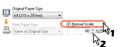
The scale can be set from 25% to 400% in units of 1%.
