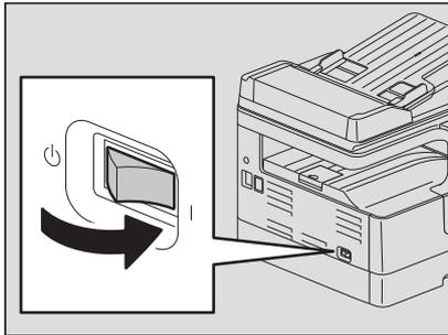
Starts warming up, which takes approx. 20 seconds. When the warm-up has finished, the equipment is ready.
