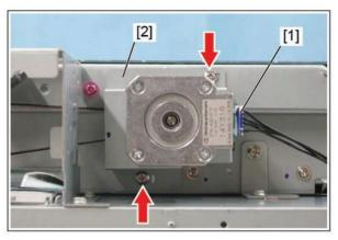
(3) Remove 2 screws and take off the scan motor [1].
