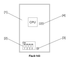
(5) Set the bits 1, 2, 3 and 4 of the DIP switch [2] as shown in the table below.
