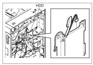
(4) Remove 4 screws and then remove 2 brackets and the ground wire from the HDD.
