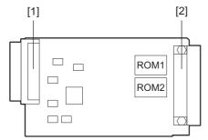
Fig.11-25 Jig board: PWA-DWNLD-350-JIG1 (16MB)
