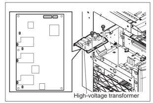
(5) Remove 5 screws and then take off the bracket from the High-voltage transformer.
