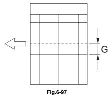
If the center line of the copy image is shifted to the rear side of the equipment, enter a value
