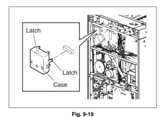
(3) Release 2 latches and take off the SRAM board for SYS board from the case.
