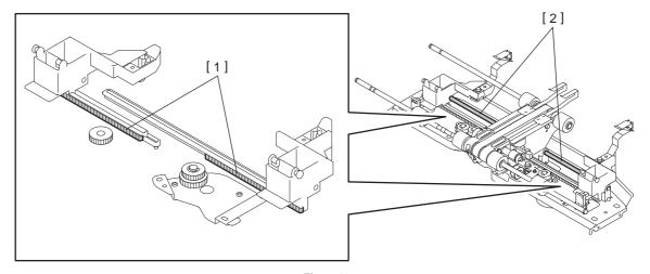
\*f Movable tray drive gear Apply an adequate amount of white grease (Molykote HP-300) to the gear teeth of the movable tray drive gear [1].
