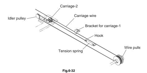
Adjustment of the carriage wire tension is not necessary since a certain tension is applied to the carriage wires by the tension springs.
