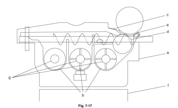
Replacement Operation Parts list Items to check Cleaning Lubrication (x 1,000 sheets) <P-I> check Whole developer unit В а Developer material R1 b 80/100/120/125/ 150/150 Front shield В R3 28-32 С d Guide roller В 29-17 Side shield В R3 28-30 е 28-31 f Developer unit lower stay В Oil seal (6 pcs.) ΑV R1 28-1 g 480/600/720/750/ 29-8 900/900 29-12
