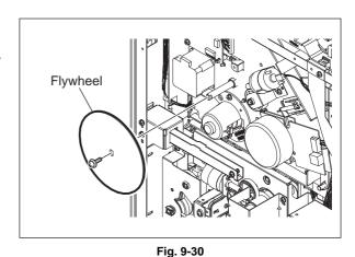
(3) Disconnect 4 connectors, remove 2 locking supports and 2 screws, and then take off the MOT board.
