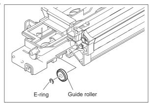
(10) Remove 1 E-ring. Remove the arm and cam.
