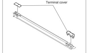
(3) Remove the terminal and spring. Then take off the needle electrode.
