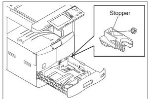
(2) Lift up the drawer paper tray. Take off the drawer tray upward by releasing it from a stopper on the front side.
