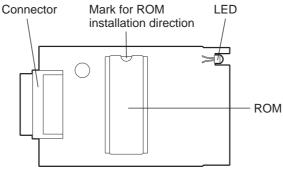
Fig.11-35 Jig board: K-PWA-DLM-320
