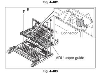
(8) Remove 2 clips, 1 bushing, 1 gear, 1 pin and the ground plate. Then take off the ADU upper transport roller.
