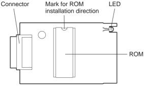
Fig.11-76 Jig board: K-PWA-DLM-320
