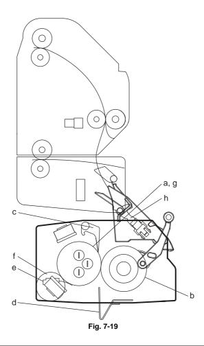
Replacement Operation Parts list Items to check Cleaning Lubrication (x 1,000 sheets) check <P-I> W2 Fuser roller A (\*1) R1 31-15 а 240/200/240/250/ 300/300 b Pressure roller A (\*1) R1 32-8 240/200/240/250/ 300/300 Separation finger for Α R1 31-22 fuser roller 240/200/240/125/ 150/150 Fuser unit entrance guide 32-11 d Α Thermistor (3 pcs.) Α R3 31-12 е 31-13 f Drive gear (tooth face W2 R3 31-11 and shaft) Fuser roller gear R3 31-18 g h Exit sensor actuator Α 32-25
