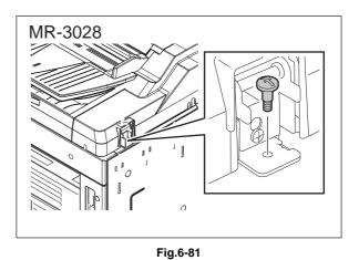
(9) Loosen the hinge screws at the front side.
