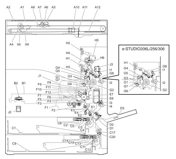
Fig. 3-1 Front side view
