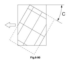
Shift the aligning plate in the direction of "+".
