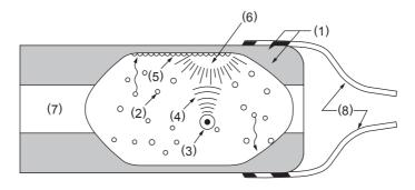
(1)Electrode (2)Electron (3)Xenon atom (4)Ultraviolet ray (5)Fluorescer
