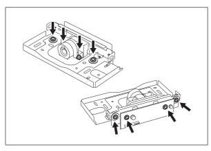
4. Handle the unit with extra care. Do not touch the adjusted area or lens. (Hold the unit as shown in the figure at right.)
