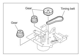
(9) Take off the gear and timing belt from the main motor drive unit rear bracket.
