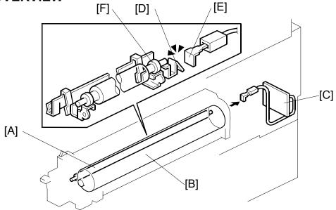
This copier uses a drum charge roller to charge the drum.
