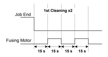
After the machine prints a job of **30 to 99 continuous pages**, the 1st Cleaning is done twice. (15 sec. after the job ends the fusing/exit motor switches on for 15 sec., pauses for 15 sec. then switches on again for 15 sec.)
