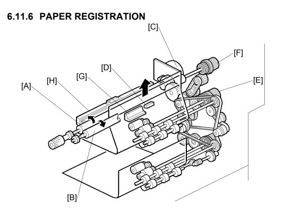
The registration drive roller [A] and idle roller [B] correct the skew of the paper to ensure that the leading edge of the paper is positioned correctly at the drum. The paper feed/development motor [C] drives the registration mechanism.
