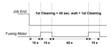
After the machine prints a job of over **100 continuous pages**, the 1st Cleaning is done, there is a pause of 45 sec. then the 1st cleaning is done again.
