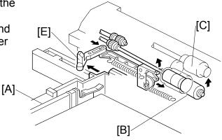
When the paper tray is set into the machine, it pushes the release lever [E]. This causes the pick-up roller [D] to go down and the separation roller [B] to move up and contact the paper feed roller.
