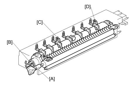
The fusing unit has two fusing lamps: the first fusing lamp (center: 650W) [A] heats the center of the fusing roller, and the second fusing lamp (ends: 650W) [B] heats both ends of the hot roller. This arrangement ensures even heat on all surfaces of the roller.
