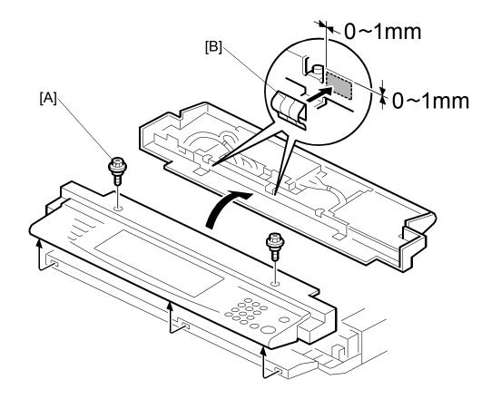
Install Anti-Static Springs on Operation Panel
