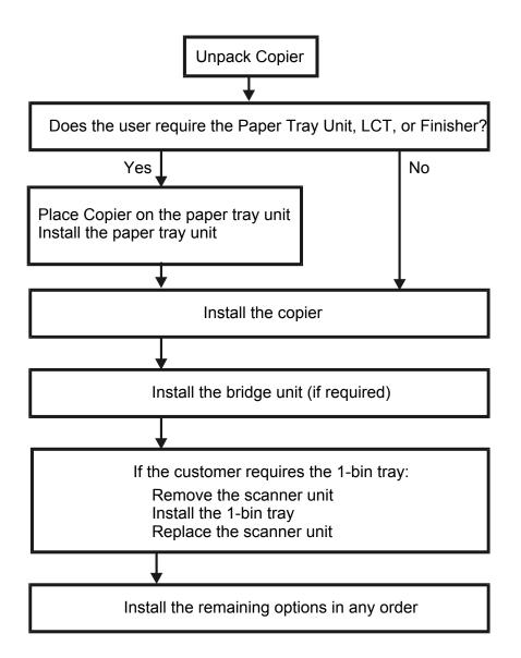
Bridge Unit: Needed for the finishers and external output tray.
