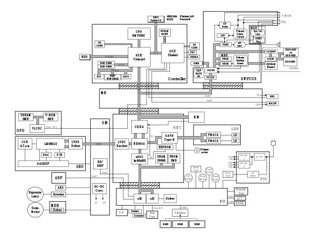
This machine uses the GW (Grand Workware) architecture, which allows the copier to be expanded as an MFP by installing simple modular components (SD cards) on the controller board. The BICU and FCU are connected to the controller via a PCI bus.
