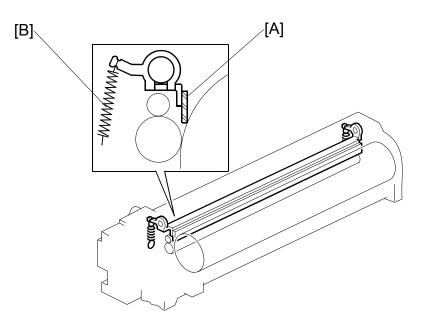
The PxP (Polyester Polymerization) toner of this machine is of much finer particle size so in addition to the stationary cleaning blade, mounted with two screws at the bottom of the PCU, an additional cleaning blade [A] has been added to increase the efficiency of drum cleaning.
