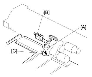
If there is paper in the paper tray, the paper end feeler [A] is raised by the paper stack, and the paper end sensor [B] is deactivates.
