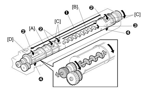
The dual mixing roller consists of the outer paddle [A] and the inner auger [B].
