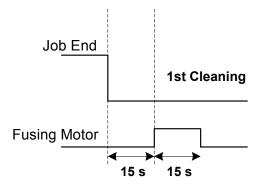
After the machine prints a total of **5 sheets** (five jobs of 1-sheet each for example, or a continues print of up to 29 pages), 15 sec. after the job ends the fusing/exit motor switches on for 15 sec. and then stops. This 15 sec. on/off cycle, called the "1st Cleaning" is done once.
