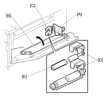
The high voltage supply board [A] applies a positive current to the transfer belt [B] through the terminal block [C], terminal plate [D], and the bias roller [E].
