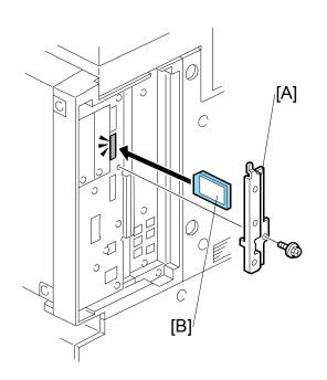
Replacement Adjustment 11. Remove the NVRAM (x2) from the controller board and replace them with the new chips.
