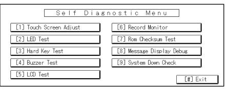
2. On the touch screen press "Touch Screen Adjust" (or press 1).
