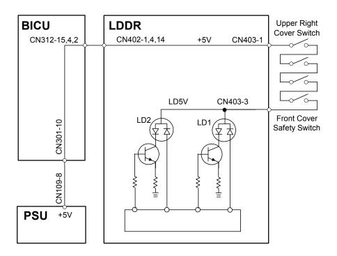
To ensure personal safety and to prevent the laser beam from inadvertently switching on during servicing, power to the laser diode is switched off when the front cover or upper right cover is opened. Four safety switches are installed in series on the LD5 V line from the power supply unit (PSU) via the BICU board.
