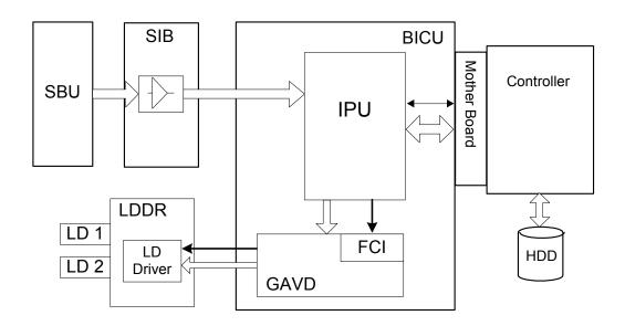
The image data from the SBU goes to the IPU (Image Processing Unit) IC on the BICU board, which carries out the following processes on the image data:
