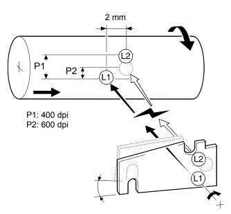
The two laser beams arrive on the drum surface about 2 mm apart in the main scan direction and about 0.06 mm apart (at 400 dpi) in the sub scan direction. The two-mm difference in the main scan direction allows the machine to detect the laser synchronization signal for each beam.
