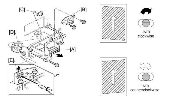
Use SP2-902-3 No. 10 (Trimming Area) to determine whether a parallelogram image appears. If the parallelogram pattern appears, perform the following procedure.
