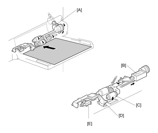
The by-pass unit is directly driven by the copier through gear [A].
