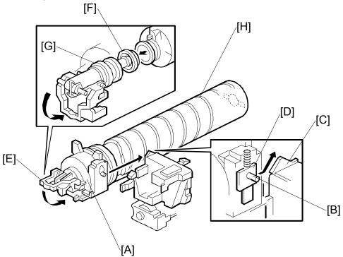
When the toner bottle is installed in the bottle holder [A], pin [B] slides up the side of the PCU [C], pulling out the toner shutter [D]. When the toner bottle holder lever [E] is returned to its original position, the cap [F] pulls away and is kept in place by the chuck [G].
