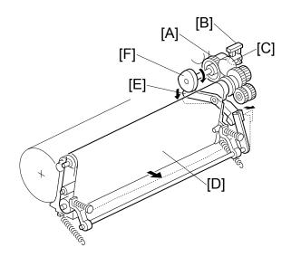
The ID sensor pattern must not be transferred to the belt. Also, the transfer belt and drum must not remain in contact for too long, to prevent contamination of the drum with oil or other foreign material from the transfer belt.
