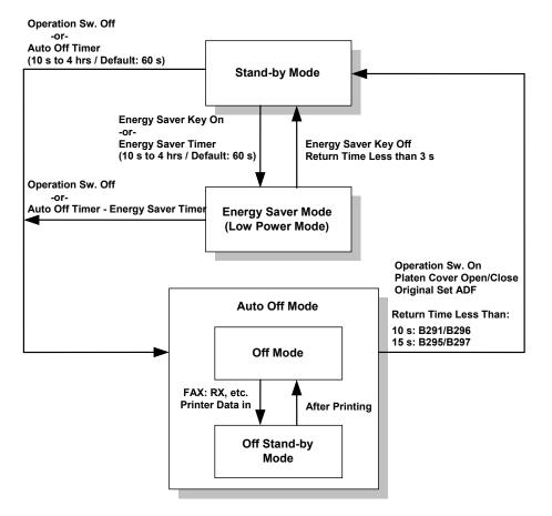
When the machine is not used, the energy saver function reduces power consumption by decreasing the fusing temperature.
