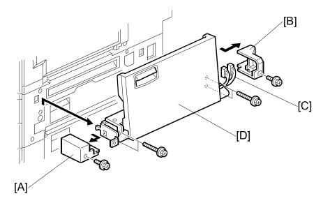
Use this procedure to remove the complete by-pass tray unit from the machine. If you wish to remove only the table, or some of the components of this unit, see 3.16.
