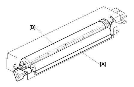
The cleaning roller [A], in constant contact with the pressure roller [B], collects toner and paper dust from the surface of the pressure roller.
