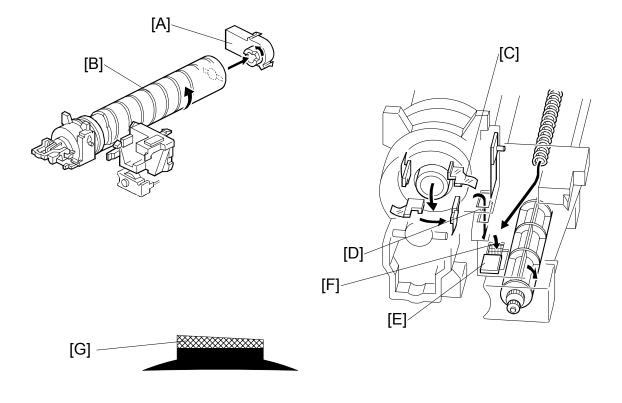
The toner supply motor [A] rotates the toner bottle [B] and the mylar blades [C]. Toner falls into the toner bottle holder, and the toner supply mylar blades [C] transfer the toner to slit [D]. Installing the PCU opens the shutter [E].
