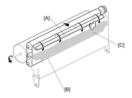
The cleaning blade [A], always in contact with the transfer belt, scrapes off toner and paper dust remaining on the transfer belt.
