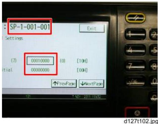
1. Use the numeric key "4" to turn bit 4 ON and be sure to press "#" button to confirm. The result should look like: **00010000** as shown above. By doing this Card Save option will appear in "List/Test Print".
