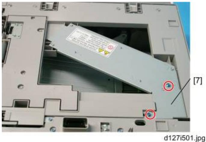
8. Attach the harness cover [7]. (
