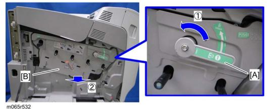
2. Turn the lock lever [A] counterclockwise, and then open the drum securing plate [B].
