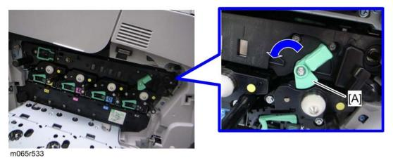
3. Turn the ITB lock lever [A] counterclockwise.
