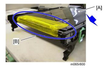
1. Lubricate a part of the surface of the image transfer belt [A] with yellow toner, and then turn the image transfer belt to the position [B] as shown above.
