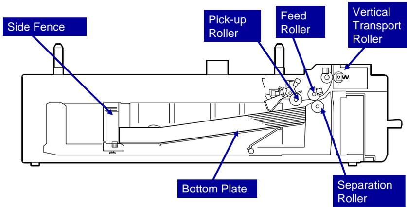
□ This tray uses a feed and reverse roller mechanism.
