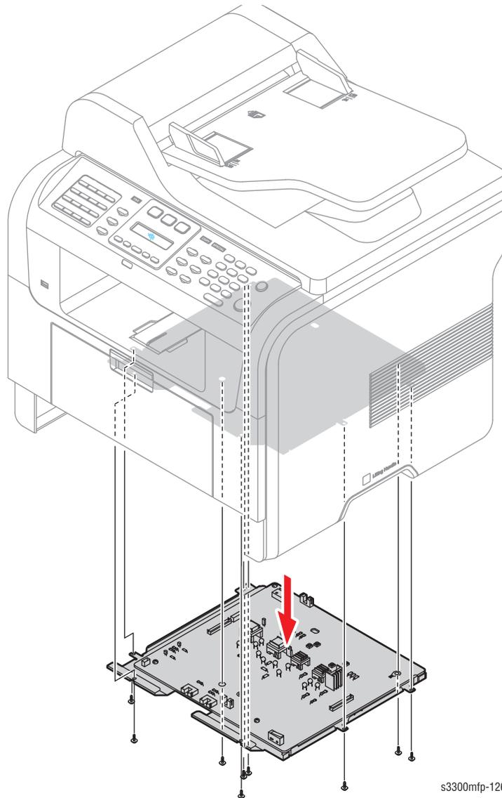
2. Unplug the connector for the Connection PBA and SMPS first. Unplug the other connections.
