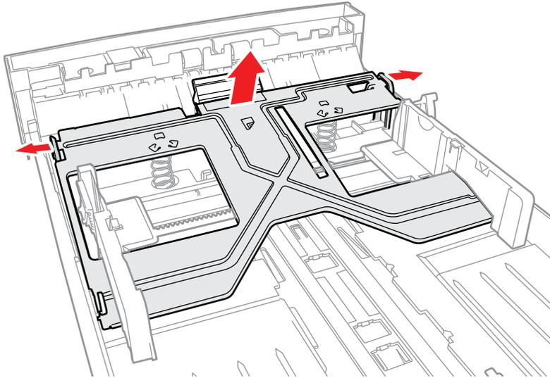
6. While holding the Tray Holder Pad, use a flat tip screw driver to pry the Holder Pad notch up from the tray.
