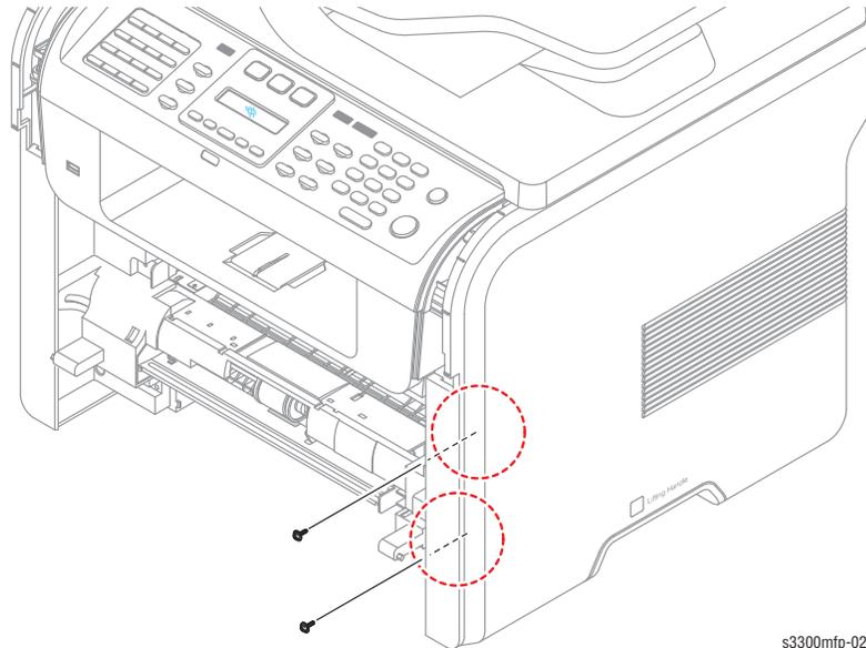
2. Apply light pressure to the bottom of the Right Side Cover and pull it to the right side in the direction of arrows, as shown below.
