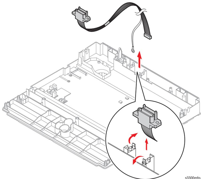
12. Unplug the connector from the Open Sensor Assembly.
