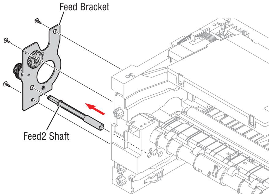
5. If necessary, release the three E-Rings securing the Gears (T2 Idle, Retard, Idle) and then remove the Gears from the Feed Bracket, as shown below.
