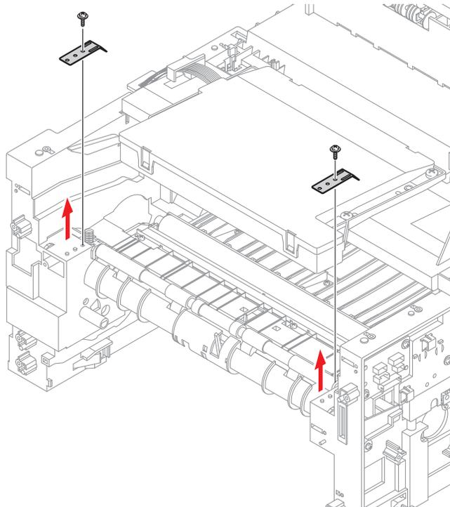
**2. Pull up the Feed Idle Shaft and the Bushings (with Spring).**
