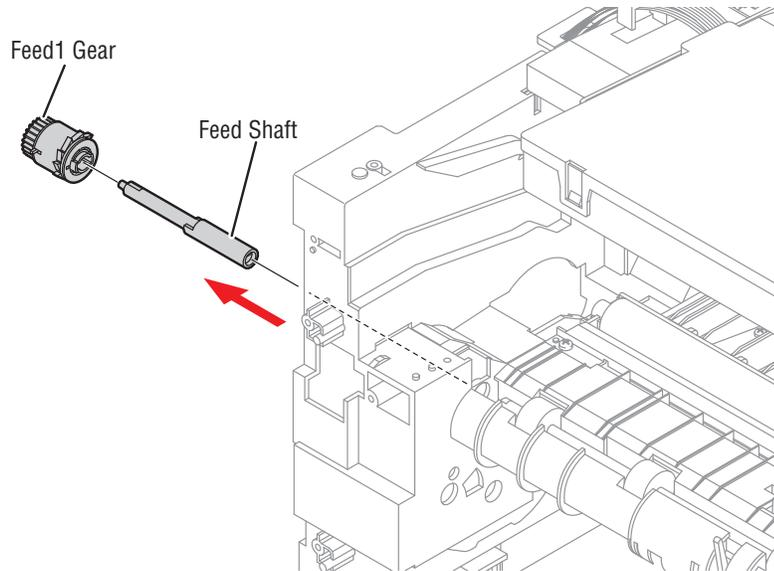
7. Pull up the Feed1 Roller from the Bushing, as shown below.
