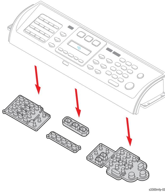
6. Remove the Lens and Keys from the Control Panel Cover.
