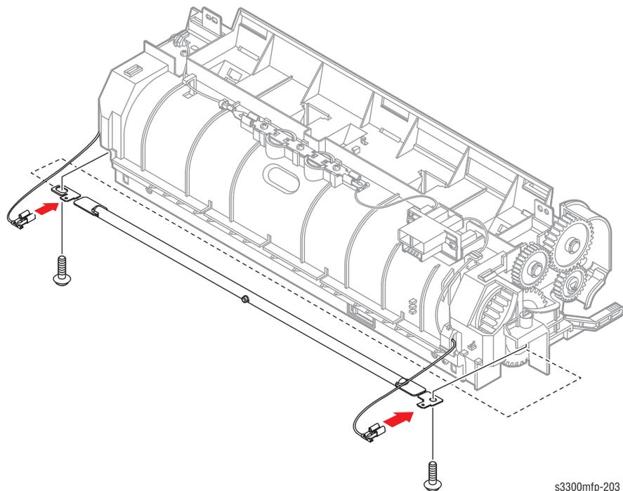
5. Remove two screws, then the Fuser Harness Connector.
