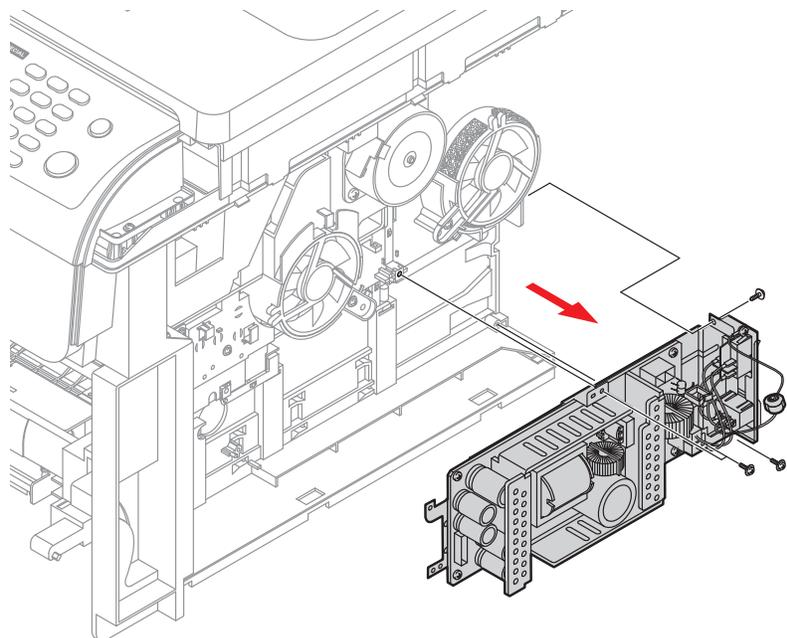
3. Unplug the connector (AC Inlet) and remove the four screws securing SMPS and remove it.
