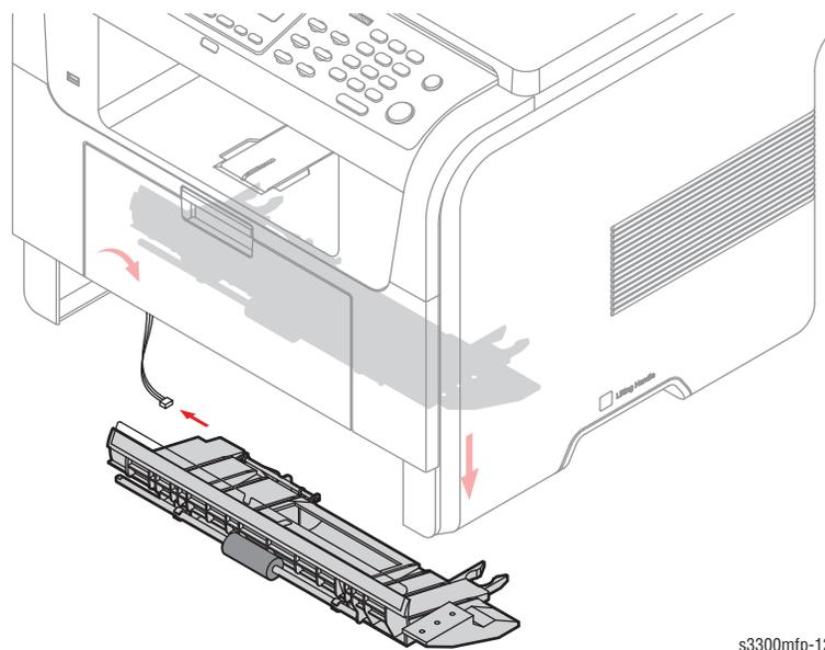
4. Pull the Feed Roller from the bushing.
