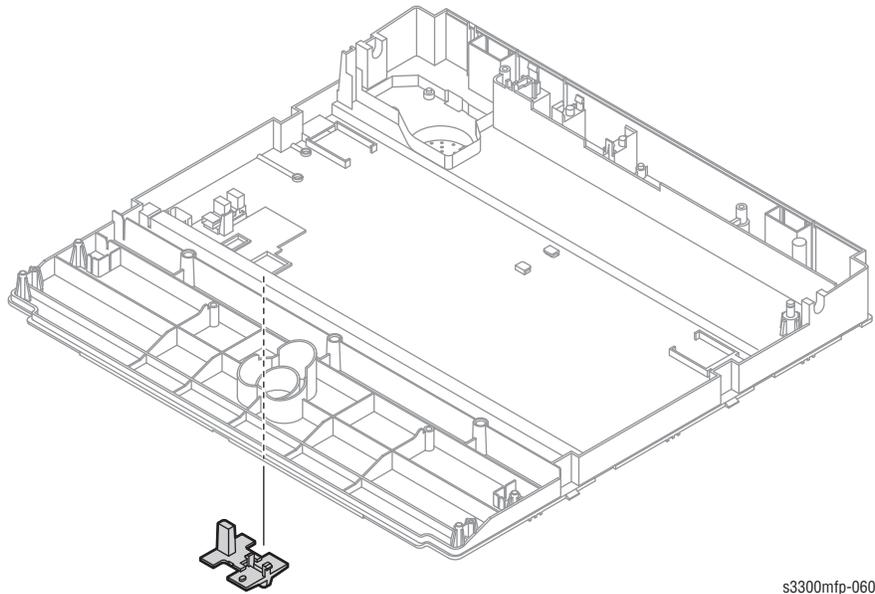
15. Unplug the Harness from the CCD Home Sensor and release the CCD Home Sensor, as shown below.
