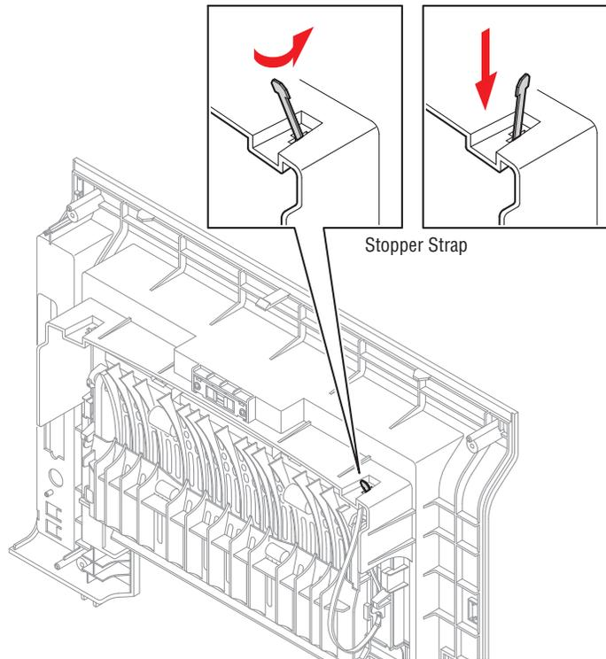
4. Unlatch the Face Up Cover from the Rear Cover and then release the Face Up Cover, as shown below.
