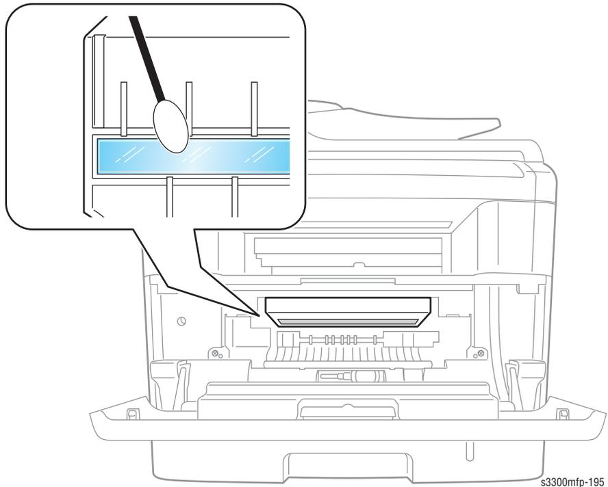
2. Check the Transfer Roller for damage.
