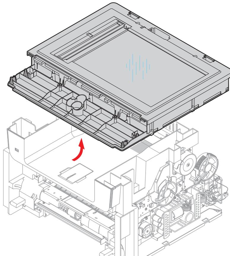
4. Remove the four screws securing the Scan Upper Cover.
