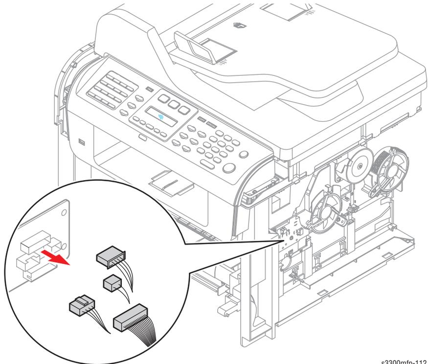
2. Remove the two screws securing the Connection PBA and remove it.
