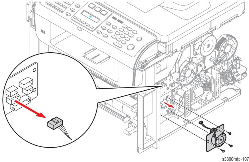
2. If necessary, remove the two screws securing the Duplex Motor and remove it.
