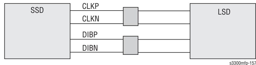
Clock from SSD to LSD has Differential structure of 180 phase difference for Noise Robustness
