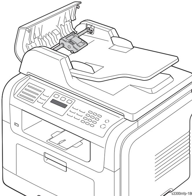
2. Lift the tab to release the bushing, and rotate it as shown below until it is straight up and the bushing is free in the slot.
