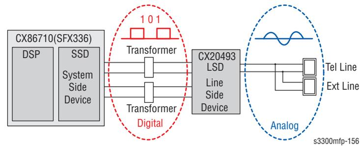
Transformer transfer Clock from SSD to LSD and Clock Frequency is 4.032 MHz.
