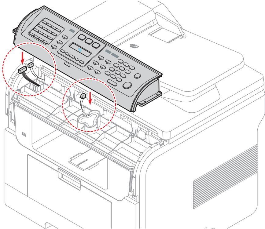
4. Remove the nine screws securing the Control Panel PBA to the Control Panel Cover.
