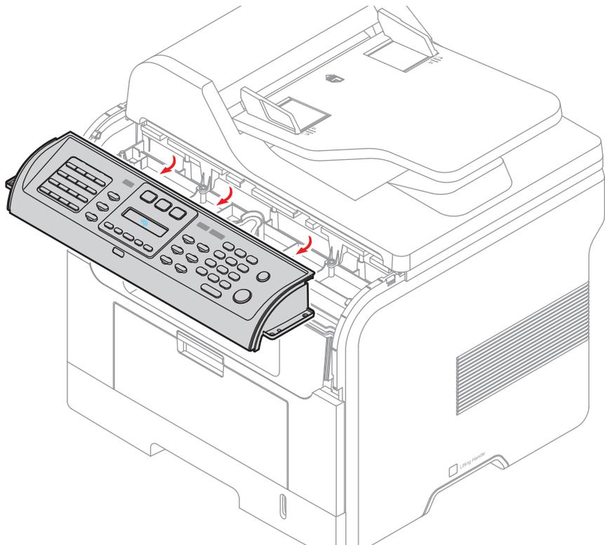
3. Unplug the three connectors from the Control Panel PBA, as shown below.
