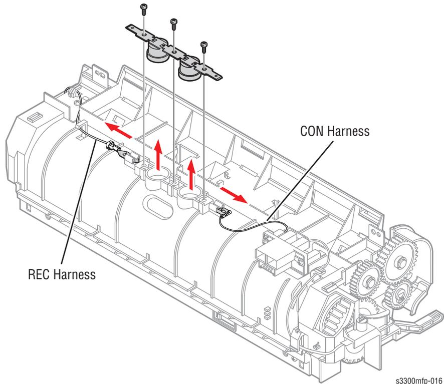
4. To remove the halogen lamp, release the REC harness and CON harness from both sides of the fuser. Remove 2 screws, then carefully slide the halogen lamp out of the fuser.
