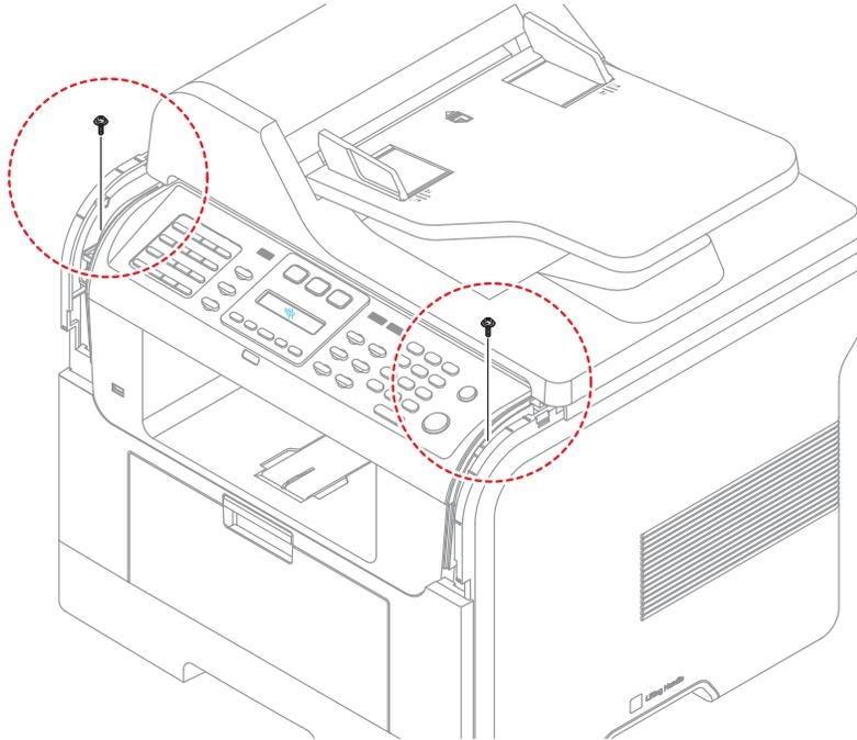
2. Apply light pressure to the front of the Control Panel and pull it in the direction of arrow, as shown below.
