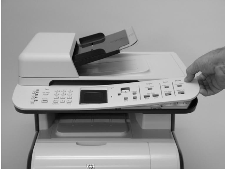
Figure 6-5 Remove the control-panel bezel
