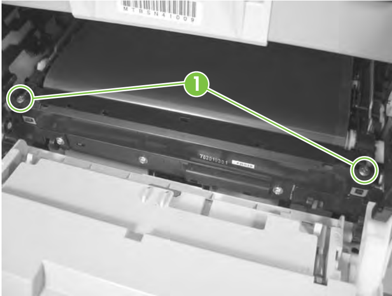
Figure 6-29 Remove the ITB (1 of 6)
