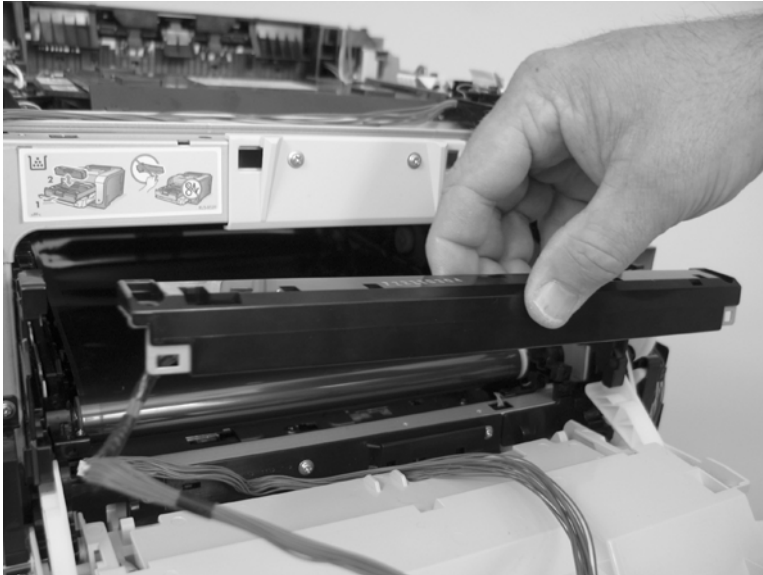
Figure 6-115 Remove the color-misregistration sensor assembly PCA (5 of 5)
