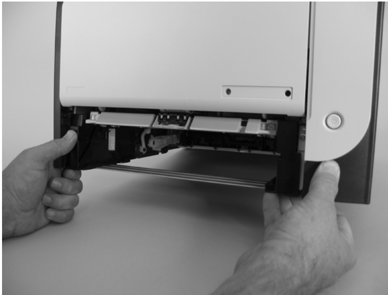
Figure 6-11 Remove the pickup roller (1 of 3)
