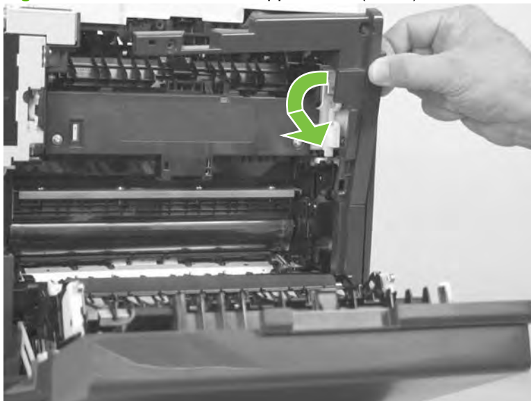
Figure 6-67 Remove the rear-upper cover (2 of 2)
