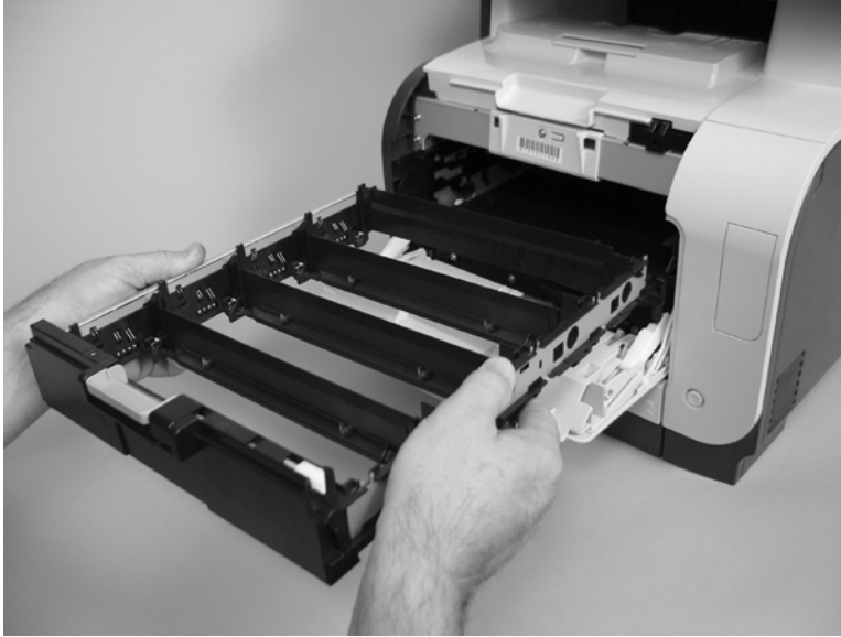
Figure 6-28 Remove the print-cartridge drawer (3 of 3)
