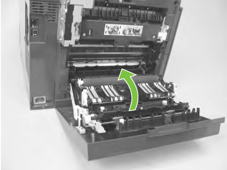
Figure 6-49 Remove the rear door (duplex product) (1 of 4)
