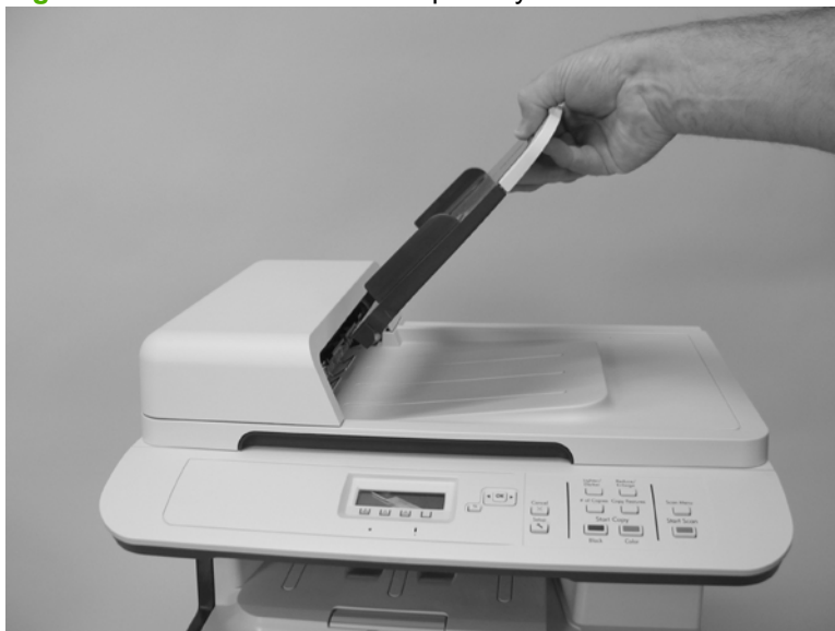
Figure 6-24 Remove the ADF input tray
