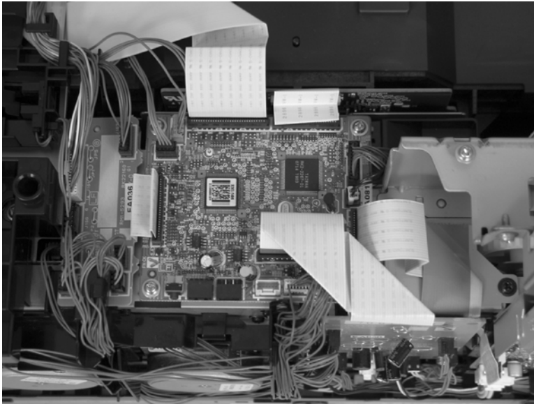
Figure 6-60 Remove the DC controller PCA (1 of 2)
