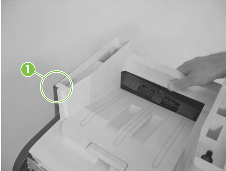
Figure 6-97 Reinstall the upper-cover assembly (1 of 3)
