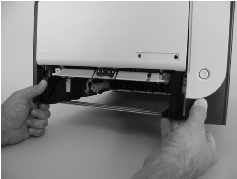
Figure 6-18 Remove the Tray 1 paper-pickup roller (2 of 3)
