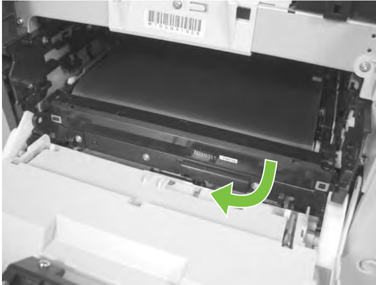
Figure 6-30 Remove the ITB (2 of 6)
