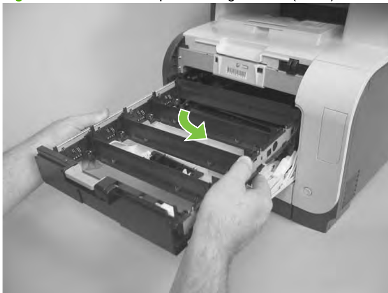
Figure 6-27 Remove the print-cartridge drawer (2 of 3)
