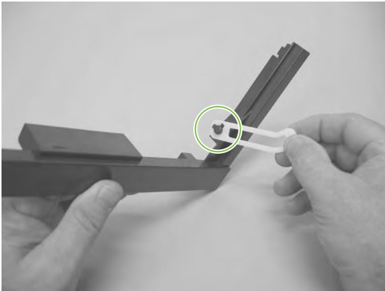
Figure 6-79 Remove the rear-lower cover and rear-door links (duplex product) (6 of 6)
