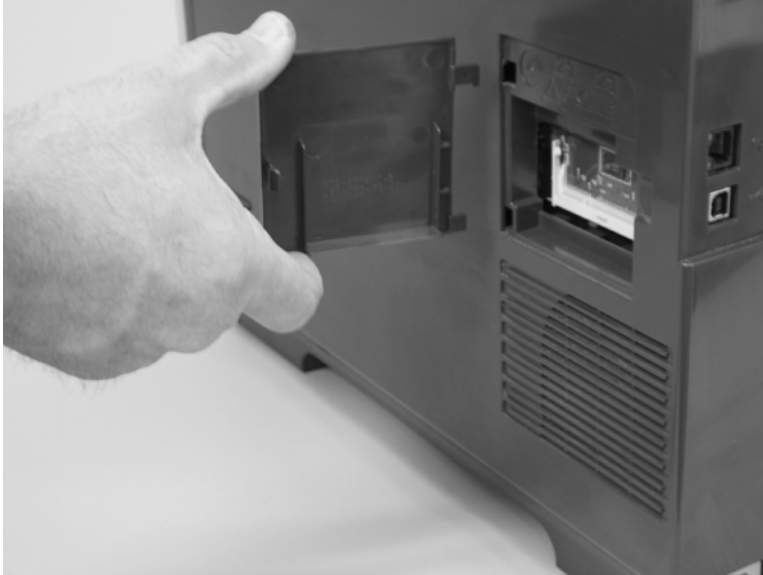
Figure 6-25 Remove the DIMM cover
