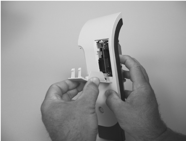
Figure 6-130 Remove the memory-card cover and PCA (6 of 7)
