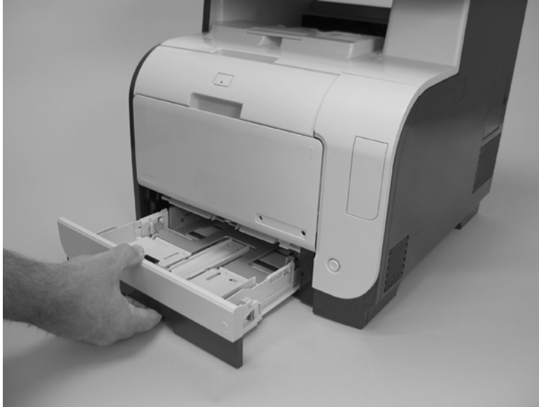
Figure 6-3 Remove the tray cassettes and optional Tray 3 assembly (1 of 2)
