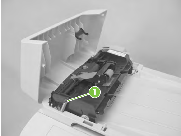
Figure 6-15 Remove the ADF pickup roller assembly (1 of 2)
