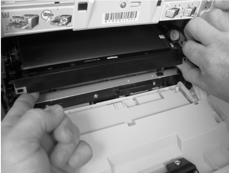
Figure 6-32 Remove the ITB (4 of 6)
