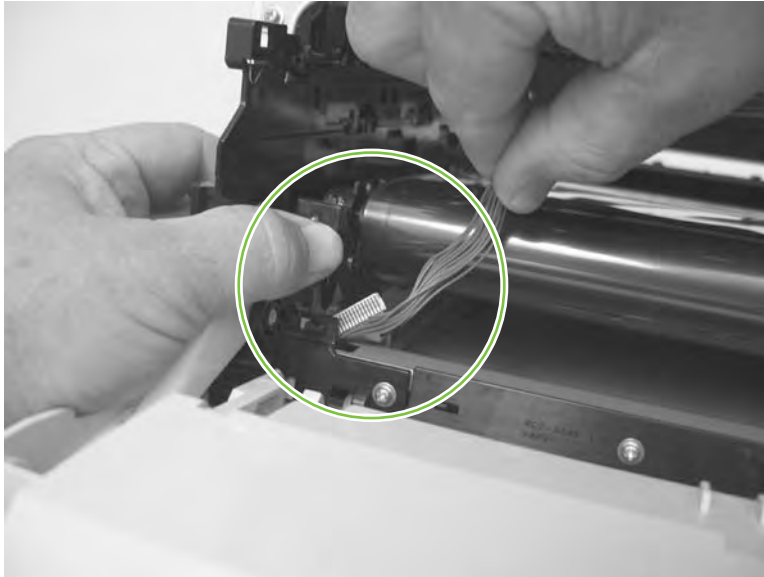
Figure 6-116 Reinstall the color-misregistration sensor assembly PCA (1 of 2)
