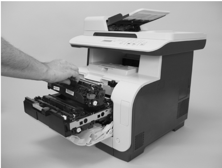
Figure 6-2 Remove the print cartridge
