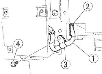
A technical diagram of a control PCB assembly. It shows a cable (1) being inserted into a connector (2) labeled J126. A cable holder (3) is positioned to hold the cable in place. A screw (4) is used to secure the cable holder. The diagram is a line drawing with numbered callouts 1, 2, 3, and 4 pointing to the respective parts. |
