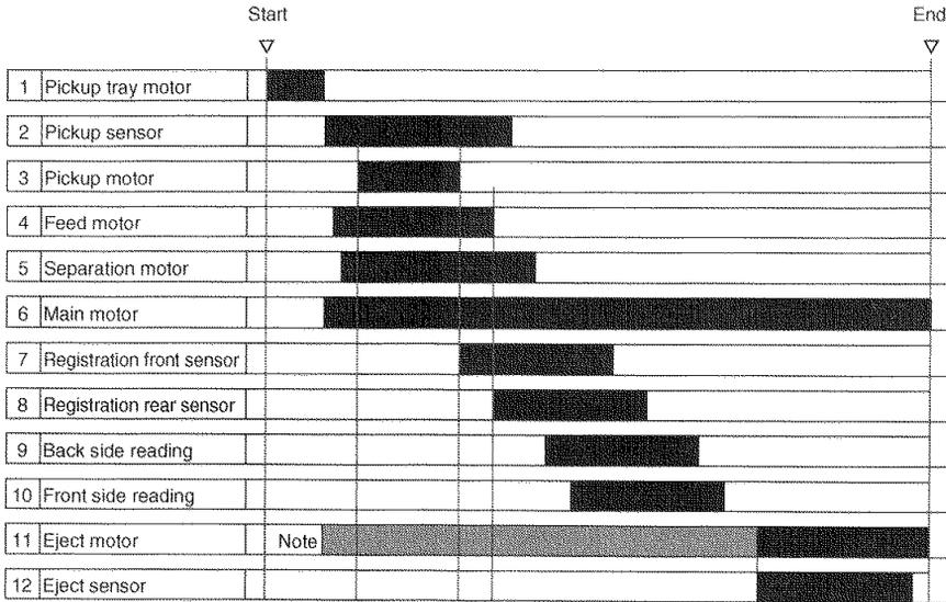
Note: The gray part of the eject motor is ON for high-speed feeding and OFF for low-speed feeding.
