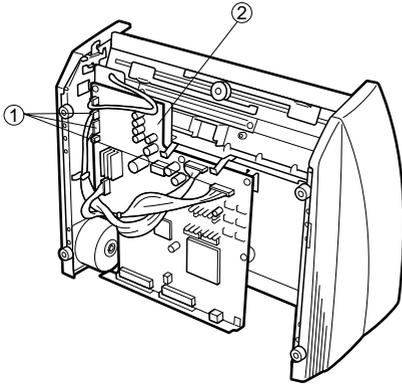
① Connectors      ② CPU PCB assembly
