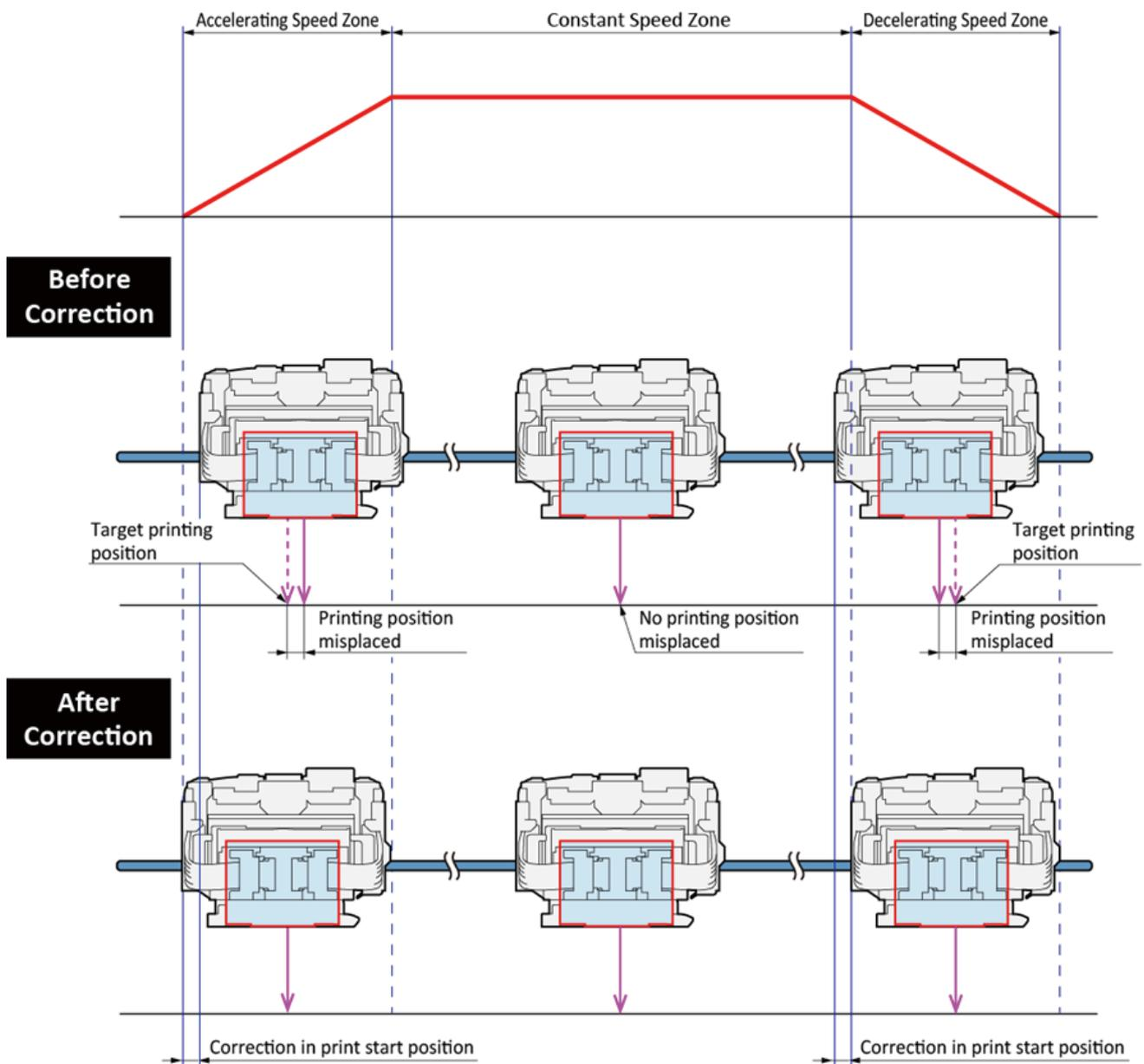
3) **Correcting misplacement of printing position caused by mechanical error:**
