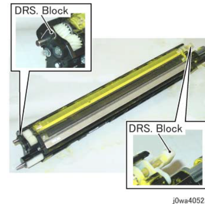
Figure 10 Make sure that no Developer or toner is stuck to the DRS Block locations
