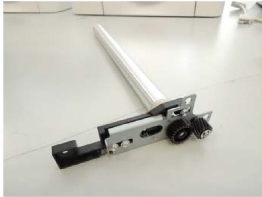
Figure 11 Rear holder and tension roll
