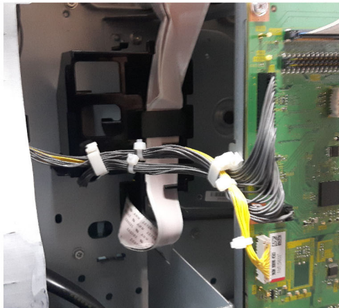
Figure 5 Wire harness removal
