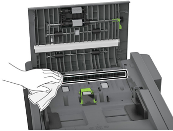
Figure 7 DADF glass in door C
