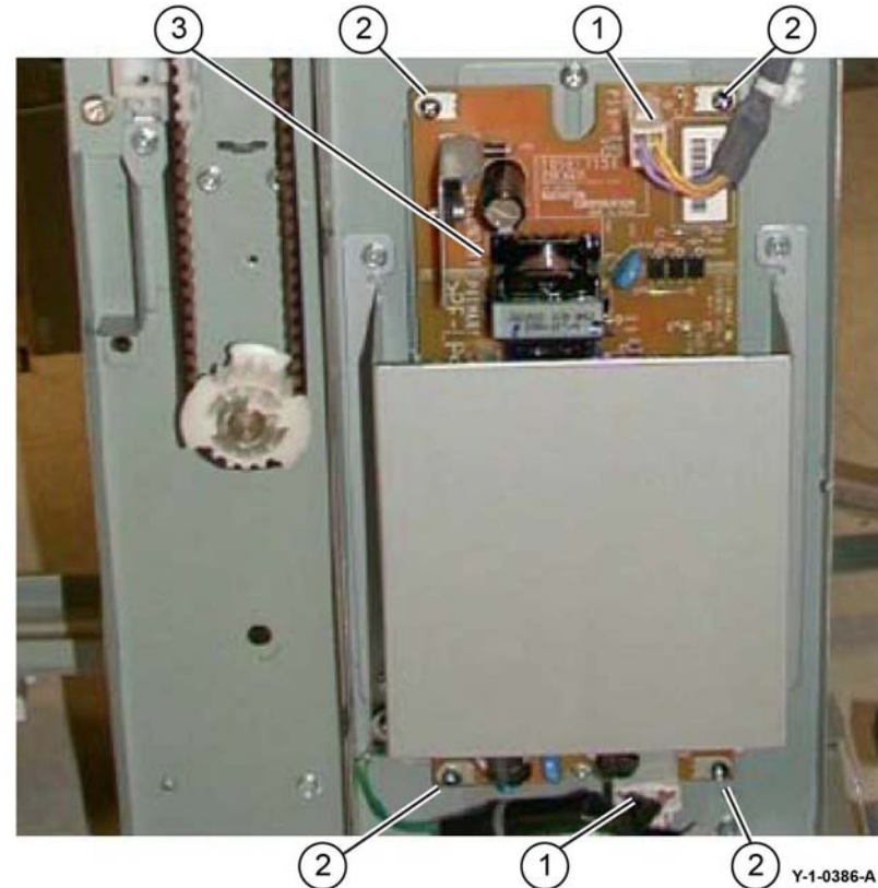
Figure 1 Finisher LVPS removal
